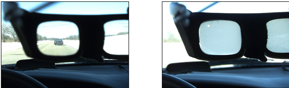
Figure 10. Open and Closed States of the Occlusion Glasses from the Driver's Perspective
