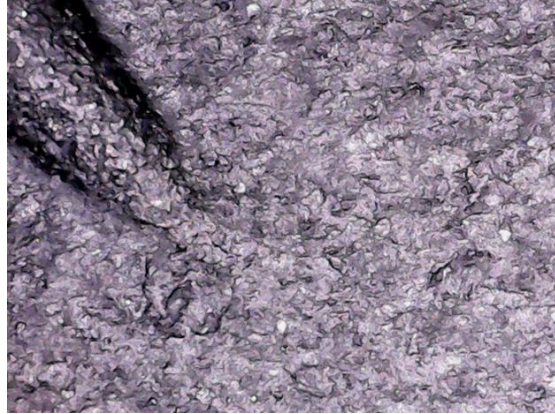
SafeRoute – Outdoor exposed 8-months black coupon
