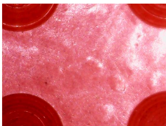
Armor-Tile – Outdoor exposed 12-months red coupon
