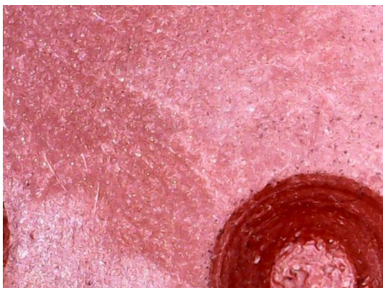
ADA Solutions – Outdoor exposed 20-months red coupon
