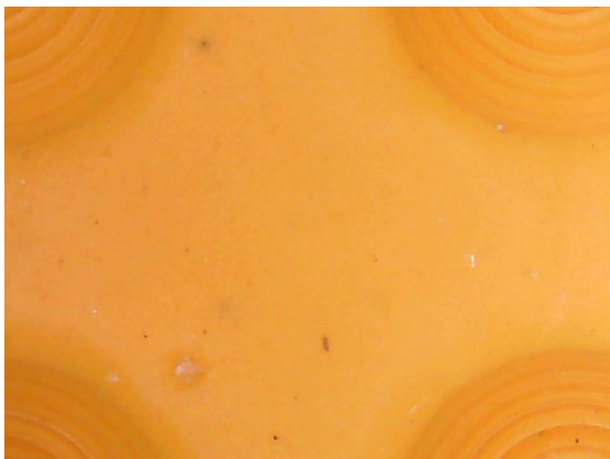
Armor-Tile – Xenon Condition [C] 3,000 hr.
