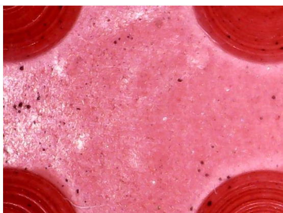
Armor-Tile – Outdoor exposed 20-months red coupon
