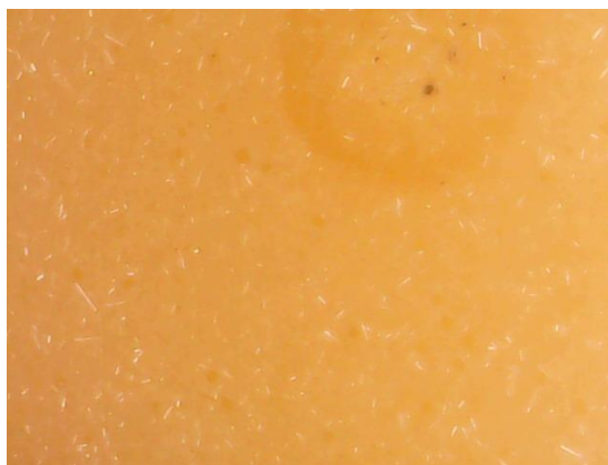
Redimat – Xenon Condition [A] 500hr.
