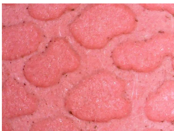
AlertCast – Outdoor exposed 20-months red coupon
