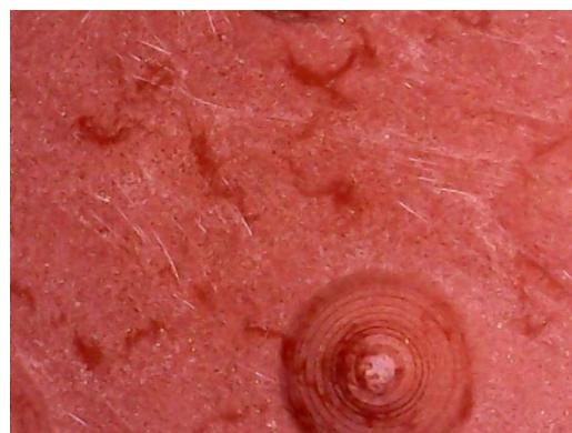
ADA Solution, Red – Condition [A], 2000 hr.
