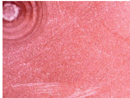
ADA Solution, Red – Condition [B], 2000 hr.
