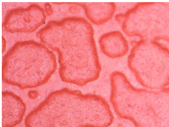
AlertCast – Outdoor exposed 12-months red coupon
