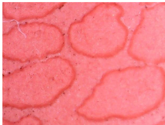
AlertCast – Outdoor exposed 16-months red coupon
