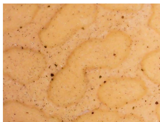
AlertCast – Outdoor exposed 24-months yellow coupon
