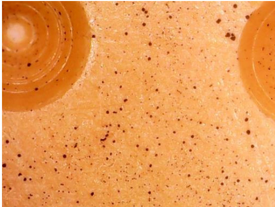
ADA Solutions – Original exposed 12 months yellow coupon
