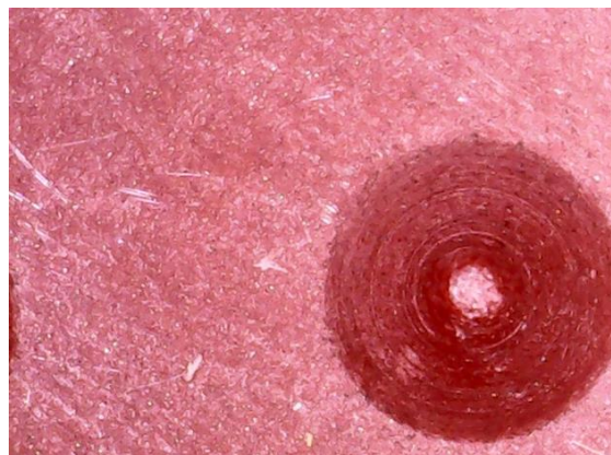
ADA Solutions – Outdoor exposed 24-months red coupon
