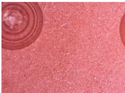
ADA Solution, Red-Condition [C], 1500 hr.
