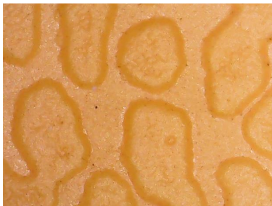
AlertCast – Outdoor exposed 8-months yellow coupon
