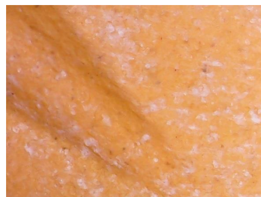
SafeRoute, Yellow – Condition [B], 2000 hr.
