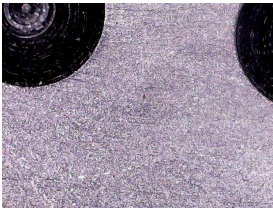
ADA Solutions – Outdoor exposed 8-months black coupon
