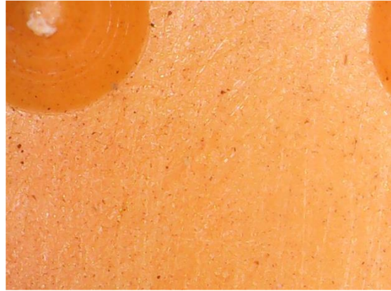
ADA Solutions – Outdoor exposed 8-months yellow coupon
