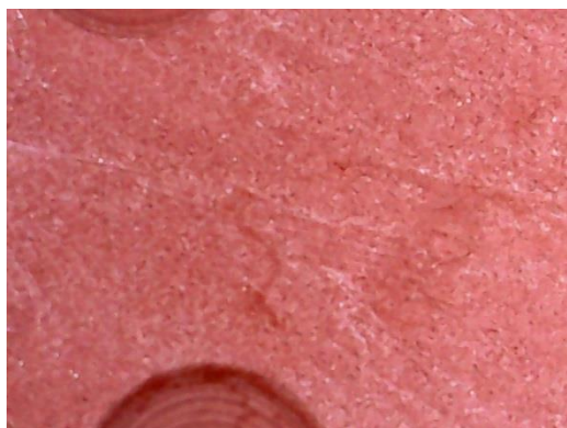
ADA Solution, Red-Condition [A], 1500 hr.
