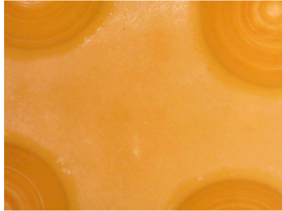
Armor-Tile – Xenon Condition [A] 3,000hr.
