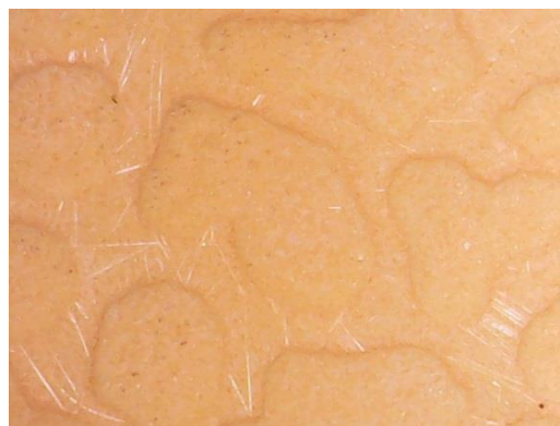
AlertCast, Yellow – Condition [C], 3000 hr.
