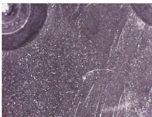
ADA Solution, Black – Condition [B], 3000 hr.
