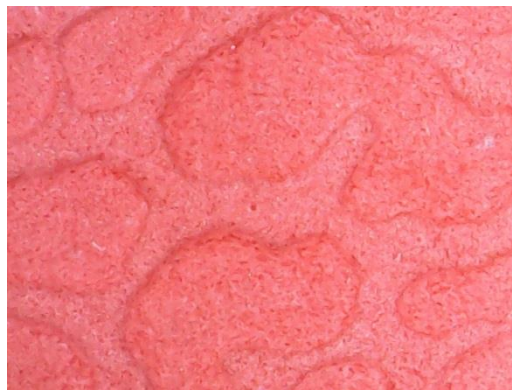
AlertCast, Red – Condition [B], 2000 hr.
