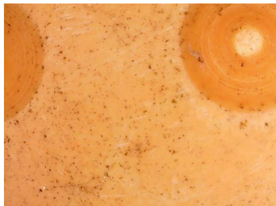
ADA Solutions – Outdoor exposed 24-months yellow coupon
