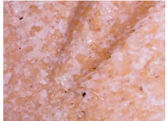
SafeRoute – Outdoor exposed 16-months yellow coupon
