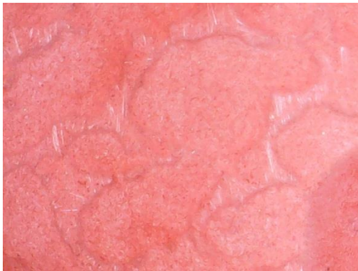
AlertCast, Red – Condition [C], 2500 hr.
