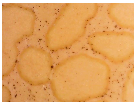
AlertCast – Outdoor exposed 16-months yellow coupon
