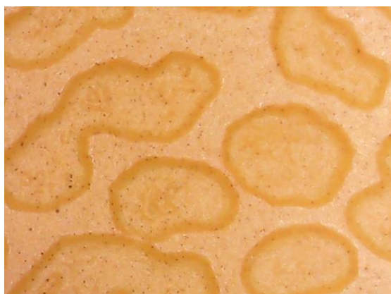
AlertCast – Outdoor exposed 12-months yellow coupon
