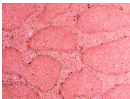
AlertCast – Outdoor exposed 24-months red coupon
