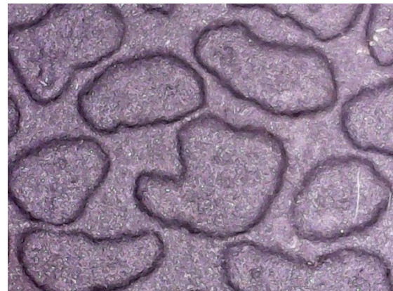
AlertCast – Outdoor exposed 24-months black coupon
