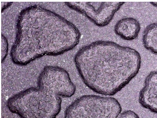
AlertCast – Outdoor exposed 20-months black coupon
