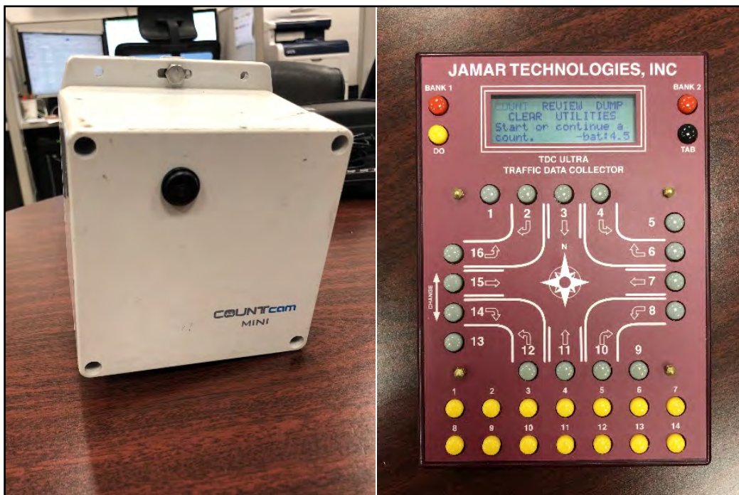
Figure 4. Traffic Recording Camera and Turning Movement Counting Box
