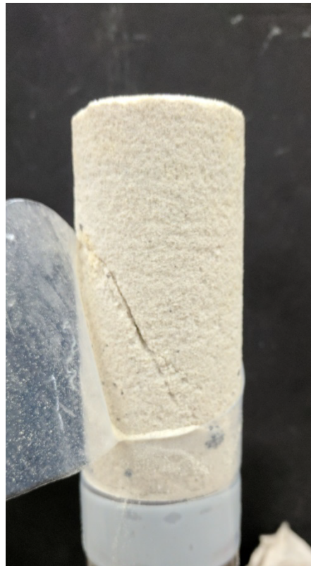
Figure G.8 Specimen SPSS 4 after triaxial compression ( \sigma_3=5 MPa)
