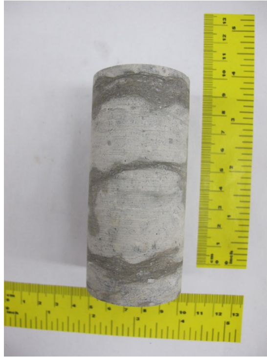
Figure E.7 Specimen x4 before triaxial compression test
