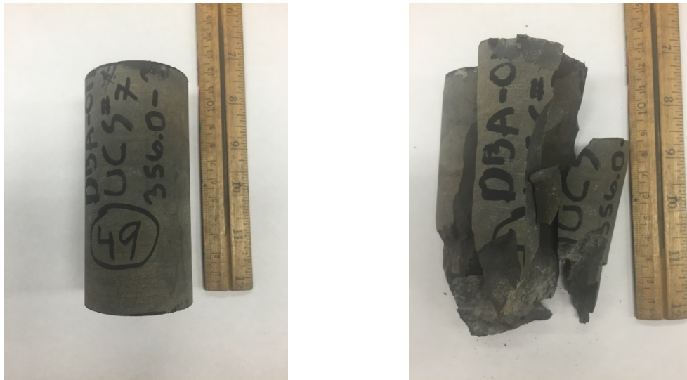
Figure A.96 Specimen 49: Before UCS test and After UCS test
