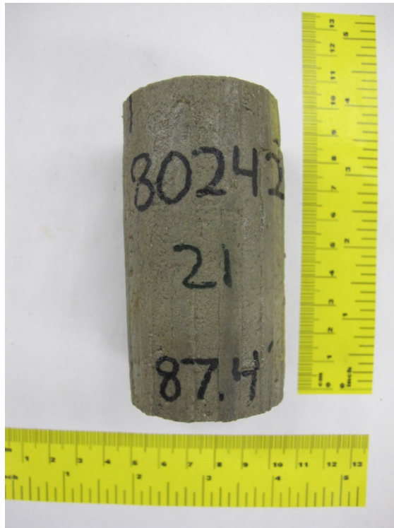
Figure F.28 Specimen 21 after triaxial compression ( \sigma_3=0 MPa, leaked)
