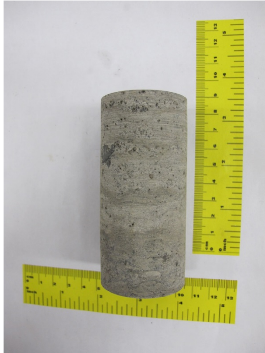
Figure E.9 Specimen x5 before triaxial compression test
