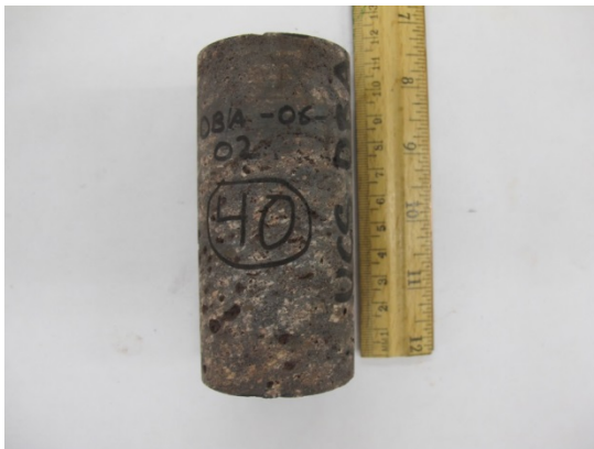
Figure A.79 Specimen 40: Before UCS test and After UCS test
