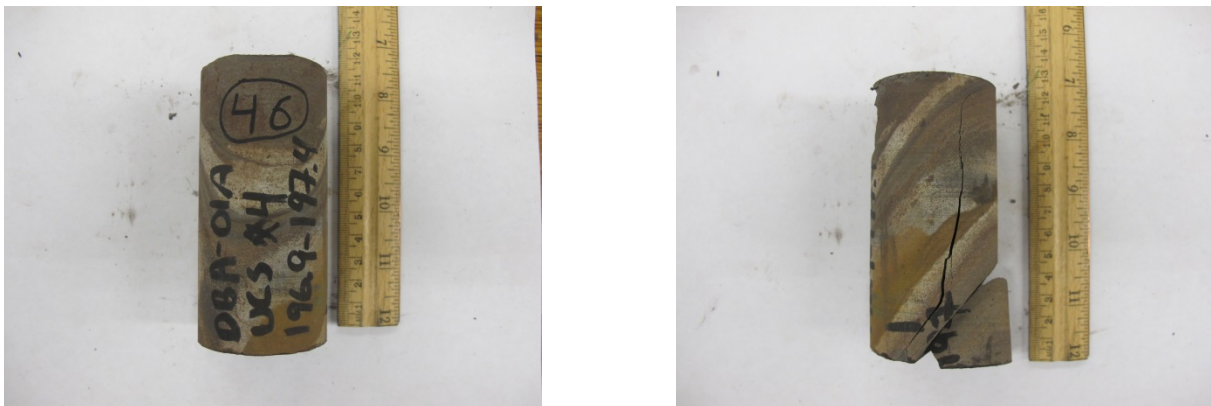
Figure A.90 Specimen 46: Before UCS test and After UCS test
