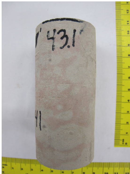
Figure F.12 Specimen 13 after triaxial compression ( \sigma_3=5 MPa)
