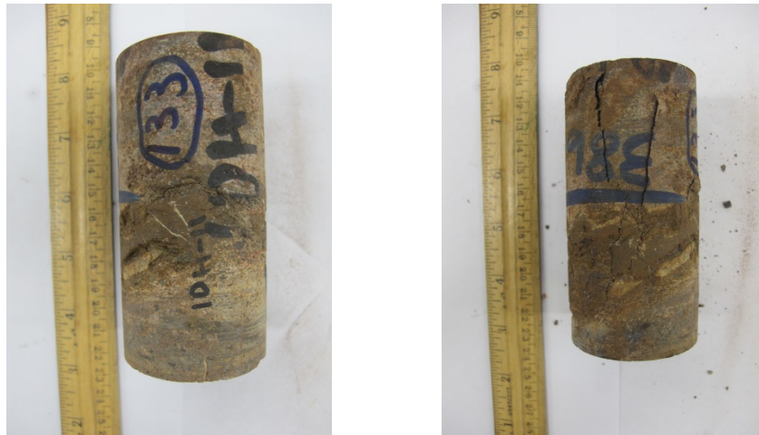
Figure A.263 Specimen 133: Before UCS test and After UCS test
