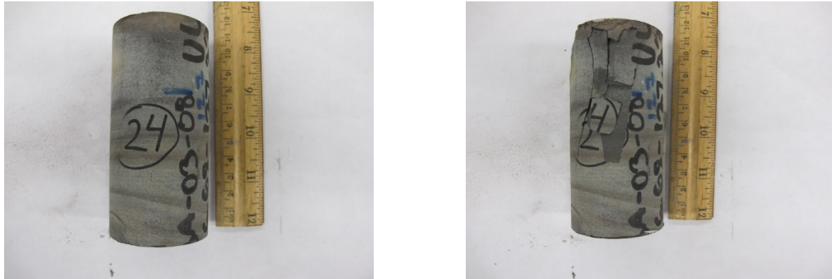
Figure A.47 Specimen 24: Before UCS test and After UCS test
