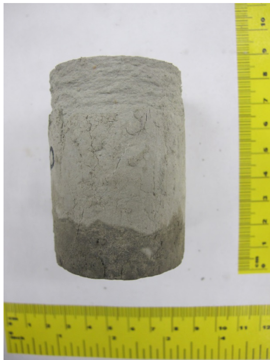
Figure F.4 Specimen 8 after triaxial compression ( \sigma_3=10 MPa)
