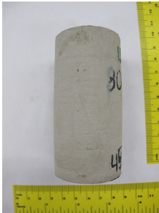
Figure F.16 Specimen 15 after triaxial compression ( \sigma_3 = 5 MPa)
