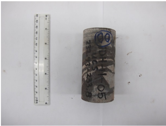
Figure A.197 Specimen 100: Before UCS test and After UCS test
