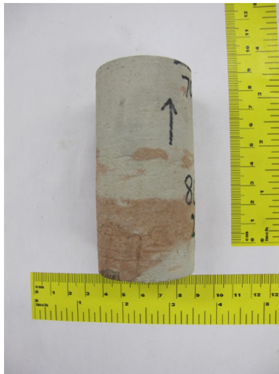
Figure F.30 Specimen 22 after triaxial compression ( \sigma_3=10 MPa)
