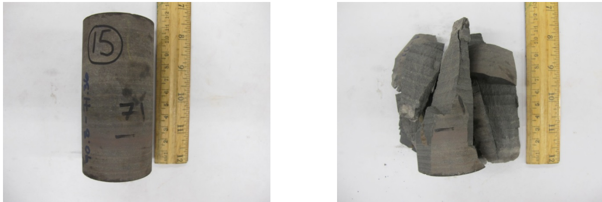
Figure A.29 Specimen 15: Before UCS test and After UCS test
