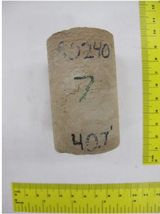
Figure F.1 Specimen 7 before triaxial compression
