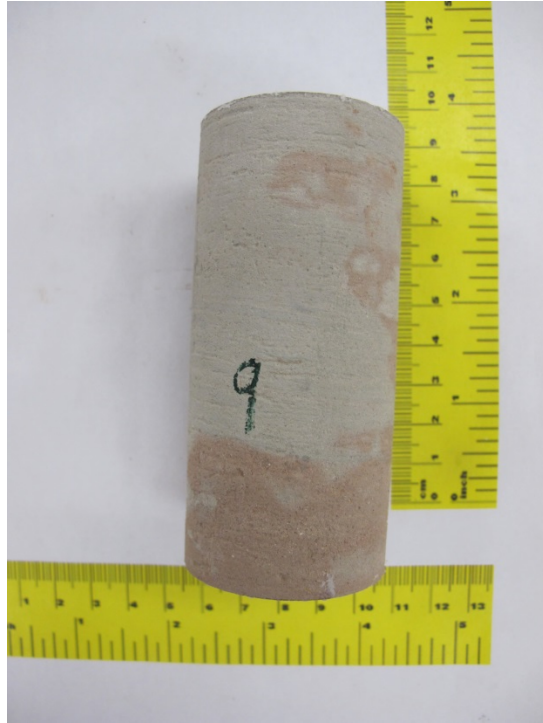
Figure F.5 Specimen 9 before triaxial compression
