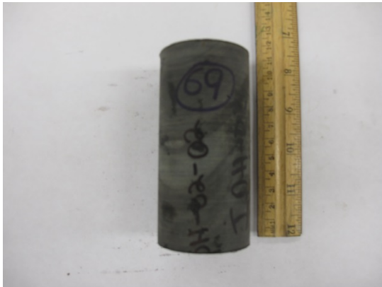
Figure A.136 Specimen 69: Before UCS test and After UCS test
