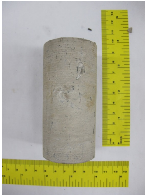
Figure E.2 Specimen x1 after triaxial compression test ( \sigma_3=5 MPa)
