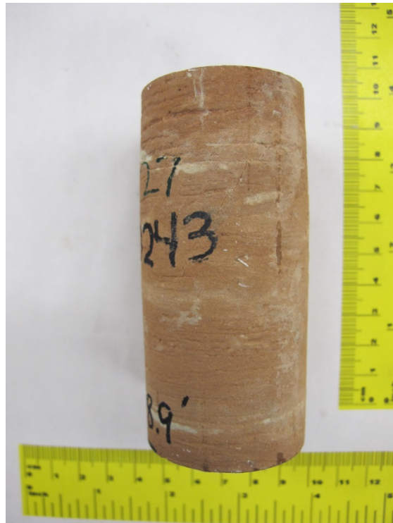
Figure F.40 Specimen 27 after triaxial compression ( \sigma_3=5 MPa)
