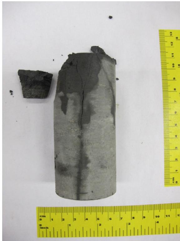
Figure E.12 Specimen x6 after triaxial compression test ( \sigma_3=20 MPa)
