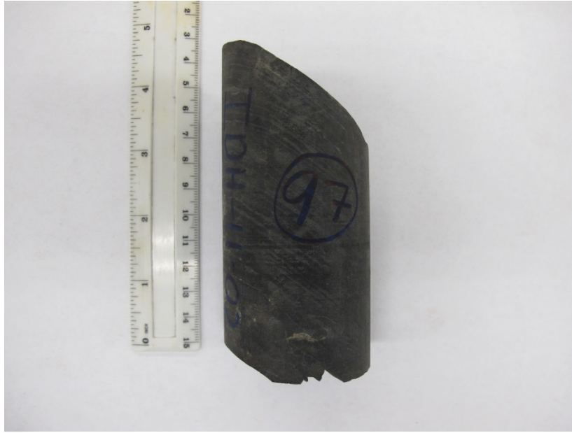
Figure A.191 Specimen 97: Fracture occurred during cutting portion of preparation
