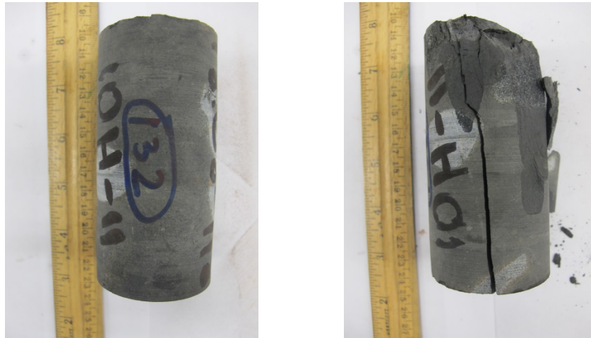
Figure A.261 Specimen 132: Before UCS test and After UCS test
