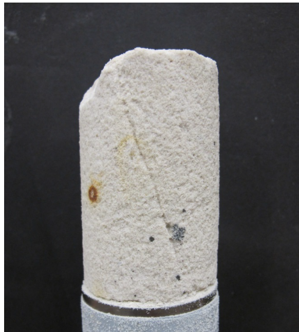
Figure G.6 Specimen SPSS 3 after triaxial compression ( \sigma_3=2.5 MPa)
