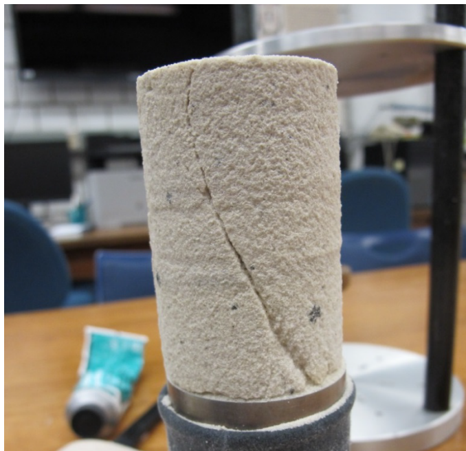
Figure G.2 Specimen 28 after triaxial compression ( \sigma_3=1 MPa)
