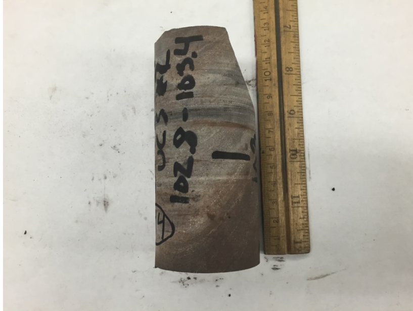
Figure A.86 Fracture in specimen 44 occurred during cutting portion of preparation
