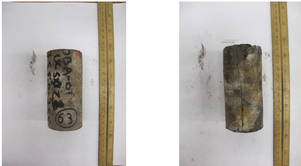
Figure A.124 Specimen 63: Before UCS test and After UCS test
