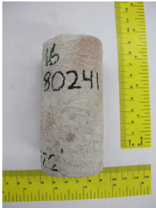
Figure F.18 Specimen 16 after triaxial compression ( \sigma_3=2.5 MPa)
