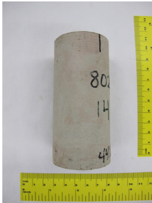
Figure F.14 Specimen 14 after triaxial compression ( \sigma_3=10 MPa)
