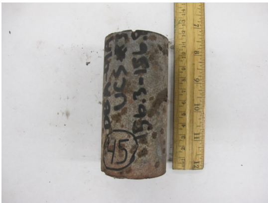
Figure A.88 Specimen 45: Before UCS test and After UCS test
