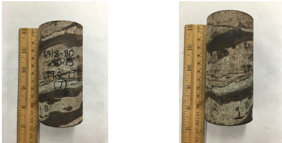
Figure A.13 Specimen 7: Before UCS test and After UCS test
