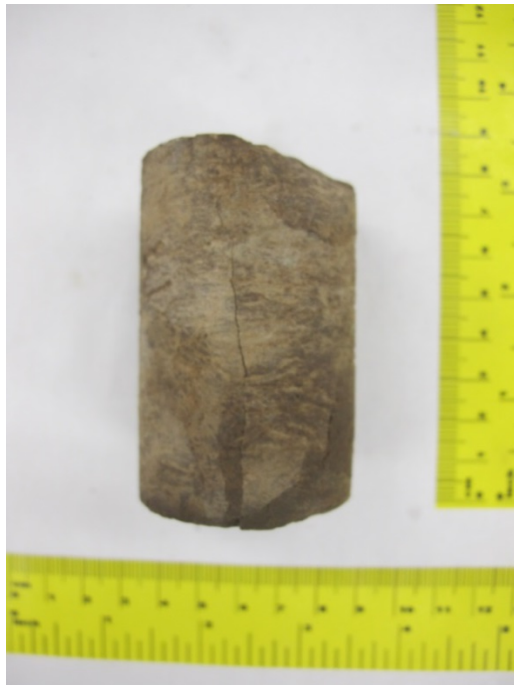
Figure F.2 Specimen 7 after triaxial compression ( \sigma_3=2.5 MPa)
