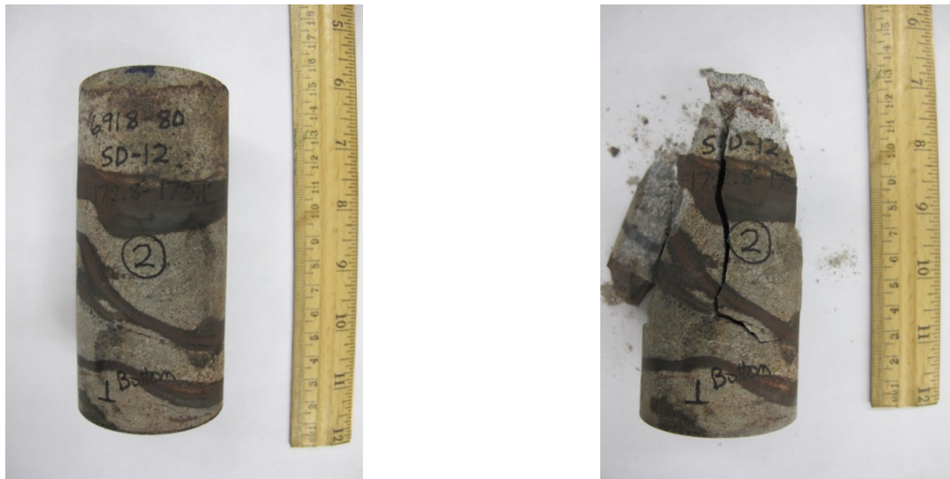
Figure A.4 Specimen 2: Before USC test and After UCS test
