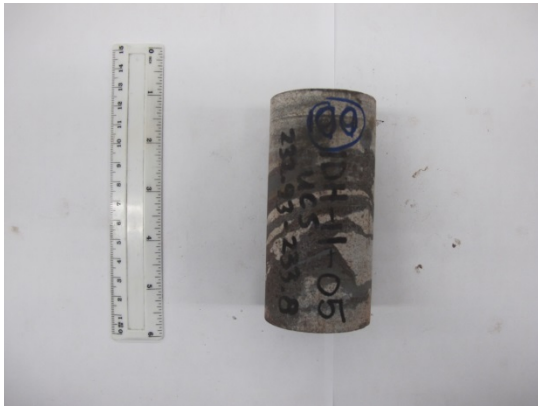
Figure A.217 Specimen 110: Before UCS test and After UCS test
