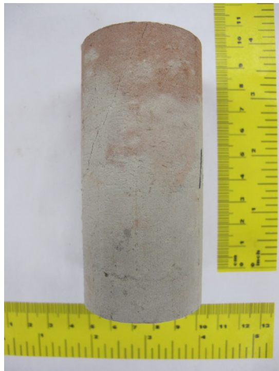
Figure F.24 Specimen 19 after triaxial compression ( \sigma_3=2.5 MPa)
