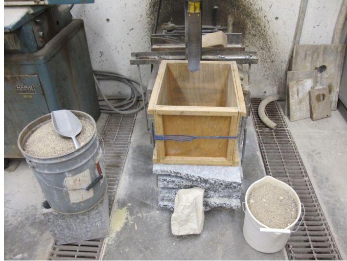
Figure G.9 St. Peter Sandstone coring setup. Sandstone block (bottom-middle) placed in wood contained (middle) and confined with compacted sand (bottom left and bottom right). Wood container then clamped down while dry coring with toothed core barrel (top-middle).
