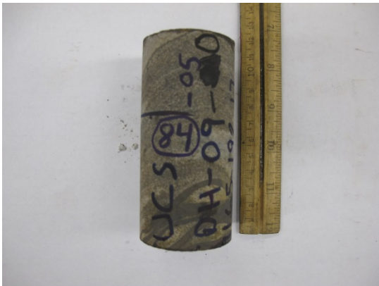
Figure A.166 Specimen 84: Before UCS test and After UCS test
