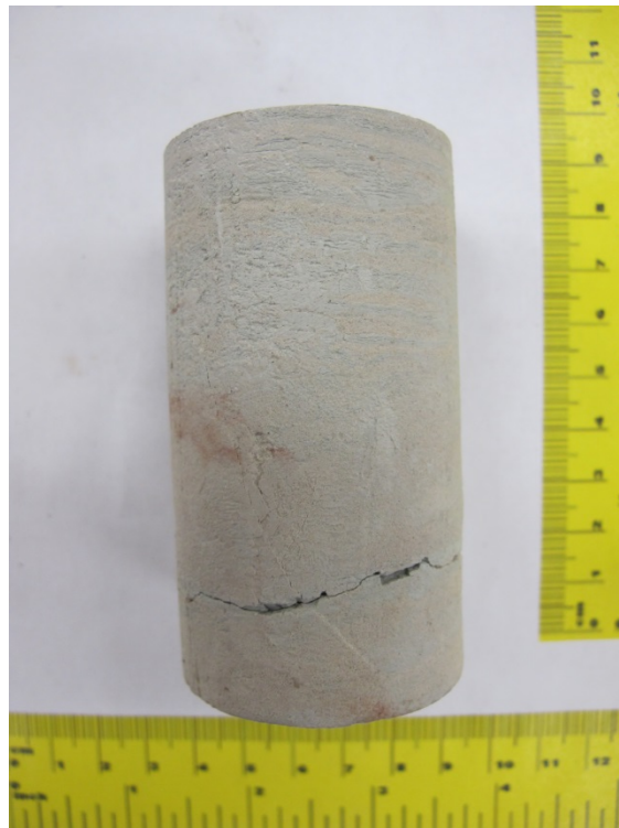
Figure F.26 Specimen 20 after triaxial compression ( \sigma_3=2.5 MPa)
