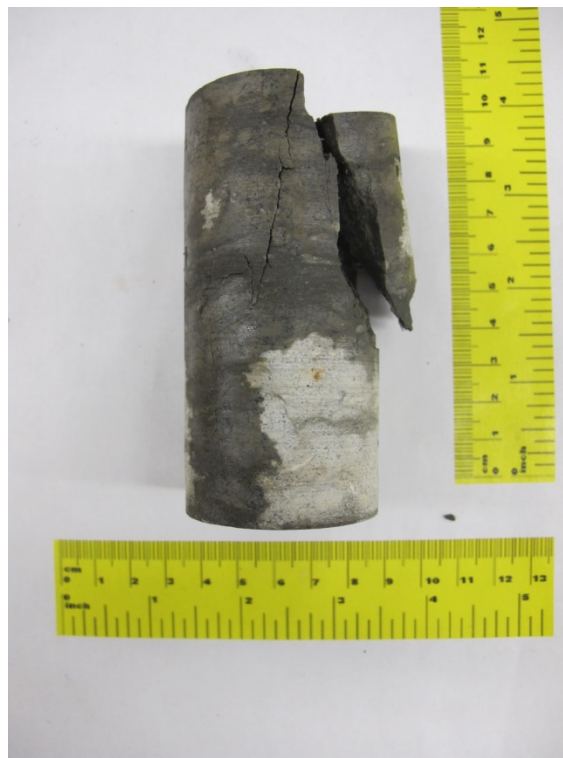
Figure E.8 Specimen x4 after triaxial compression test ( \sigma_3=5 MPa)
