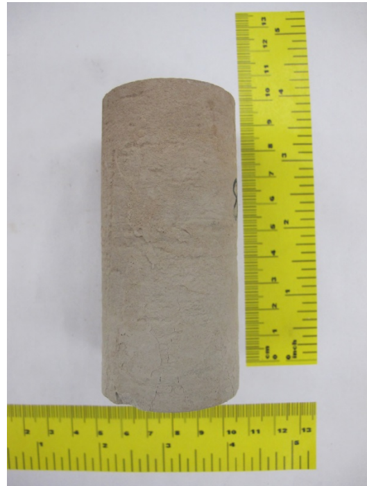
Figure F.8 Specimen 10 after triaxial compression ( \sigma_3=2.5 MPa)
