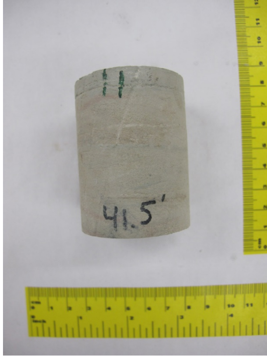
Figure F.9 Specimen 11 before triaxial compression
