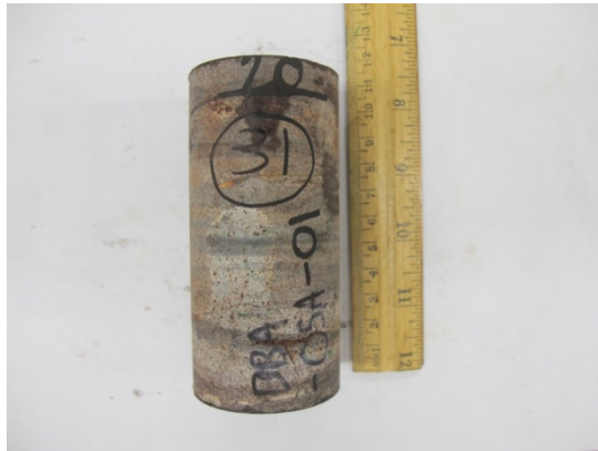
Figure A.61 Specimen 31: Before UCS test and After UCS test
