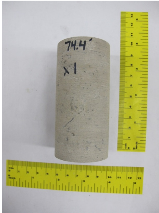
Figure E.1 Specimen x1 before triaxial compression test
