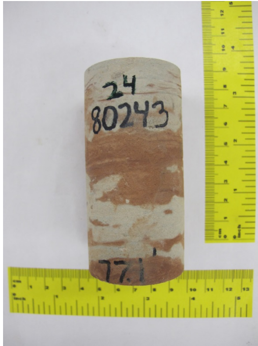
Figure F.33 Specimen 24 before triaxial compression
