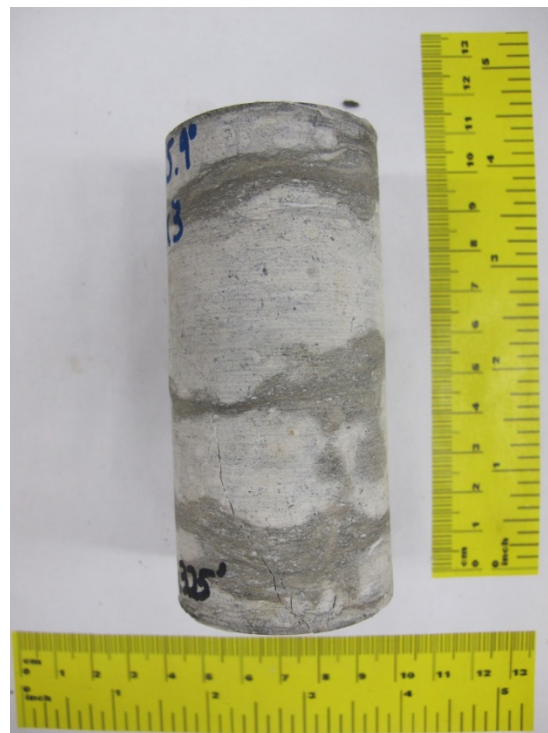
Figure E.6 Specimen x3 after triaxial compression test ( \sigma_3=20 MPa)
