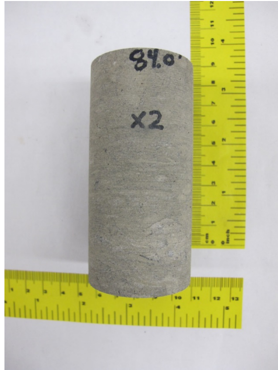
Figure E.3 Specimen x2 before triaxial compression test
