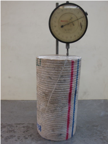
Figure 3.8 Core on surface table with dial indicator.
