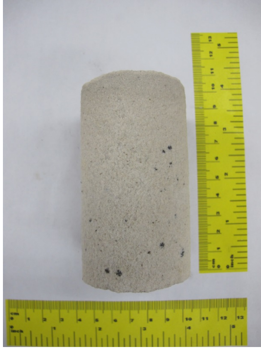
Figure G.3 Specimen SPSS 2 before triaxial compression
