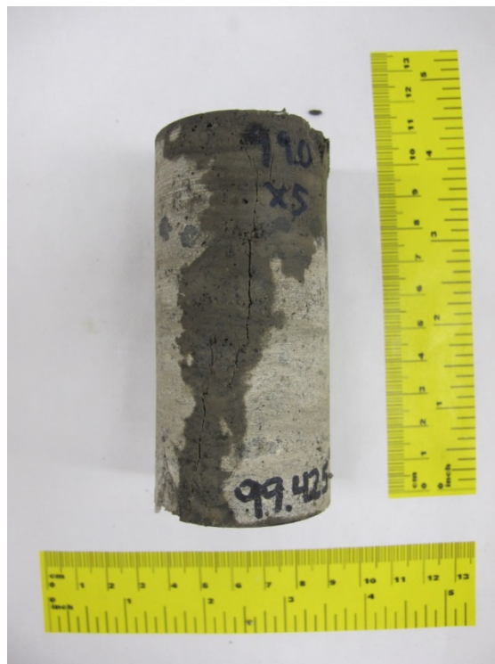
Figure E.10 Specimen x5 after triaxial compression test ( \sigma_3=10 MPa)
