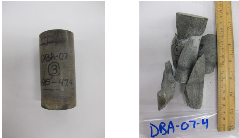
Figure A.219 Specimen 111: Before UCS test and After UCS test
