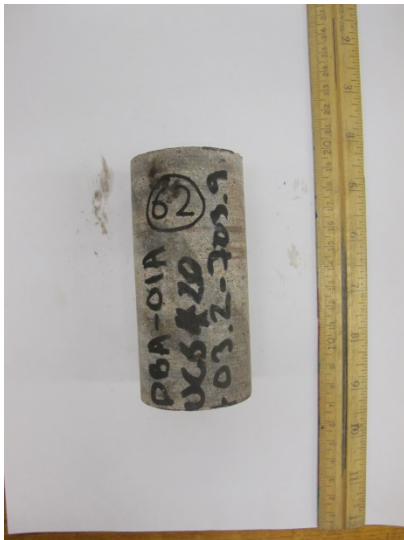
Figure A.122 Specimen 62: Before UCS test and After UCS test
