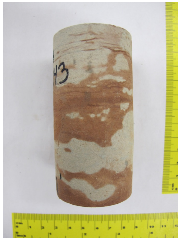
Figure F.34 Specimen 24 after triaxial compression ( \sigma_3=5 MPa)
