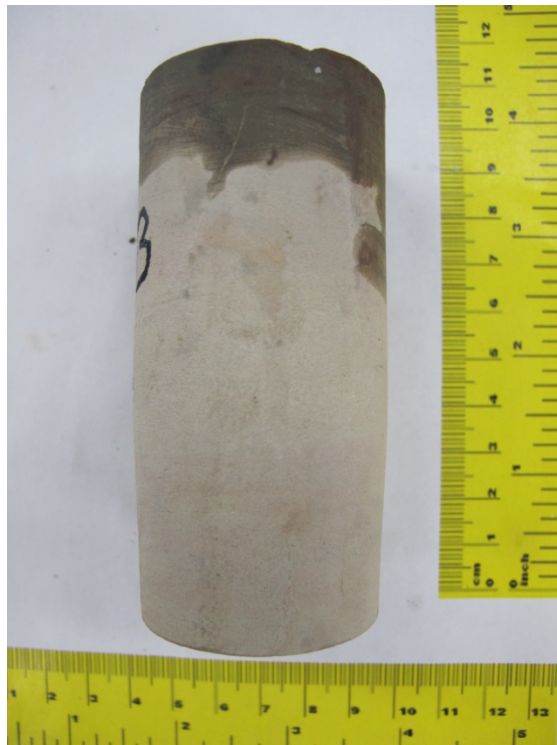
Figure F.36 Specimen 25 after triaxial compression ( \sigma_3=10 MPa)
