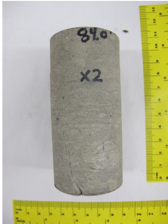
Figure E.4 Specimen x2 after triaxial compression test ( \sigma_3=10 MPa)
