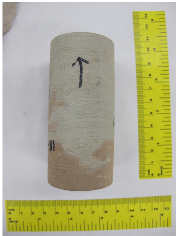
Figure F.6 Specimen 9 after triaxial compression ( \sigma_3=5 MPa)
