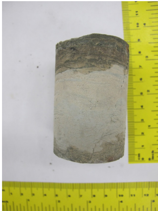
Figure F.32 Specimen 23 after triaxial compression ( \sigma_3=7.5 MPa)
