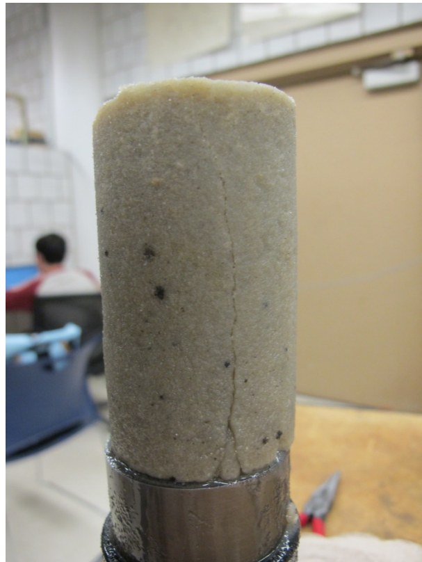
Figure G.4 Specimen SPSS 2 after compression ( \sigma_3=0 MPa)
