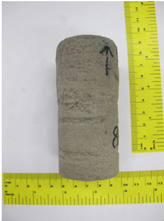
Figure F.20 Specimen 17 after triaxial compression ( \sigma_3=0 MPa, leaked)
