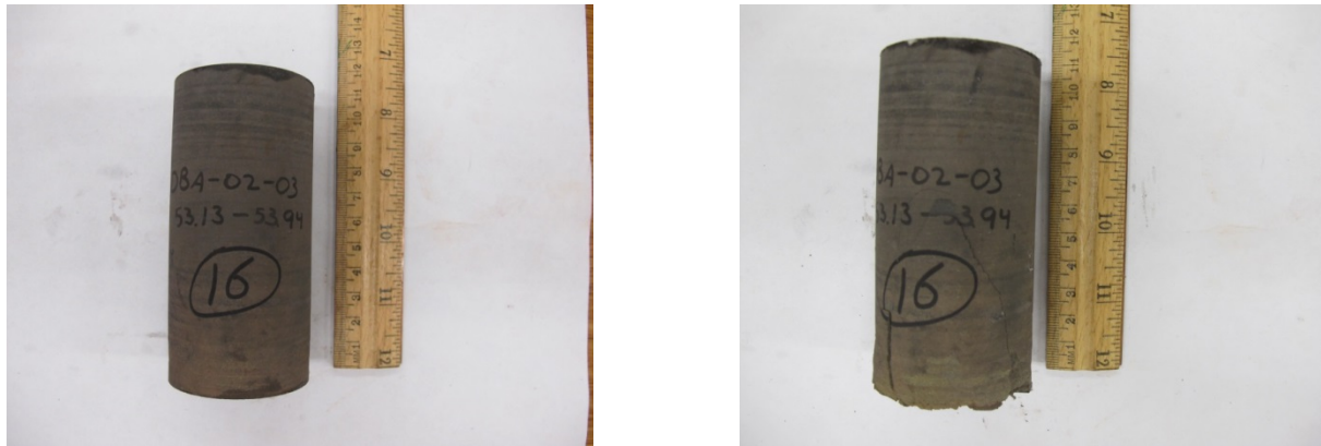
Figure A.31 Specimen 16: Before UCS test and After UCS test
