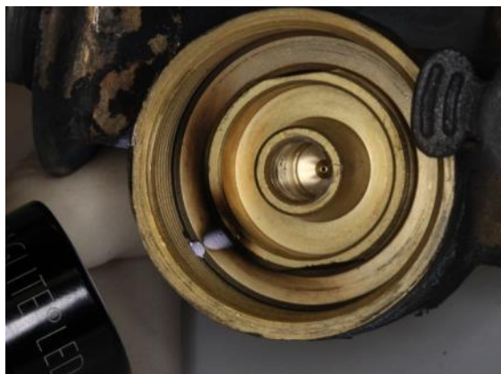
Figure 10 – Regulator Atmospheric Vent Port Illuminated from Exterior
