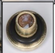
D - Regulator Assembly, PTFE Piston, Spring and Inlet Filter (lubricant on filter surface)
