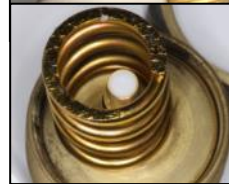
D - Regulator Assembly, PTFE Piston, Spring and Inlet Filter (lubricant on filter surface)
