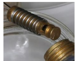
D - Regulator Assembly, PTFE Piston, Spring and Inlet Filter (lubricant on filter surface)
