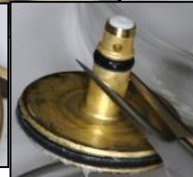
D - Regulator Assembly, PTFE Piston, Spring and Inlet Filter (lubricant on filter surface)
