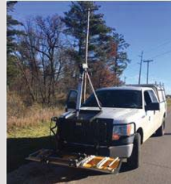
Figure 1 (left): FDH rapid bridge deck scanning
