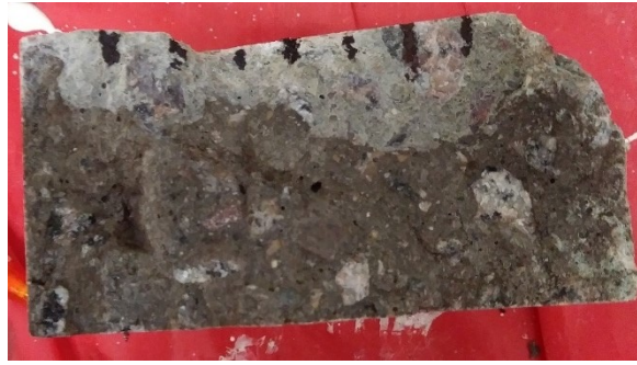
Figure 3.2 Concrete sample from Bridge 62892 (Mackubin St., Saint Paul) with epoxy topping (left) and no epoxy topping (right) after the NT Build 492 test
