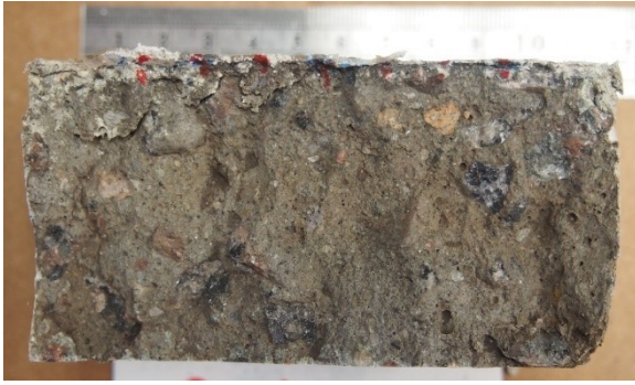
Figure 3.2 Concrete sample from Bridge 62892 (Mackubin St., Saint Paul) with epoxy topping (left) and no epoxy topping (right) after the NT Build 492 test
