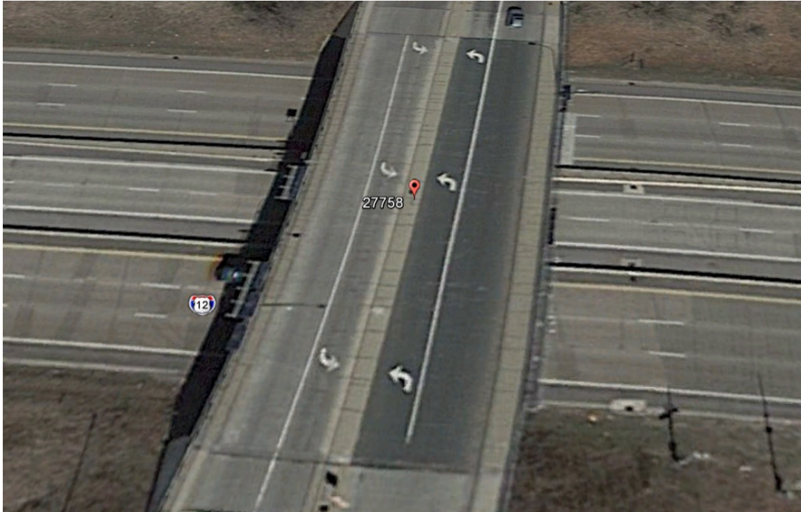
Figure 6.12 Bridge 27758 (Penn Ave. over I-394 in Minneapolis, MN) with a thin polymer overlay on the northbound lane (right lane) and a Methymethacrylate flood seal on the southbound lane (left lane) placed in 2007
