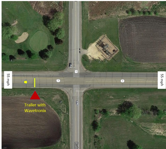
Tentative location of trailer with Wavetronix (© 2017 Google)
