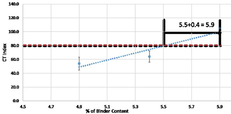
Figure 4.2. IDEAL-CT Test Results for Mix 1.
