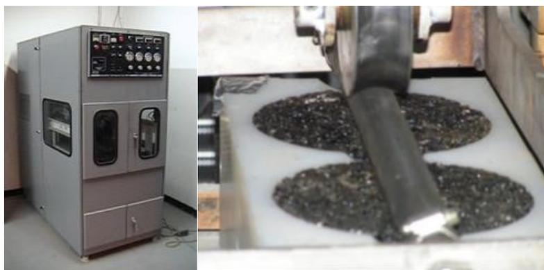
Figure 2.17. APA; a) Equipment Overview, (b) Close-Up View of the Loaded Specimen (Mahoney et al. 2011).
