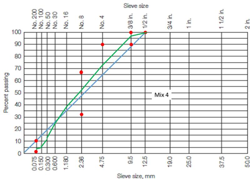
Figure 3.4. Gradation for Mix 4 (0.375 in (9.5 mm) Superpave, Non-Carbonate, Level 4).
