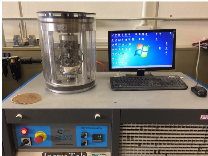
Figure 2.19. Asphalt Mixture Performance Tester for FN Test.
