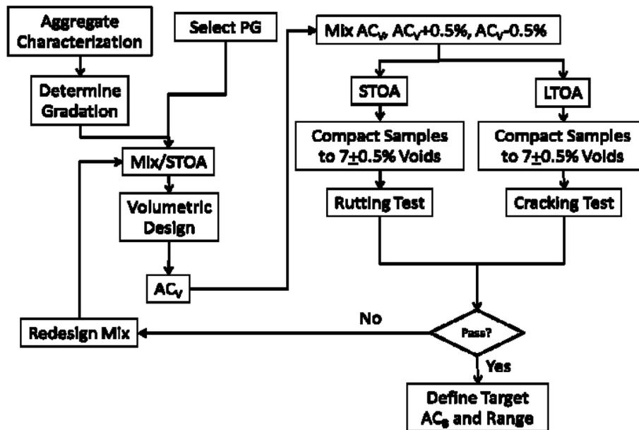
Figure 3.6. Flow Chart of BMD Approach Using Volumetric Data as a Starting Point.
