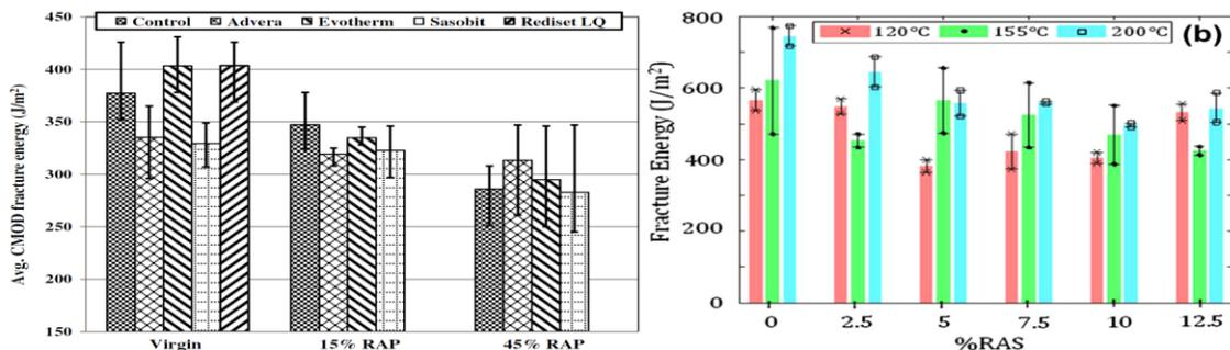
(b) Fracture energy vs. RAP (Hill et al. 2013) (c) Fracture energy vs. RAS (Arnold et al. 2014)
