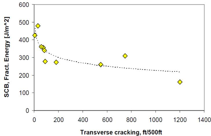
**Figure 2.9. Field Data Suggesting a Minimum SCB Fracture Energy of 350 J/m<sup>2</sup> to Prevent Thermal Cracking (Marasteanu et al. 2012).**
