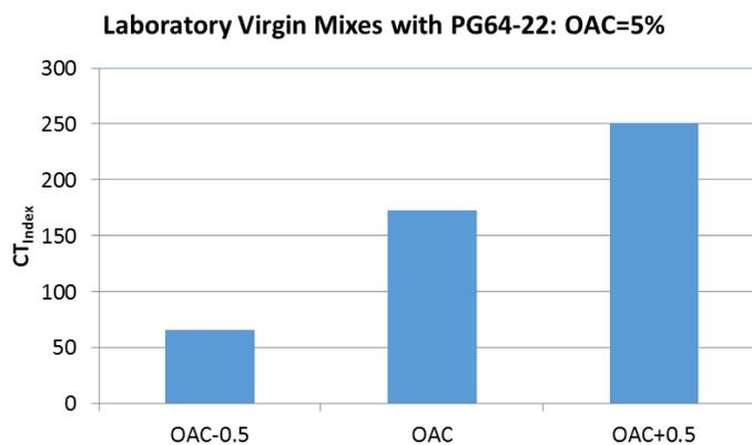
Figure 2.16. IDEAL-CT Sensitivity to Asphalt Content.
