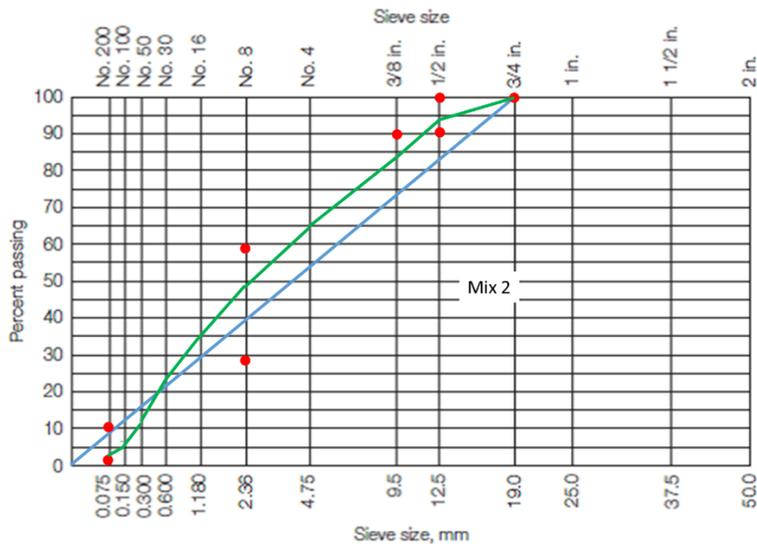
Figure 3.2. Gradation for Mix 2 (0.5 in (12.5 mm) Superpave, Non-Carbonate, Level 4).
