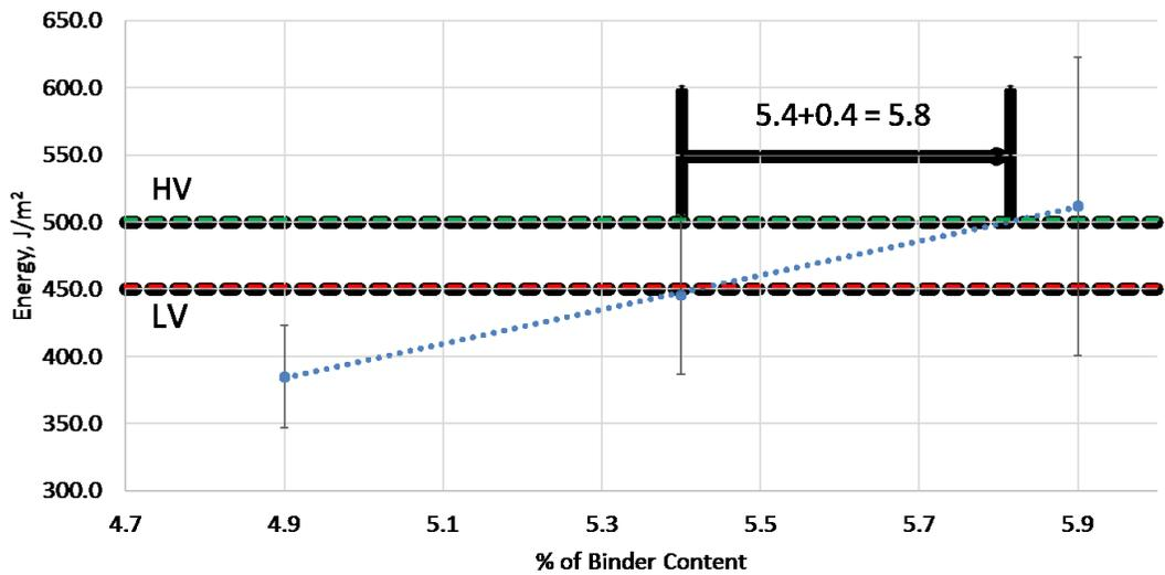
Figure 4.3. DCT Test Results for Mix 1.
