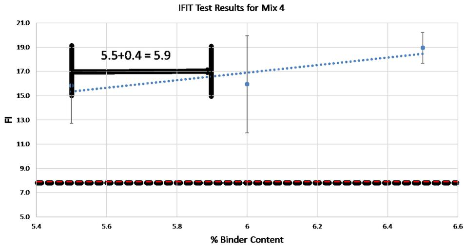
Figure 4.13. I-FIT Results for Mix 4.
