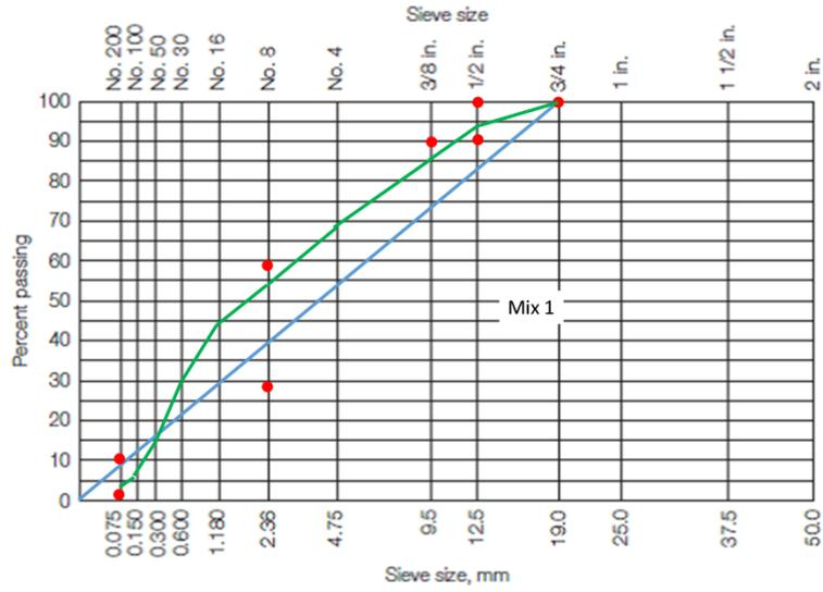
Figure 3.1. Gradation for Mix 1 (0.5 in (12.5 mm) Superpave, Carbonate, Level 3).
