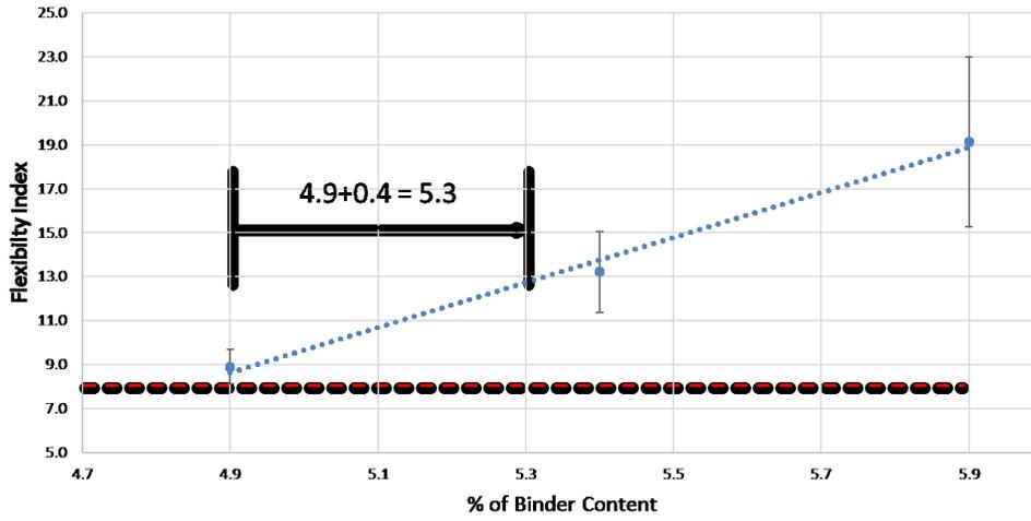
Figure 4.5. I-FIT Results for Mix 2.
