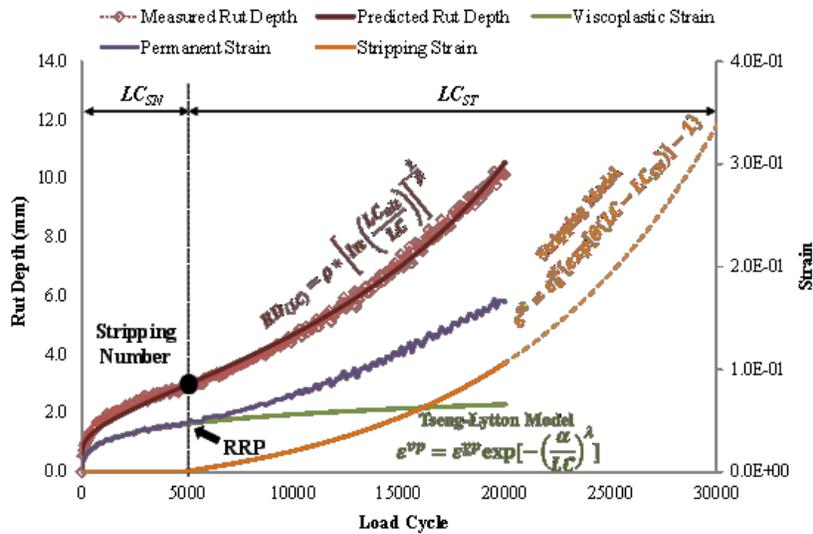
Figure 2.20. HWTT Analysis Methodology (Yin et al. 2014).
