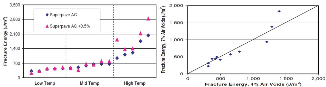
(a) Fracture energy vs. test temperature, asphalt content, and air voids (Braham et al. 2007)
