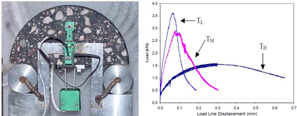
**Figure 2.6. SCB Test Setup, LLD Extensometer, and Typical Plot of SCB Test at Different Temperatures:  $T_L$ -12 ° C below  $T_M$ ,  $T_M$ -binder PG low limit+10 ° C, and  $T_H$ -12 ° C above  $T_M$  (Li and Marasteanu, 2004).**
