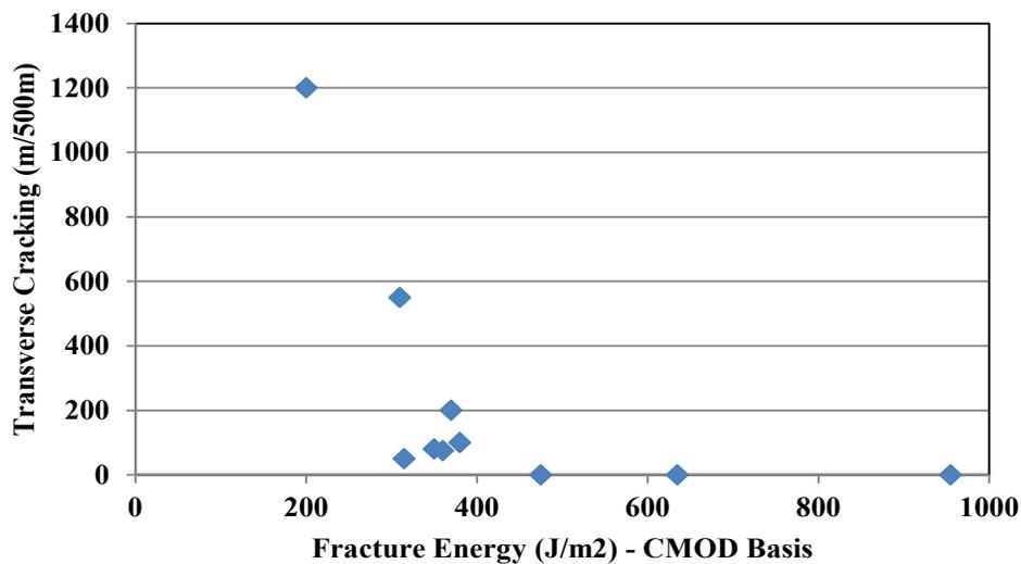
Figure 2.5. Correlation between DCT and Thermal Cracking (Marasteanu et al. 2012).
