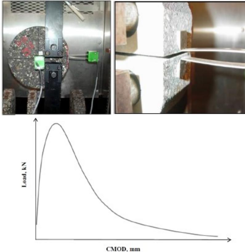
**Figure 2.3. DCT Test Setup, CMOD Gauge, and Typical Test Curve (Marasteanu et al. 2012).**
