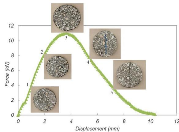
Figure 2.14. Force-Displacement (FD) Curve for IDEAL-CT.
