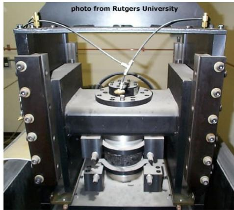
**Figure 1.3. Superpave Shear Tester (from PavementInteractive.org).**
