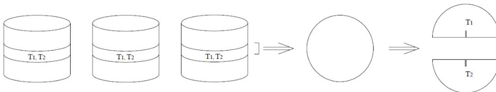
**Figure 2.7. SCB Specimen Preparation (AASHTO T105-13).**
