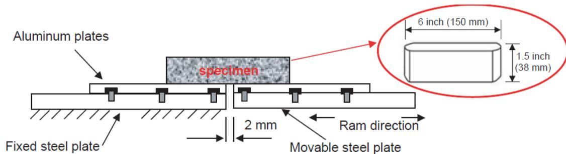
**Figure 2.11. Schematic of Upgraded TTI OT.**
