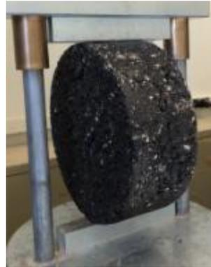
Figure 2.13. Test Set-Up for Indirect Tension Asphalt Cracking Test (IDEAL-CT).
