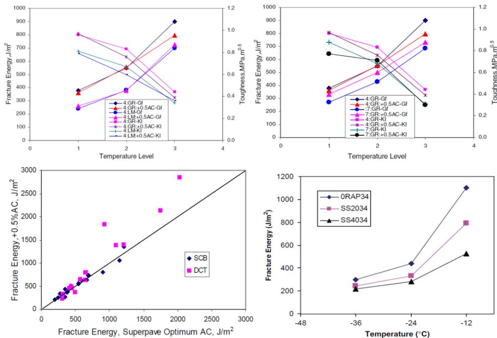
Figure 2.8. Sensitivity SCB Fracture Energy to Mix Compositions and Design Parameters (Li et al. 2008).
