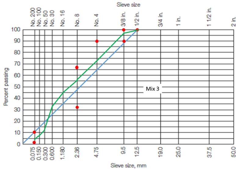
Figure 3.3. Gradation for Mix 3 (0.375 in (9.5 mm) Superpave, Carbonate, Level 3).
