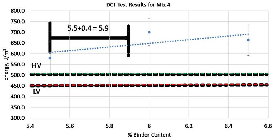
Figure 4.15. DCT Test Results for Mix 4.
