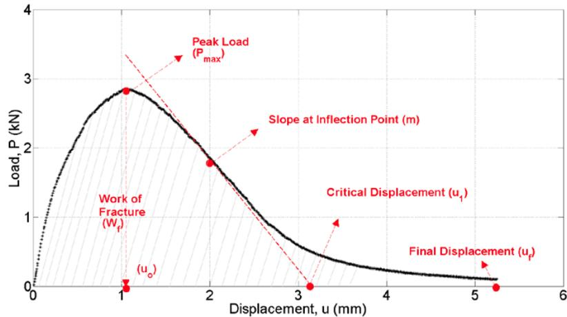
**Figure 2.10. Parameters for Determining the Flexibility Index.**
