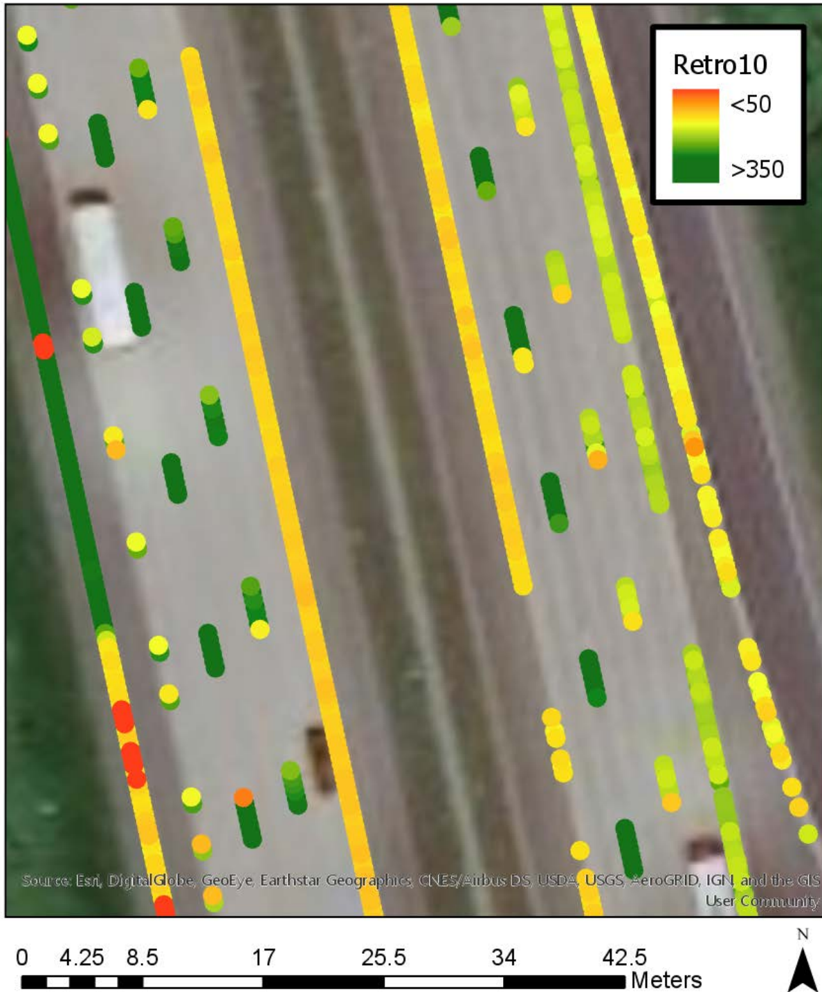
Figure 12.9: Example output of the csv2gdb.py script showing the retro feature class colored by retroreflectivity values.
