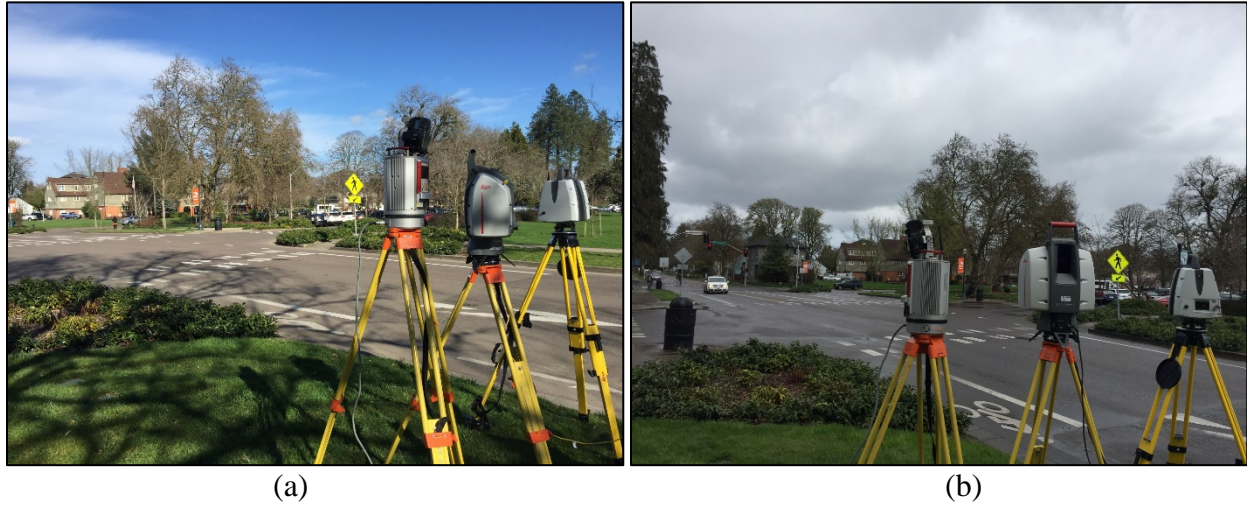
Figure 7.3: Data collection under (a) dry and (b) wet conditions with three laser scanners.
