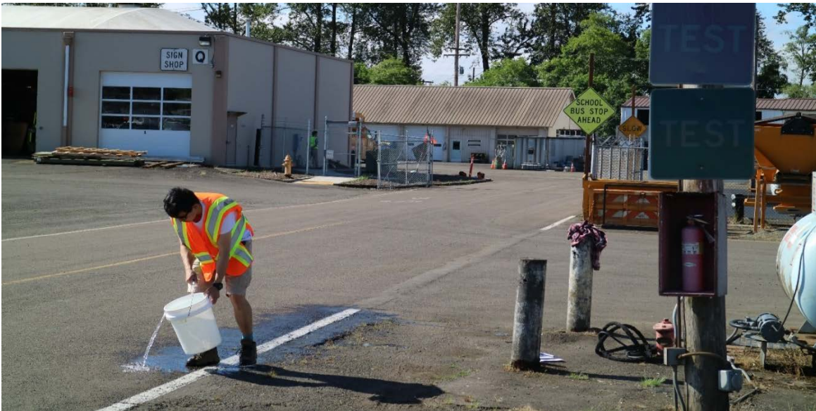
Figure 8.1: A project team member wets pavement with bucket prior to pass T07.
