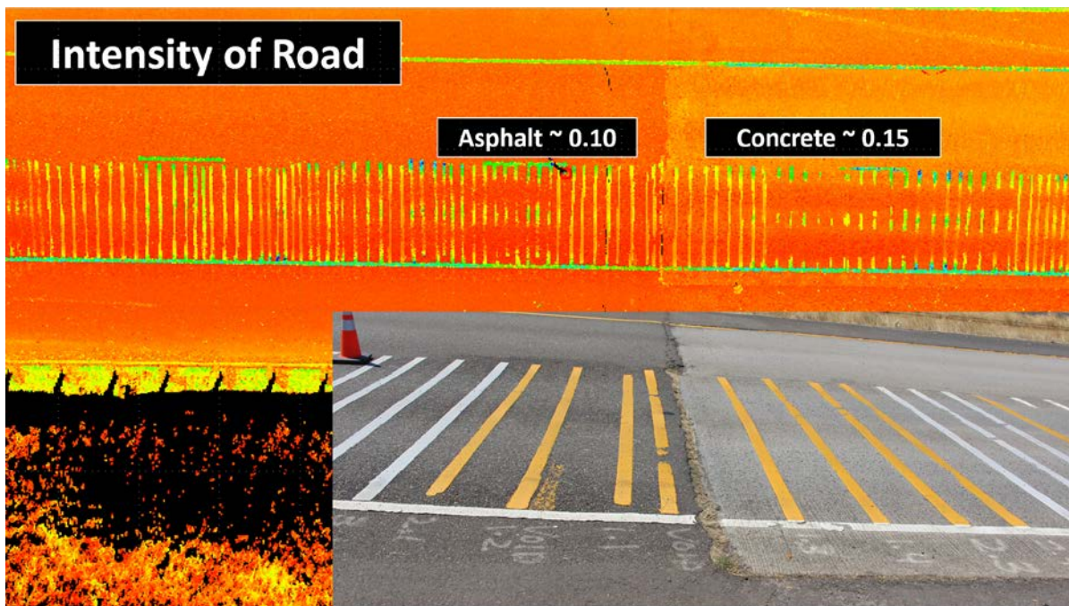
Figure 4.5: Example plan view of data at Testdeck at the asphalt/concrete interface colored by intensity values. Blue indicates high intensity while red indicates low intensity. An oblique photograph at the interface is included for reference purposes. The figure shows typical intensity values for asphalt (~0.10) and concrete (~0.15).
