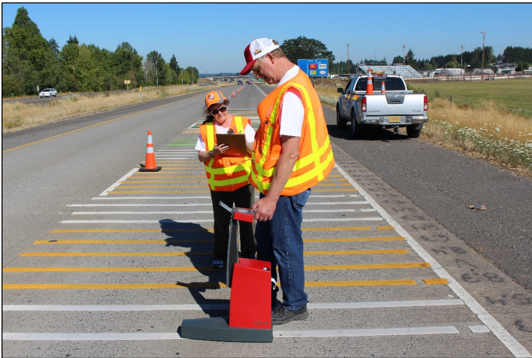
Figure 4.3: Acquisition of retroreflectivity readings with a Delta LTL-X Handheld retroreflectometer.
