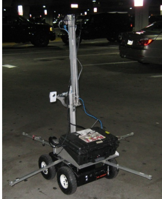
Figure 15. Robotic Roadway Lighting Mobile Measurement System (RRLMMS).
