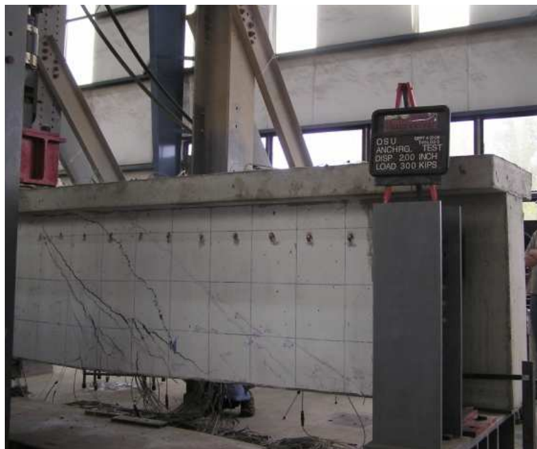
Fig. 4.7 – Specimen T.45.Ld3.(5) digital photograph at failure
