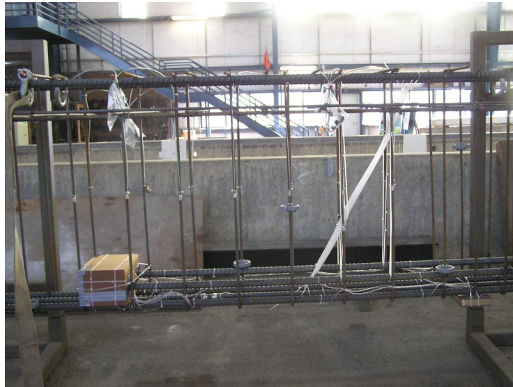
Fig. 3.9 – Example of specimen geometry prior to concrete placement
