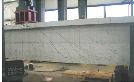
Fig. 5.32 – Specimen 8T12-B3 load-deflection plot and failure photo (Higgins, et al. 2004)
