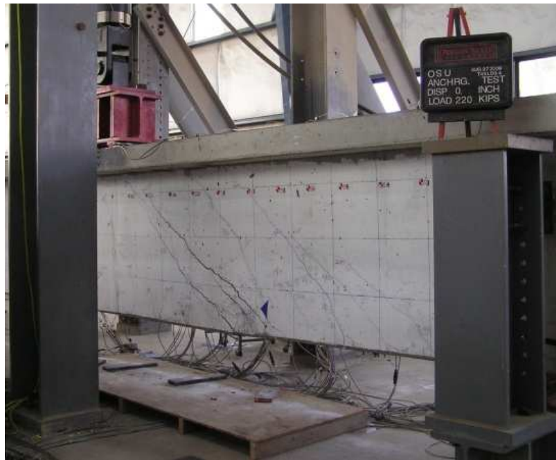
Fig. 4.6 – Specimen T.45.Ld3.(4) digital photograph at failure
