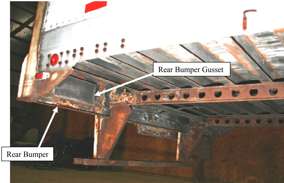
Figure 29. Photograph. Rear bumper and rear bumper gusset locations on semitrailer
