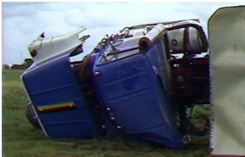
Figure 99. Photograph. Post test view of test vehicle illustrating damage to tractor due to roll-over
