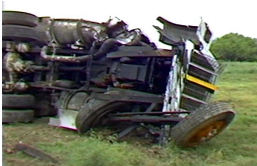
Figure 98. Photograph. Post test view of test vehicle illustrating damage to tractor
