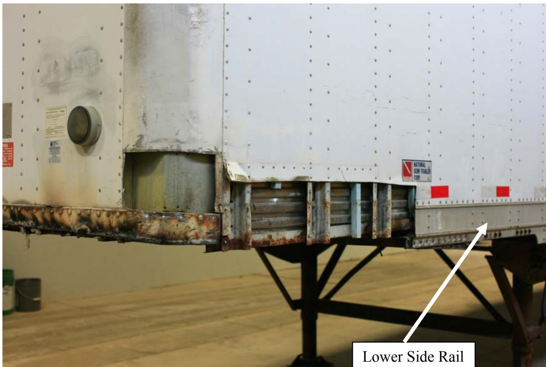
Figure 30. Photograph. Lower side rail location on semitrailer
