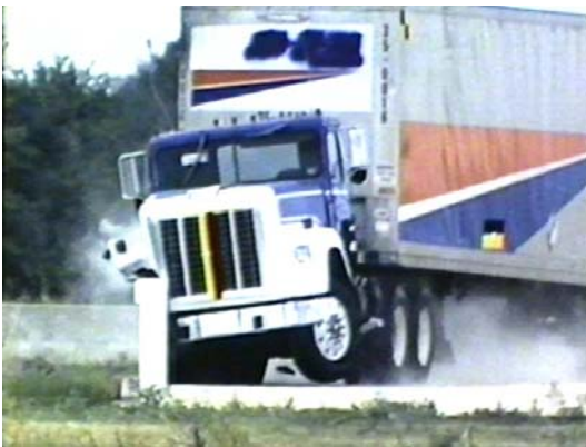
Figure 76. Photograph / Illustration. Sequential views of TTI Test 7069-13 and FE model simulation from a downstream viewpoint
