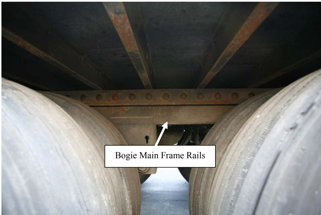
Figure 26. Photograph. Bogie main frame rails location on semitrailer
