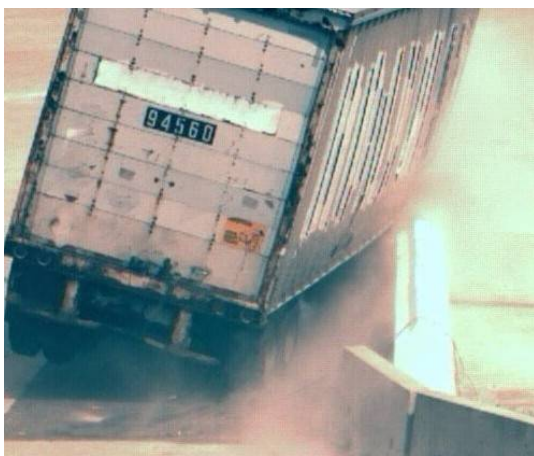
Figure 44. [CONTINUED] Photograph / Illustration. Sequential views of MwRSF Test TL5CMB-2 and FE Model simulation from an upstream viewpoint
