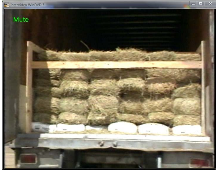
Figure 74. Photo. Trailer ballast for TTI test 7069-10
