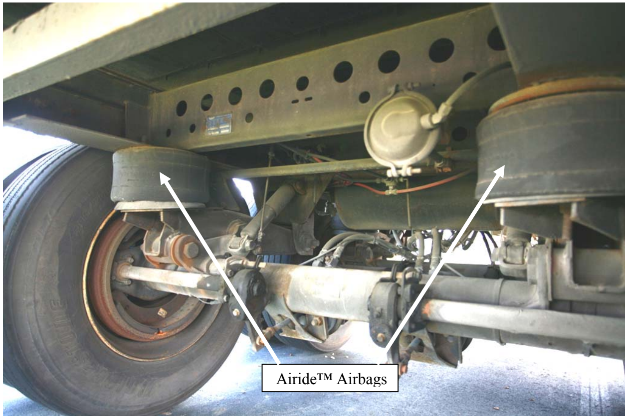
Figure 2. Photograph. Airide™ Airbag location on semitrailer
