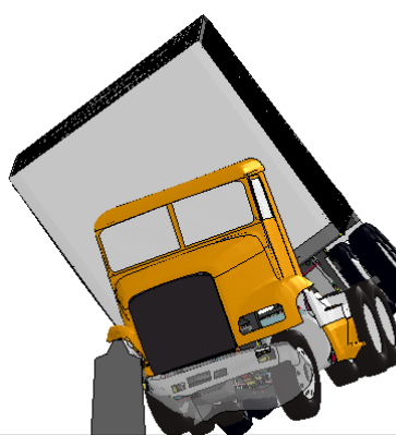
Figure 43. [CONTINUED] Photograph / Illustration. Sequential views of MwRSF Test TL5CMB-2 and FE model simulation from a downstream viewpoint
