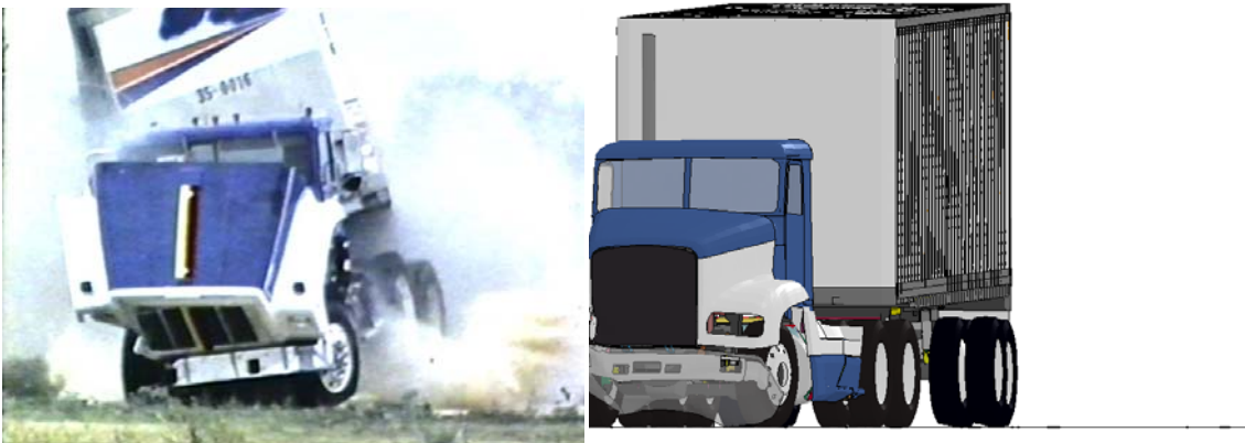
Figure 76. [CONTINUED] Photograph / Illustration. Sequential views of TTI Test 7069-13 and FE model simulation from a downstream viewpoint
