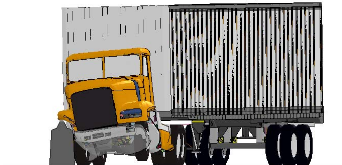
Figure 43. Photograph / Illustration. Sequential views of MwRSF Test TL5CMB-2 and FE model simulation from a downstream viewpoint
