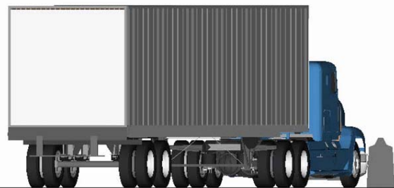
Figure D-1. Photograph / Illustration. Views of FLD 120 Tractor and 48-foot Stoughton semitrailer vehicles and FE corresponding models
