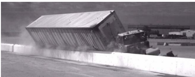
Figure 45. [CONTINUED] Photograph / Illustration. Sequential views of MwRSF Test TL5CMB-2 and FE model simulation from an isometric viewpoint
