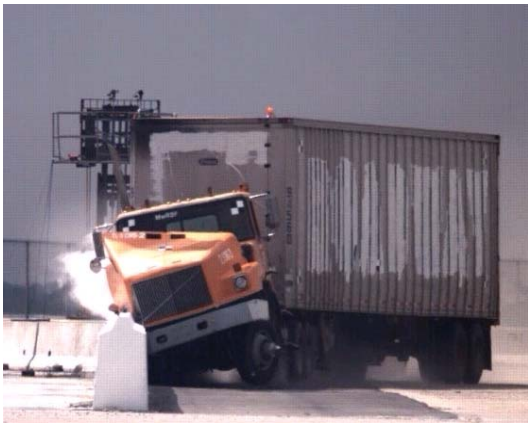
Figure 43. Photograph / Illustration. Sequential views of MwRSF Test TL5CMB-2 and FE model simulation from a downstream viewpoint
