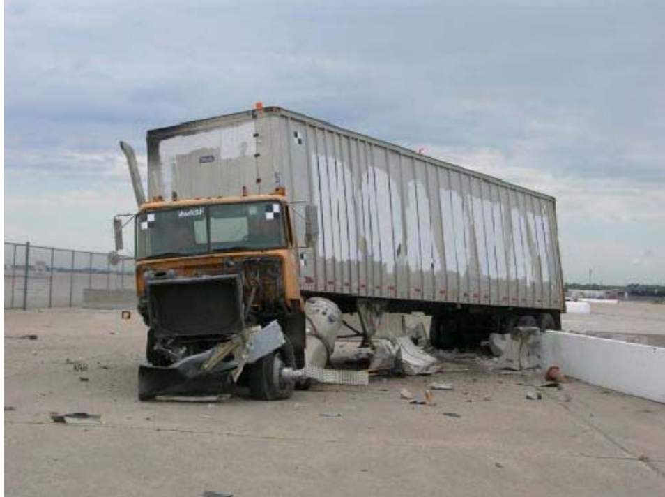
Figure 60. Photograph. Post test view of test vehicle illustrating excessive damage after secondary impact
