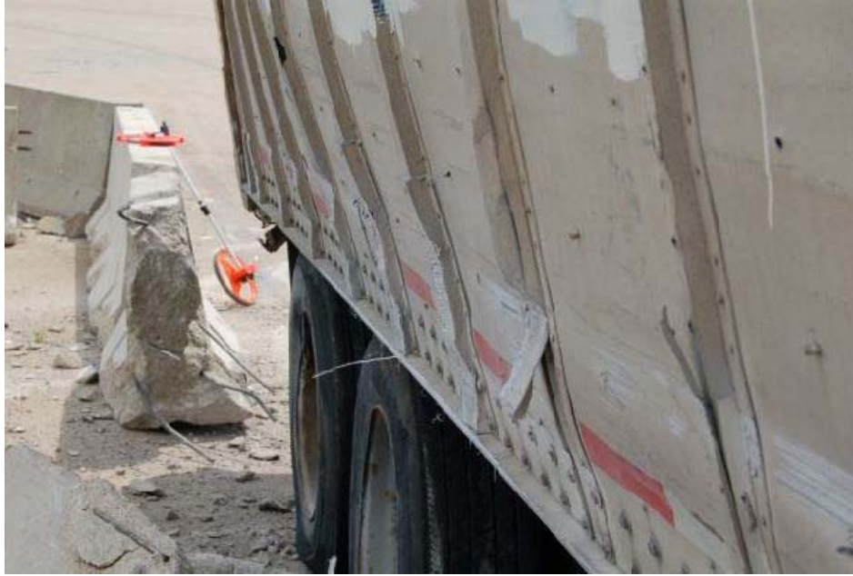
Figure 61. Photograph. Post test view of the trailer showing damage to sidewall and external ribs
