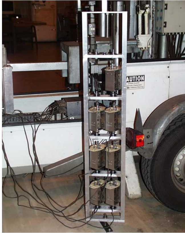
Figure 124. Photo. Seismometer stand with sensors attached.
