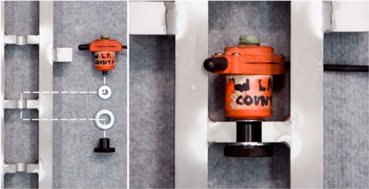
Figure 119. Photo. Attachment of a JILS or Carl Bro geophone to the stand.
