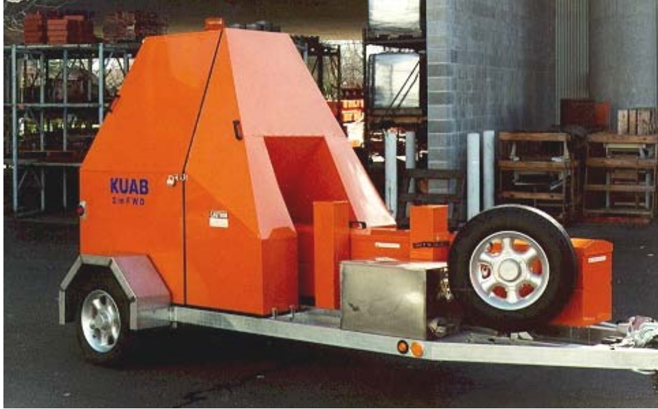
Figure 9. Photo. KUAB FWD with sensors aligned toward the tow vehicle.
