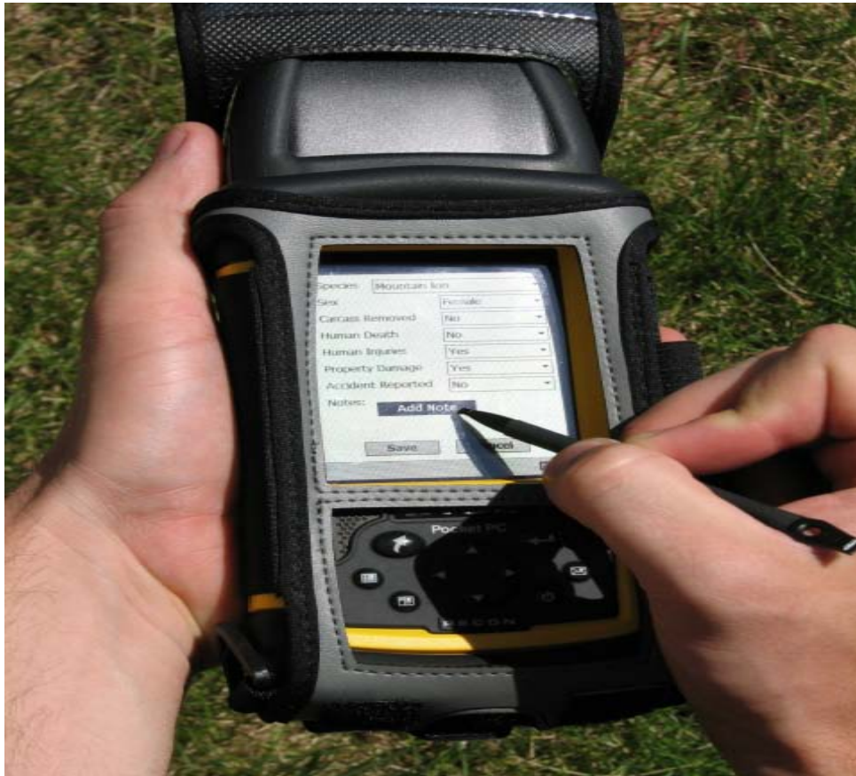
Figure 3: Photo. An integrated PDA-GPS handheld data collector developed and used in Phase II of the ROCS project.
