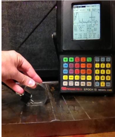
Figure 3.1 Photograph of an ultrasonic transducer detecting a defect in a steel weld
