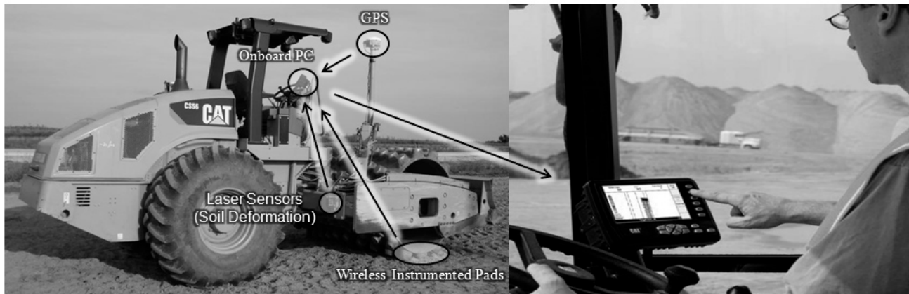
Figure 1. Concept of real-time soil compaction monitoring for static pad foot rollers. Wireless instrumented pads provide soil stiffness measurements, which are spatially referenced by GPS and provided to the operator via an onboard computer and monitor.
