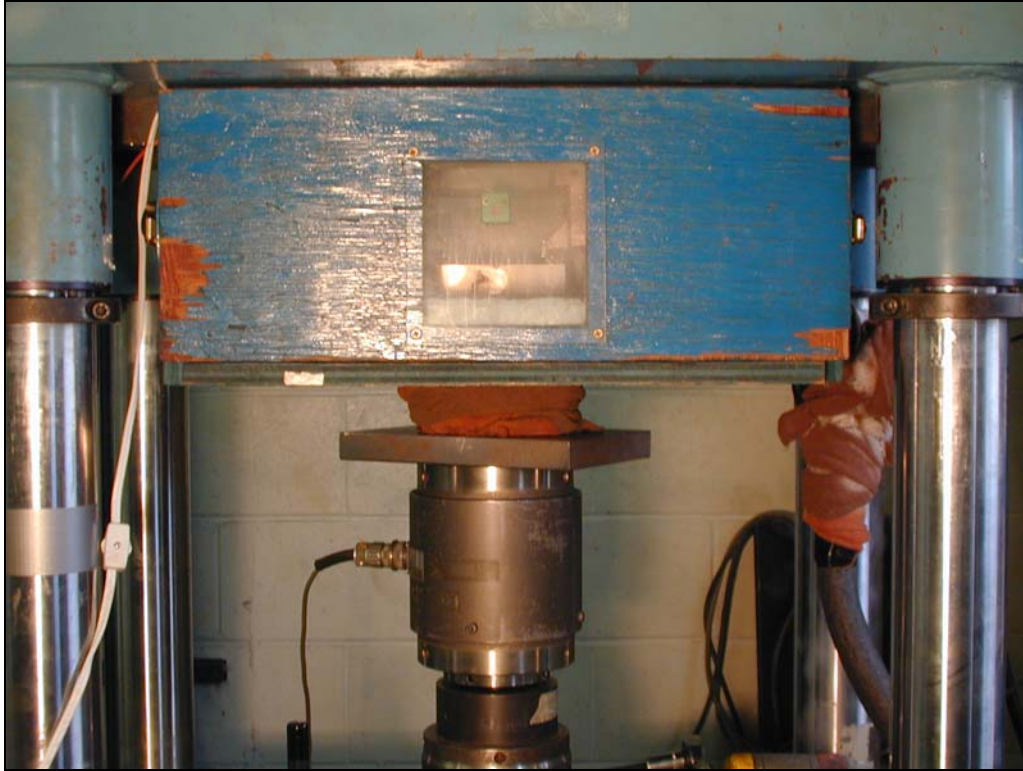
Figure 6.87: CTOD Test Set up
