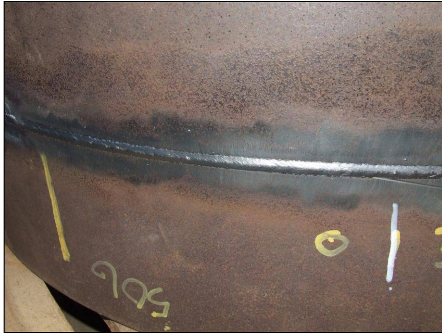
Figure 6.35: Typical Face Bead Profile for X80
