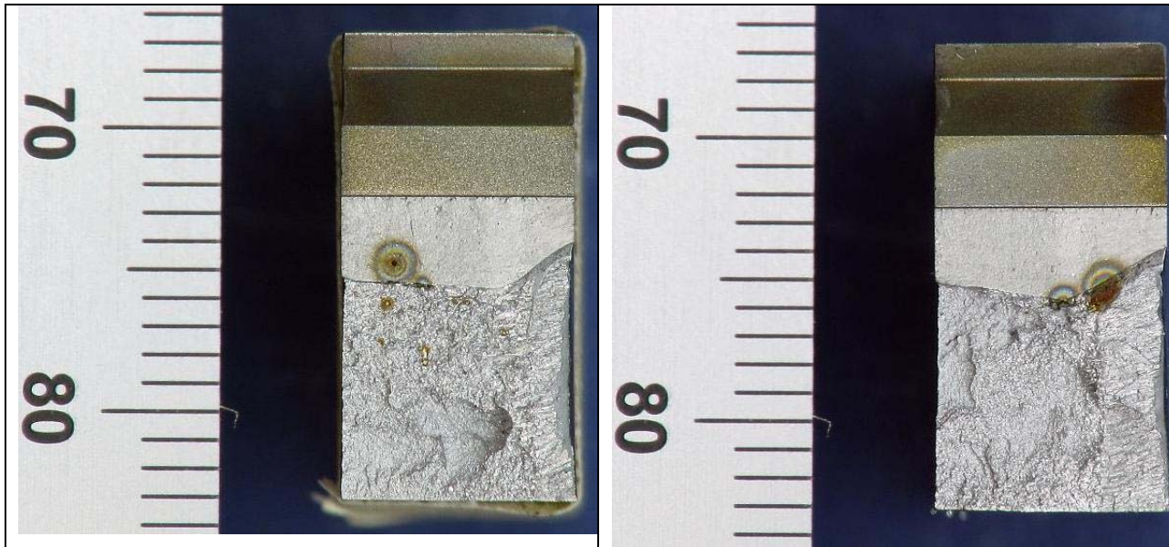
Figure 6.88: Fracture Surface of Specimens 3W (left) and 6W (right) from X80 Pipe Weld
