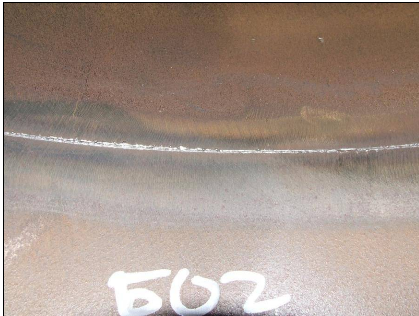
Figure 6.38: Typical Root Bead Profile for X100
