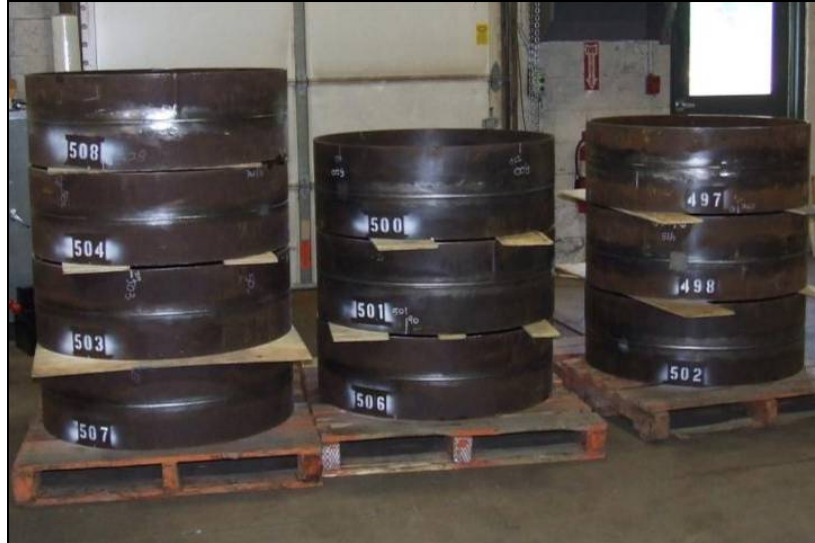
Figure 6.39: Ten Pipe Sections Manufactured for Testing (Pipe Samples 498 to 508)
