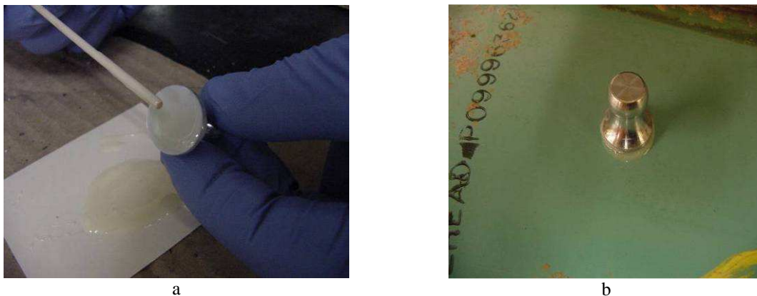
Figure 4. Procedure to adhere the dolly to the pipe surface. a) Uniformly embed the base of the dolly with the epoxy-base adhesive and b) firmly press the dolly on the pipe surface until all the excess is displaced.
