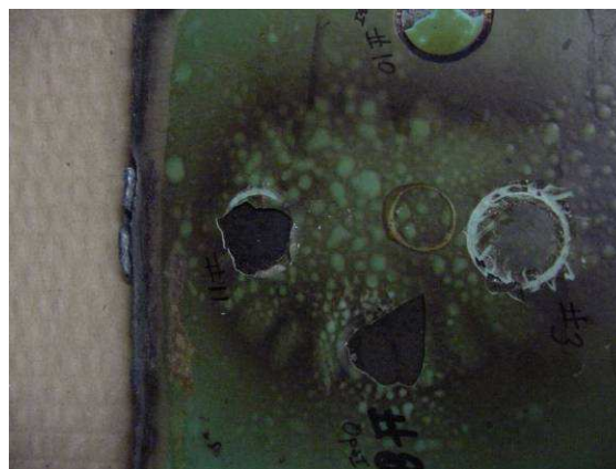
Figure 11. Typical appearance of an intentionally blistered FBE coated pipe.
