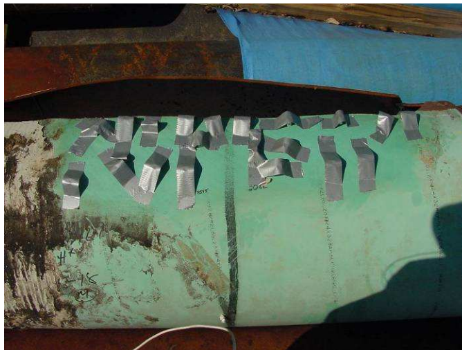
Figure 9. Example of Pull-Off adhesion strength dollies curing on a FBE-coated pipe.
