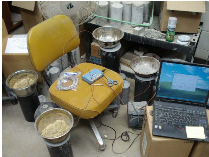
Figure 3.2 Fiber Heat Exchange Thermocouple Recording Setup.
