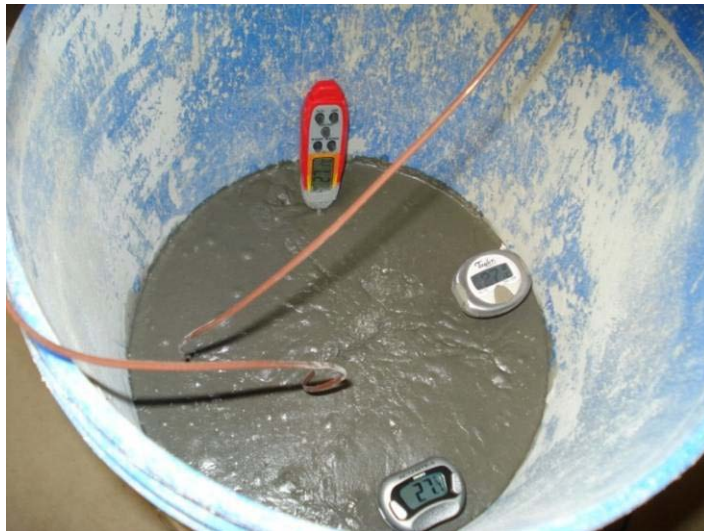
Figure 3.3 Monitoring UHPC Heat Evolution.
