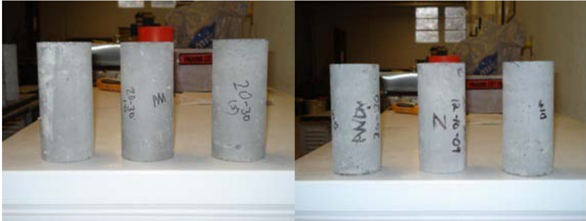
Figure 4.17 Visual Comparison between Pan and Drum Mixed Cylinders.
