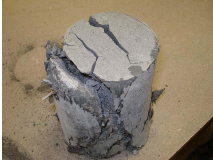
Figure 2.1 Typical UHPC Cylinder Failure.
