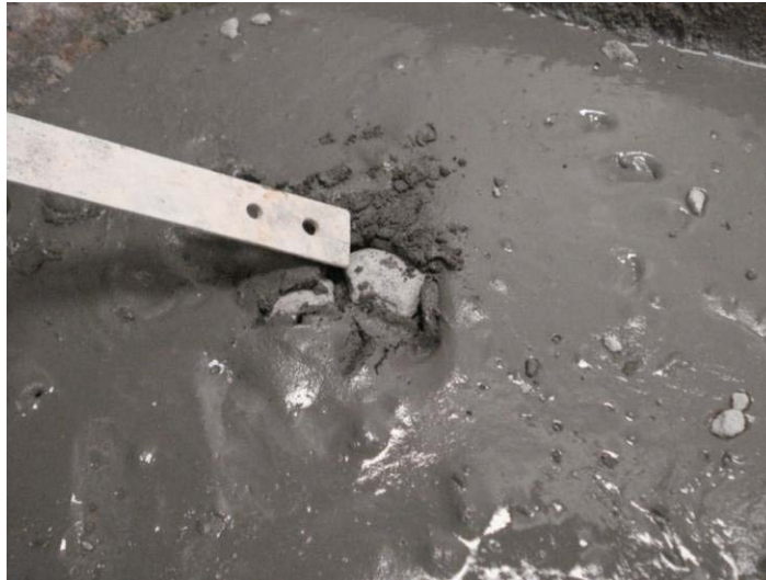
Figure 3.7 Homogeneity Issue from Full Batch Method.
