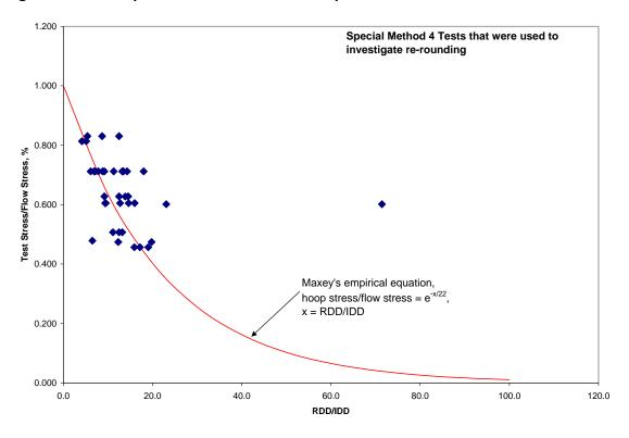
Figure B-20. Special Method-4 Tests that Show Characteristics of Re-rounding
