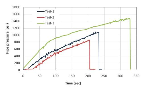
Figure 24 - Pipe pressure during burst tests of the 16-inch pipes in Set-A
