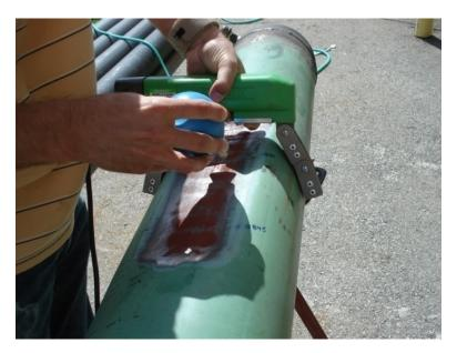
Figure 20 - Inspection of cracks using magnetic particle device
