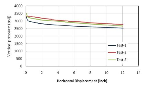
Figure 23 - Applied pressure and horizontal displacement during denting
