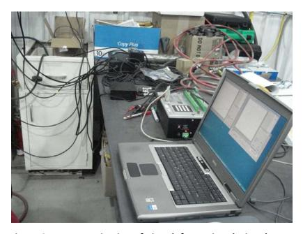
Figure 9 - Data monitoring of pipe deformation during damage application
