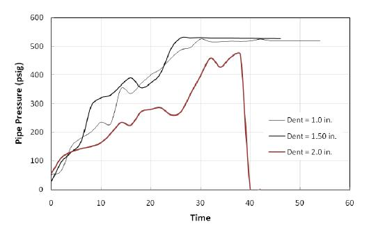
Figure 38 - Results of Test 4 with 90° gouge and various dents
