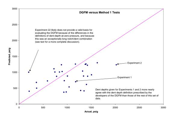
Figure B-7. Comparison between DGFM Predictions and Method-1 Test Data
