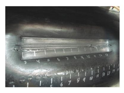
Figure 40 - View of the damage caused by the backhoe tooth application
