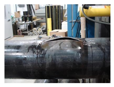
Figure 27 - View of the 16-inch pipe after burst test
