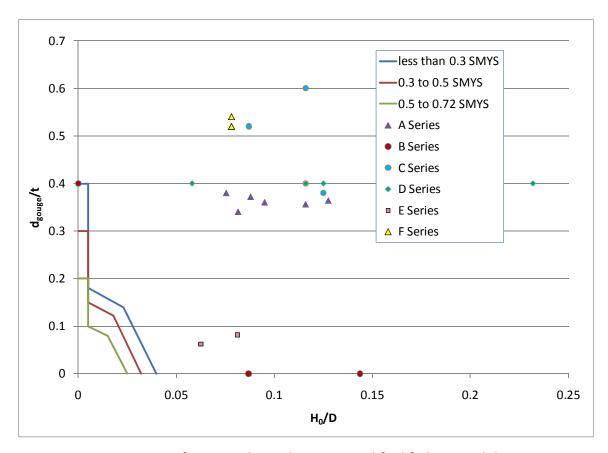
Figure 43 - Comparison of test results with EPRG simplified failure model
