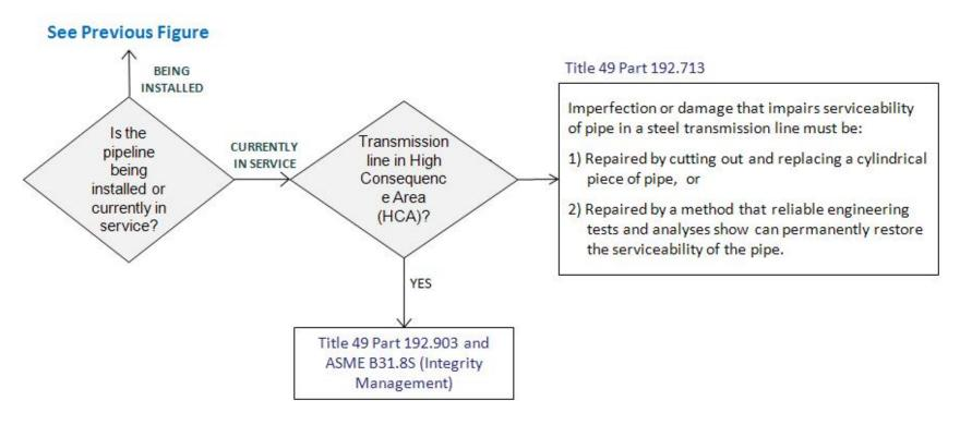
Figure 2 - Repair requirements of damaged pipes in 49 CFR Part 192-Subpart M
