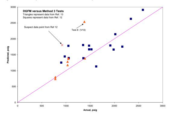
Figure B-10. Comparison between DGFM Predictions Based on Dent Depth at Zero Pressure and Method-3 Test Data
