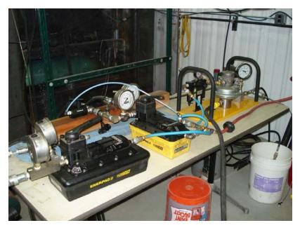
Figure 8 - The hydraulic loading system for dent-gouge applications
