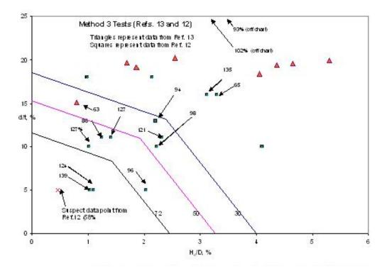
Figure B-14. Characteristic of Dent Formation in Pressurized Pipe
