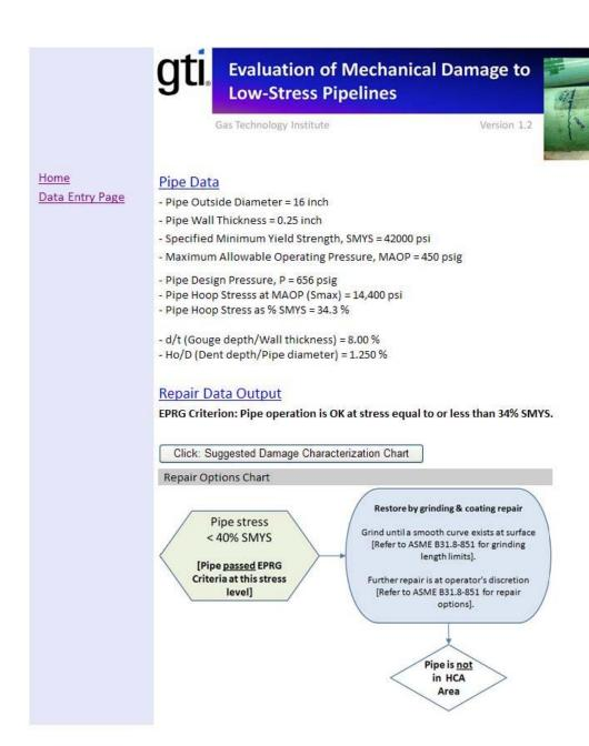
Figure 48 - Output example of damage passing EPRG criteria and not in HCA area
