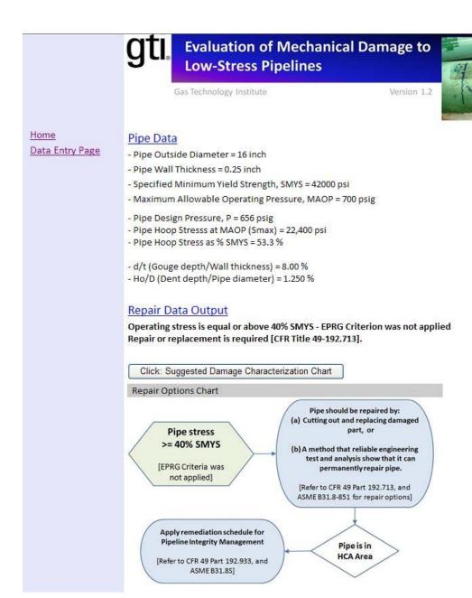
Figure 47 - Output example with operating stress larger than 40% SMYS
