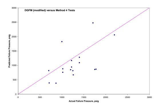
Figure B-17. Comparison between DGFM Predictions Based on Maximum Dent Depth and Method-4 Test Data
