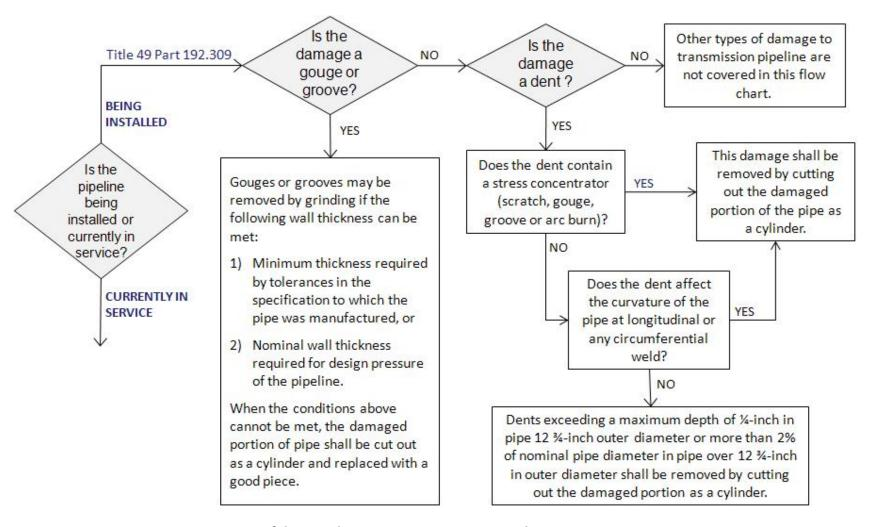
Figure 1 - Construction Requirements of damaged pipes in 49 CFR Part 192-Subpart G
