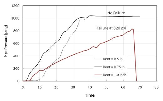
Figure 35 - Results of Test 1 with  $90^\circ$  gouge and various dents
