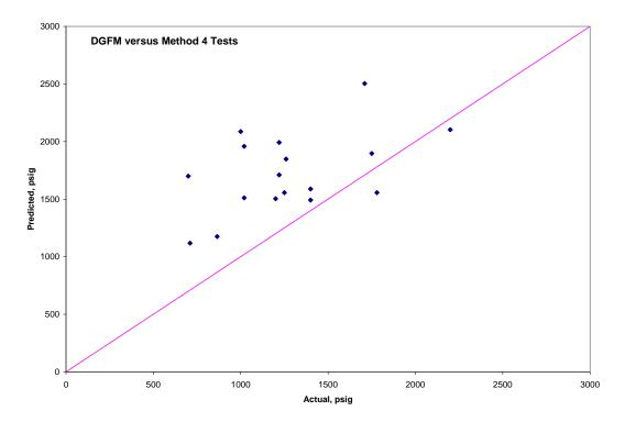
Figure B-16. Comparison between DGFM Predictions Based on Dent Depth at Zero Pressure and Method-4 Test Data
