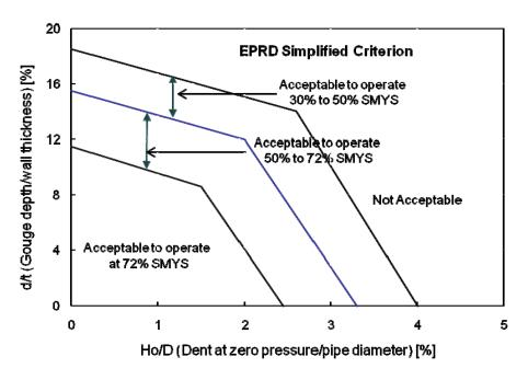
Figure 7 - The EPRG simplified model criterion
