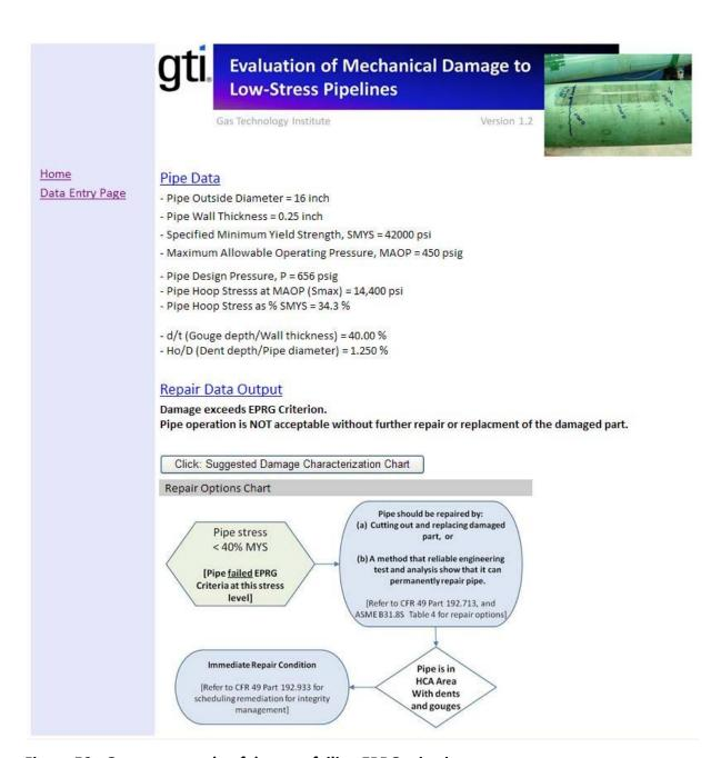
Figure 50 - Output example of damage failing EPRG criteria
