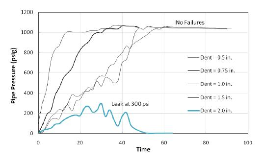
Figure 37 - Results of Test 3 with rounded gouge and various dents
