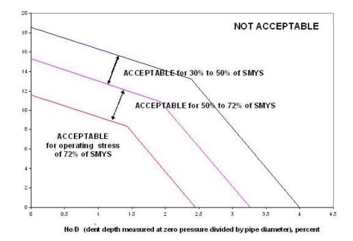
Figure B-2. The EPRG Simplified Model
