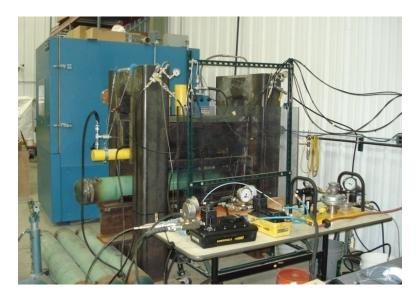
Figure 22 - View of the Large-scale dent-gouge machine
