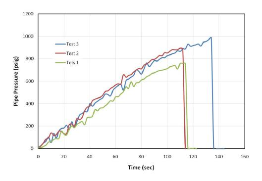
Figure 41 - Results of pressure tests of Set F
