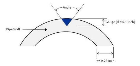
Figure 34 - Testing parameters for test Set-D
