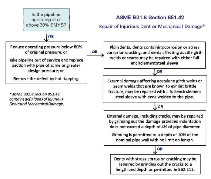
Figure 3 - Repair requirements of damaged pipes in ASME B31.8
