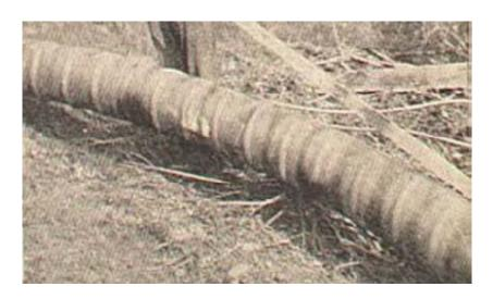
Figure C-1b. Cold formed wrinkle bend from Reference (1)
