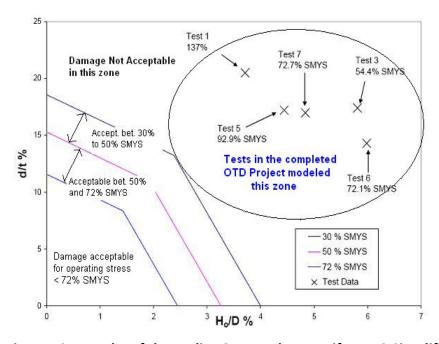
Figure 10 - Results of the earlier OTD study to verify EPRG Simplified Model
