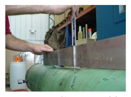
Figure 17 - Measurement of dent at zero pressure (H<sub>o</sub>)
