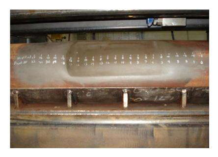
Figure 28 - Indentation of the 8-inch pipe in Set-B
