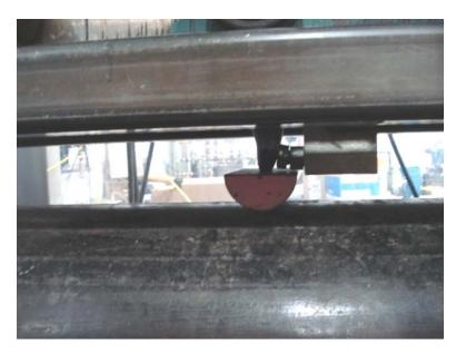
Figure 16 - Application of longitudinal dent along the pipe specimen
