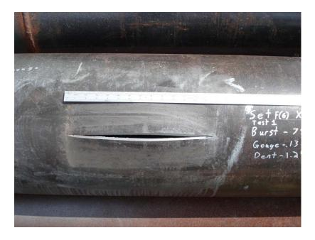
Figure 42 - View of the pipe at the completion of pressure test 3
