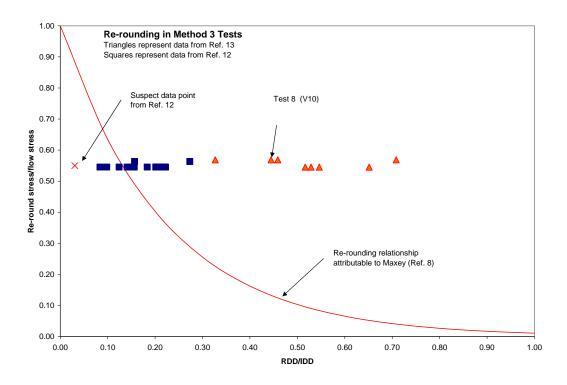
Figure B-15. Re-rounding at Pressure
