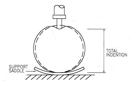
Figure 4 - Typical indentation process associated with methods 1 and 3
