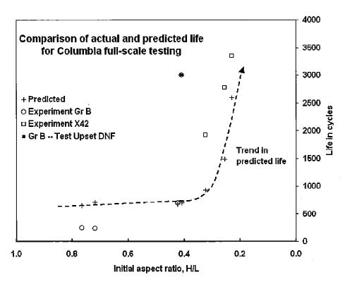
Figure C-3. Columbia Gas wrinkle bend test results
