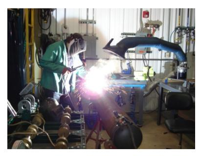
Figure 11 - Welding of pipe caps in preparation of the pipe test sample
