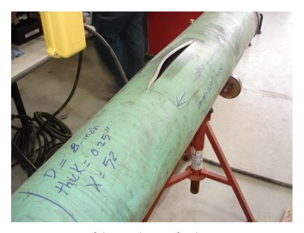
Figure 26 - View of the 8-inch pipe after burst test
