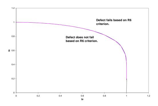
Figure B-1. Failure Assessment Diagram
