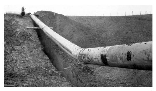
Figure C-1a. Hot formed bend with diamond shaped buckle from Reference (1)
