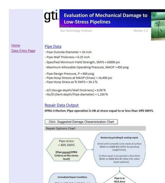
Figure 49 - Output example of damage passing EPRG criteria and in HCA area
