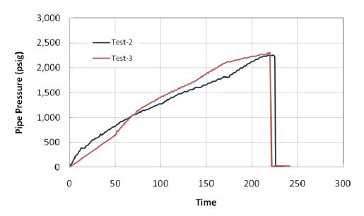
Figure 25 - Pipe pressure during burst tests of the 8-inch pipes in Set-A
