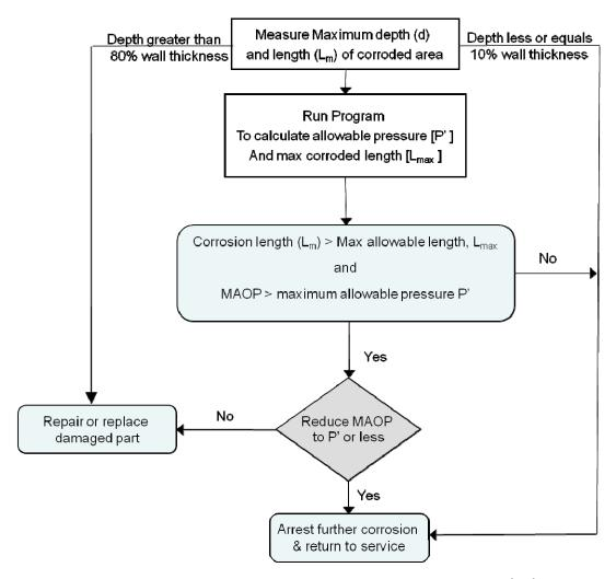
Figure 51 - Procedure for corrosion repair criteria, after ASME B31G (14)
