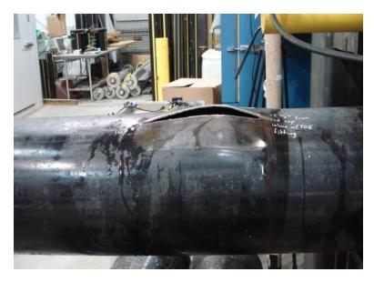
Figure 21 - View of pipe at the completion of the burst test
