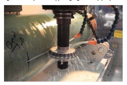
Figure 14 - Application of controlled gouge on the pipe specimen
