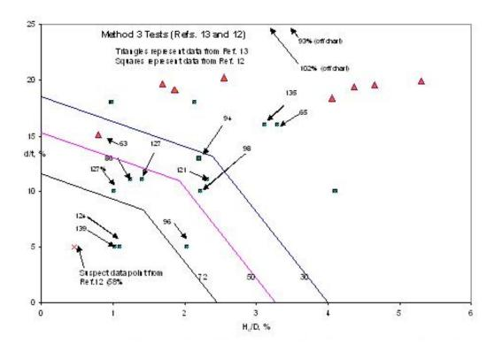
Figure B-13. Comparison between DGFM Simplified Criterion and Method-3 Test Data
