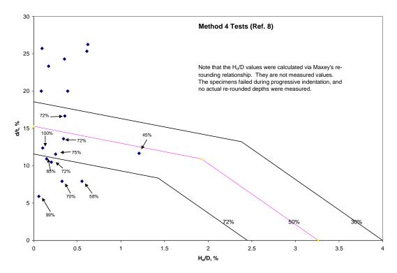
Figure B-19. Comparison between DGFM Simplified Criterion and Method-4 Tests
