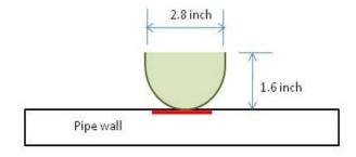
Figure 15 - Schematic of the rounded disc for dent application
