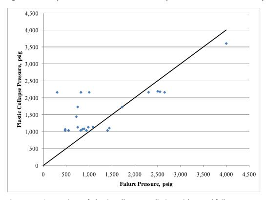
Figure 45 - Comparison of plastic collapse prediction with actual failure pressure
