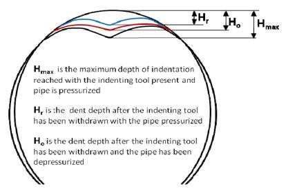
Figure 18 - Measurements of dents in the pipe during and after loading
