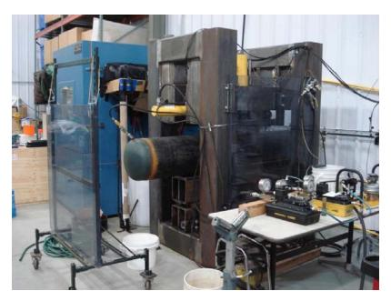
Figure 6 - The large-scale dent-gouge machine with a 16-inch diameter pipe
