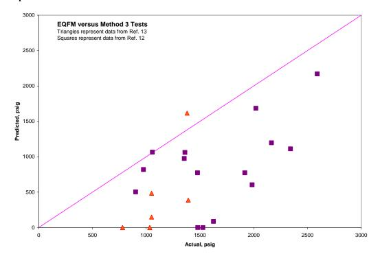
Figure B-12. Comparison between EQFM Predictions and Method-3 Test Data
