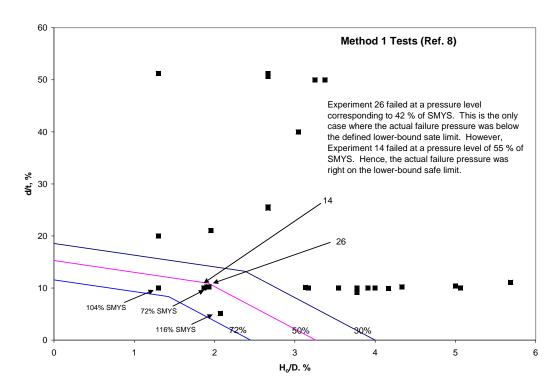
Figure B-9. Comparison between DGFM Simplified Criterion and Method-1 Test Data
