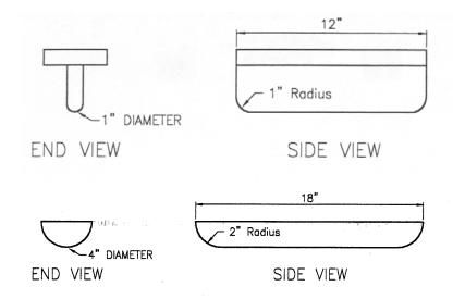
Figure B-4. Typical Indenters Associated with Methods 1 and.3
