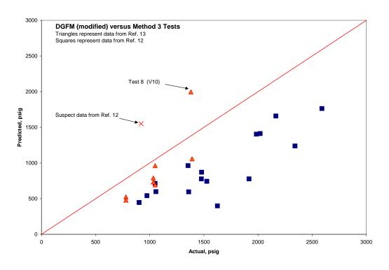
Figure B-11. Comparison between DGFM Predictions Based on Maximum Dent Depth and Method-3 Test
