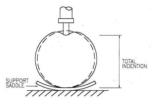
Figure B-3. Typical Indentation Process Associated with Methods 1 and 3
