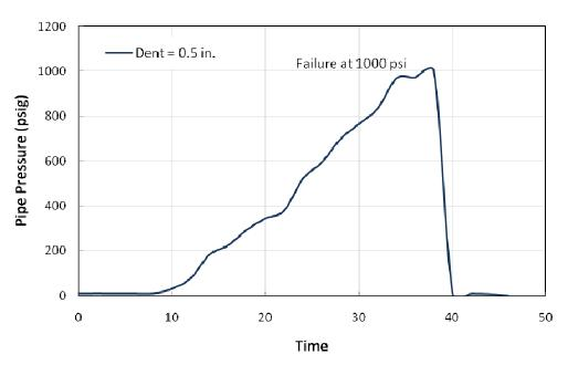
Figure 36 - Results of Test 2 with 45° gouge angle
