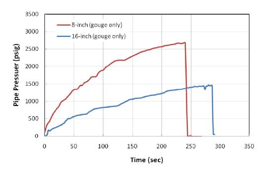
Figure 30 - Pressure tests on the gouged pipes in Set-B
