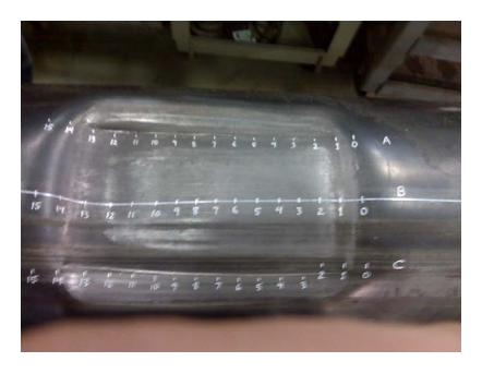
Figure 29 - Indentation of the 16-inch pipe in Set-B
