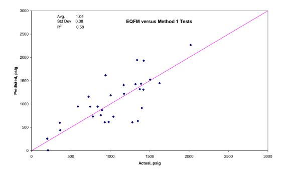
Figure B-8. Comparison between EQFM Predictions and Method-1 Test Data
