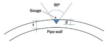
Figure 13 - Shape of the applied gouge on the pipe specimen
