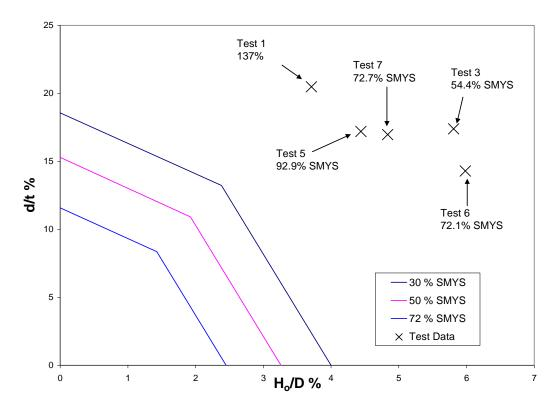
Figure B-22. EPRG simplified model compared to GTI's test data
