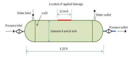
Figure 12 - Schematic of the pipe test specimen
