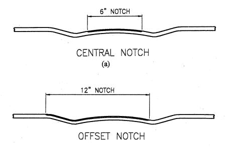
Figure B-6. Typical Locations of Notches Associated with Methods 1 and 3
