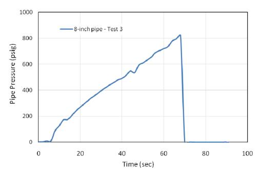
Figure 31 - Pressure tests No. 3 on the 8-inch pipe in Set-C
