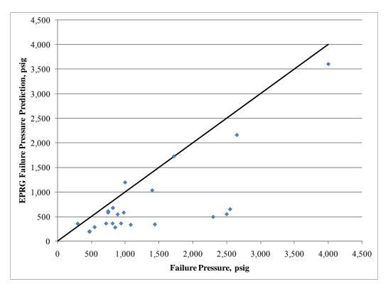
Figure 44 - Comparison of advanced EPRG failure prediction with actual failure pressure
