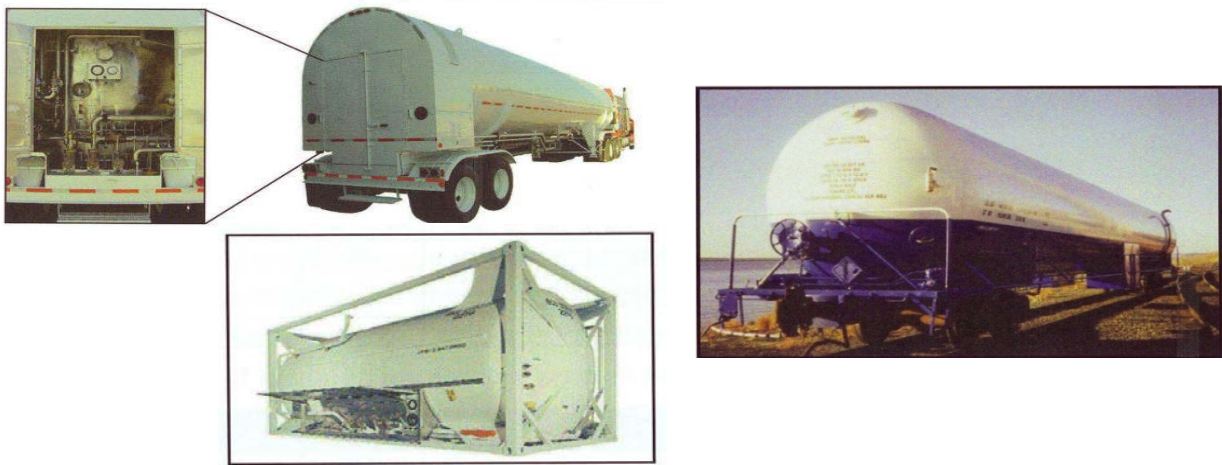
Figure 4. Chart Industries LNG Highway Semi-Trailer, 20-Foot Intermodal LNG ISO Container, and R-602 Bulk LNG Tank Car for Rail Transport
