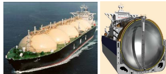
Figure 2. Moss Ship and Tank Schematic
