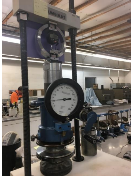
Figure 17. R-value testing equipment.
