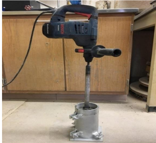
Figure 9. Vibratory compactor and sample mold.
