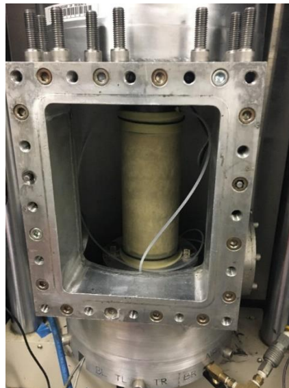
Figure 12. Sample inside the triaxial chamber.
