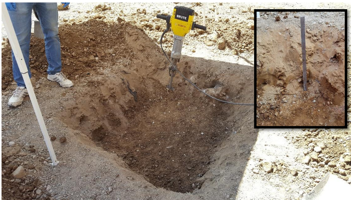
Figure 7. Sampling of SEM soil at a depth of two feet.
