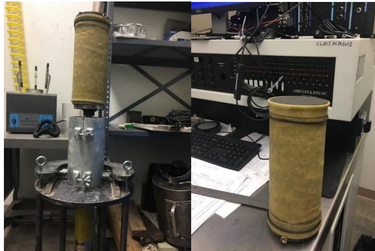
Figure 11. Compacted sample with membrane, porous stones, and O-rings.
