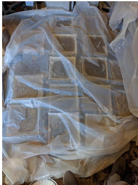
Figure 4-5 Specimens with saltwater solution covered with plastic covers
