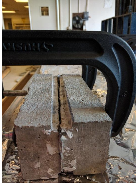
Figure 4-17 Specimens clamped to form the required width
