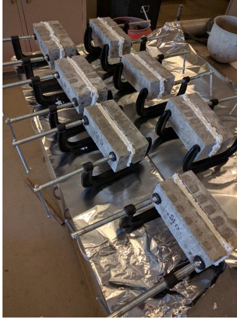
Figure 4-18 Specimens after being sealed with silicone caulk
