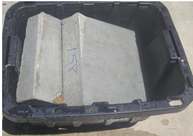
Figure 4-14 Immersion of specimens in a plastic bucket filled with water. Specimens were removed after 7 days, rinsed, towed and weighted ( W_7 ). The weight gained was calculated using Equation 4-3
