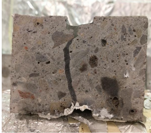
Figure 4-19 Cross section of a specimen filled with crack sealer
