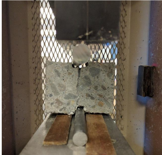
Figure 4-20 Setup used to test the bond strength of the crack sealer specimens The load rate used was approximately equal to that stated by the ASTM C 496. The loading rate in the specification is 100 to 200 psi/min. The loading rate used in the
