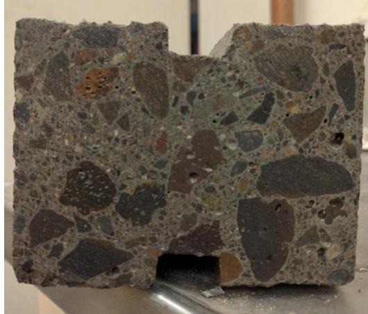
Figure 4-15 Notches in the upper and lower surface of the specimens
