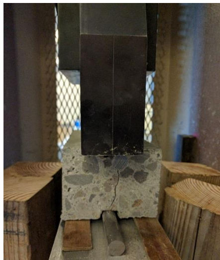
Figure 4-16 Test setup used for cracking the specimens
