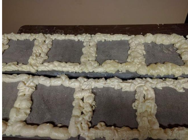
Figure 4-4 Expanded foam around the edge of the specimen
