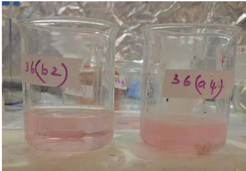
Figure 4-7 Samples after being acidic with nitric acid and methyl orange indicator Three alternate methods are specified by AASHTO T260 for the analysis of the given results of the electrode. The method used in this research was Potentiometric Titration.
