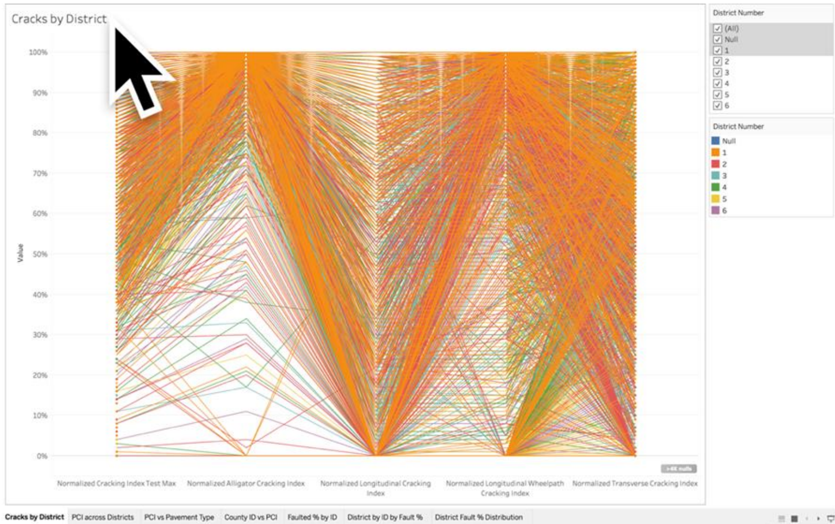
Figure 7. Initial view of selected cracking indices by road segment, district, and year
