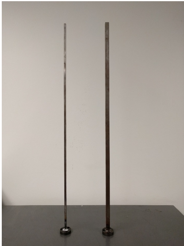
Figure 2-11. Load-carrying square steel spine. (Steel spine on the left is 3/16-inch, and spine on the right is 3/8-inch.)
