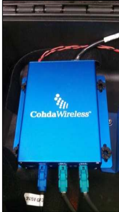
Figure 19.4 Example of an OBU, a Cohda Wireless MK5 DSRC unit
