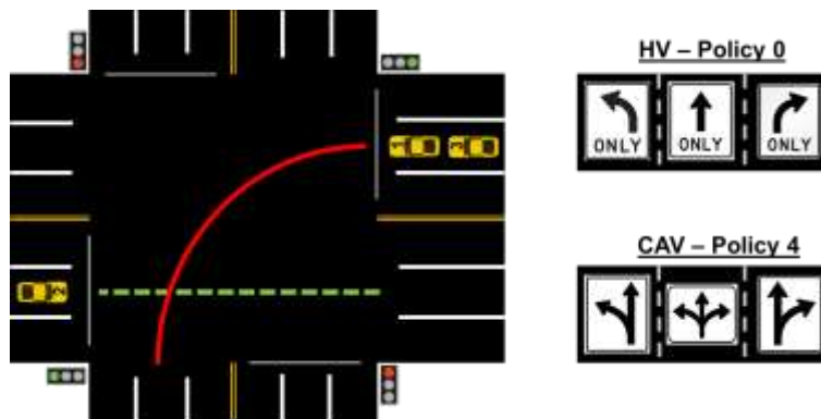
Figure 4.7 An example where a combination of strict turning policy for HVs and liberal policy CAVs is counterproductive [vehicle 1 (CAV) blocks vehicle 3 (HV) from passing the intersection]
