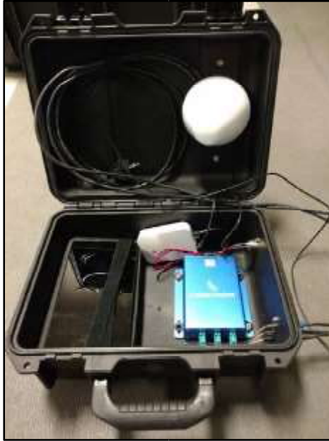
Figure 19.2 SwRI-developed PODs with all of the components necessary to turn any vehicle into a DSRC-enabled CV
