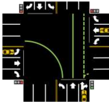
A green signal is assigned to all northbound lanes while all other lanes are assigned a red signal. Green trajectories marked with solid or dashed green lines across the intersection. Active green trajectories marked only by dashed green lines.
