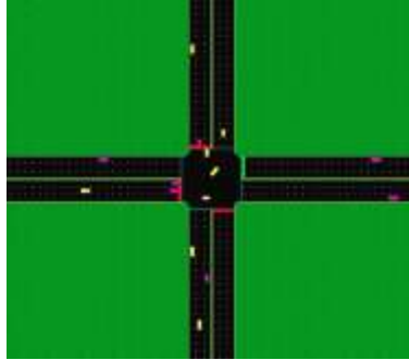
HVs (in purple) may not enter the intersection on a red signal. CAVs (in yellow) may enter the intersection on a red signal when following an approved reservation.
