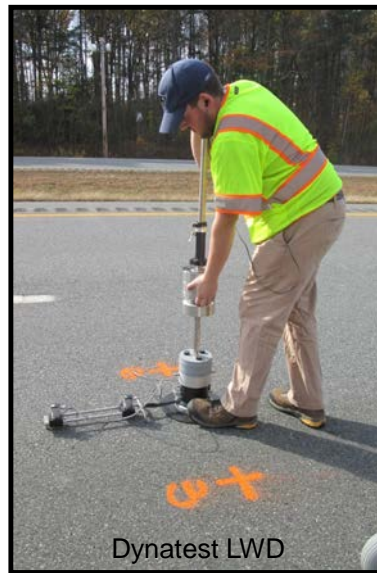
Figure 1. Operation of Dynatest LWD portable impulse loading device during field testing.
