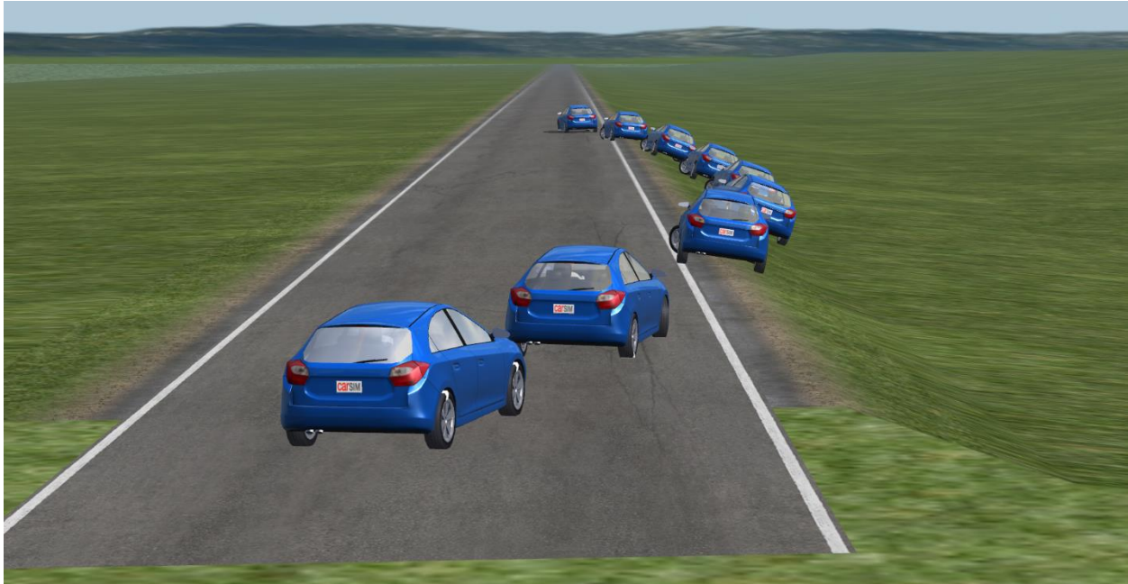
Figure 41. Class C hatchback departing at a 15° encroachment angle at a speed of 110 km/h.
