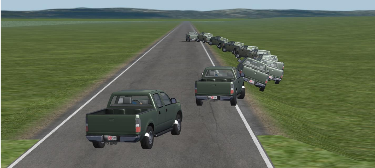
Figure 29. Pickup truck encroaching at a 15° angle at a speed of 110 km/h (CarSim).
