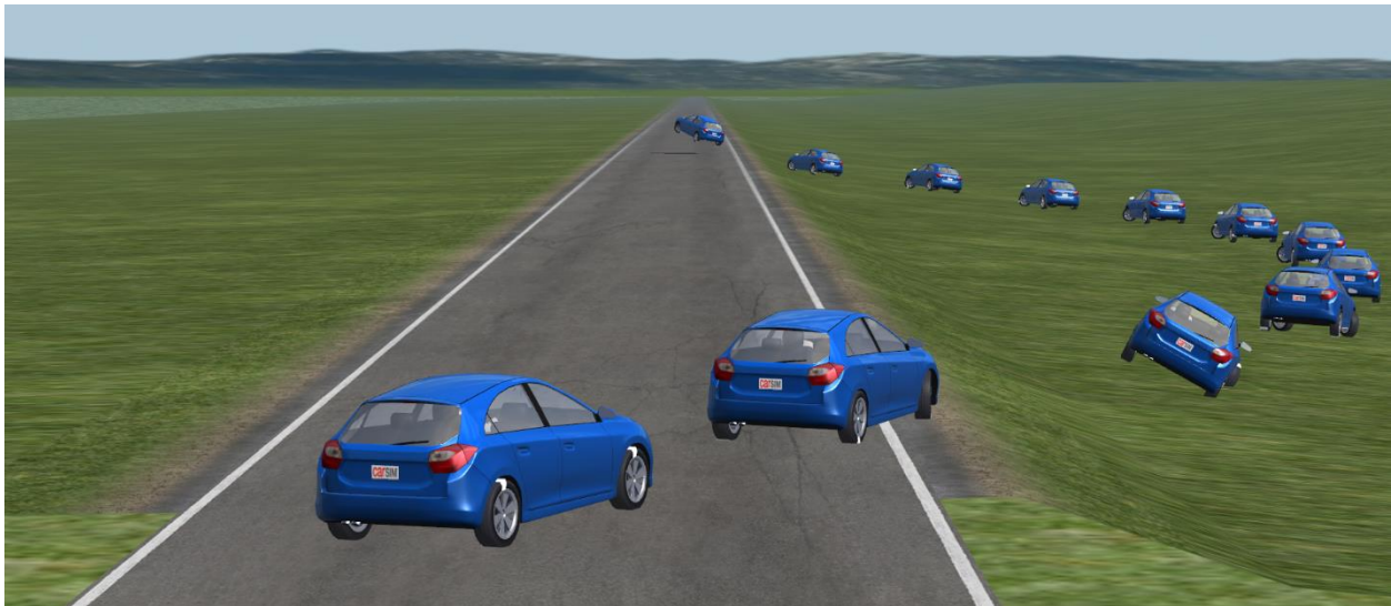
Figure 47. Class C hatchback encroaching at a 25^\circ angle at a speed of 120 km/h.
