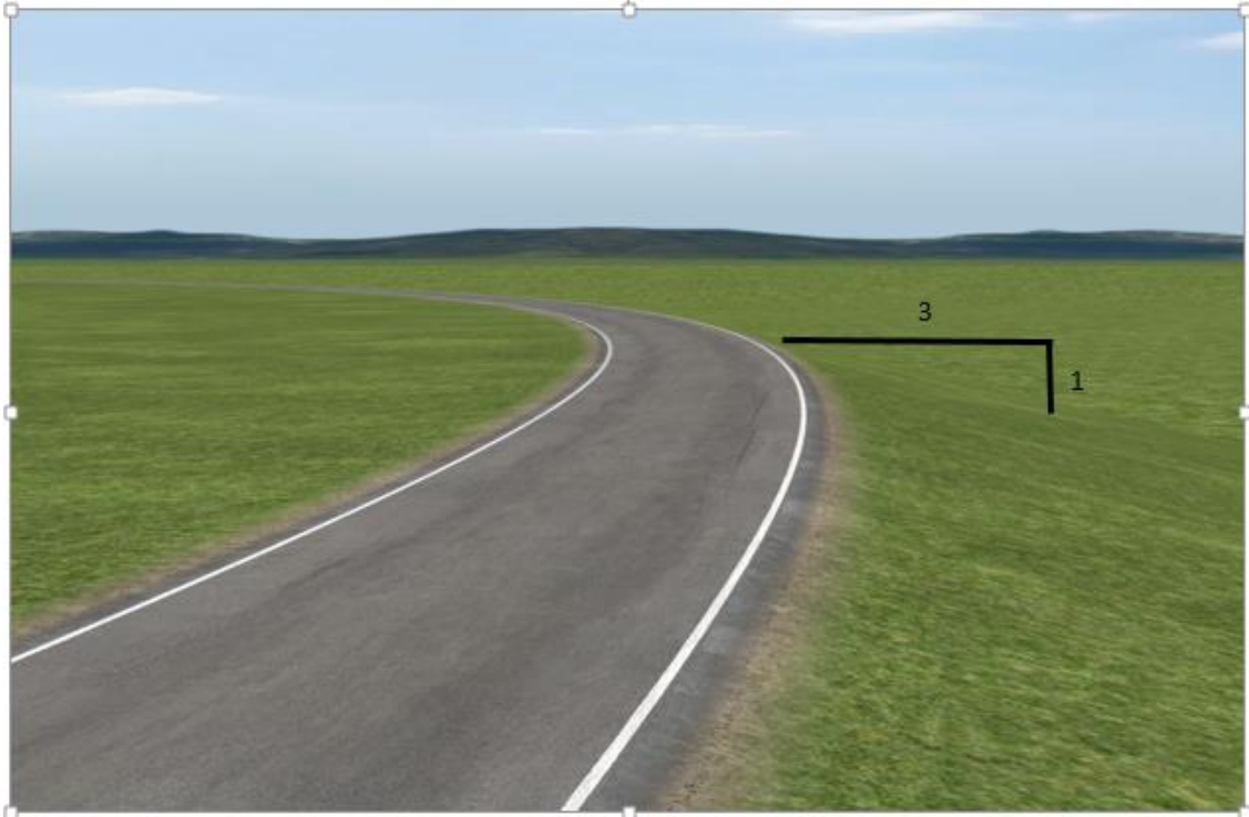
Figure 11. 621.79 m radius road with a 3:1 side-slope.
