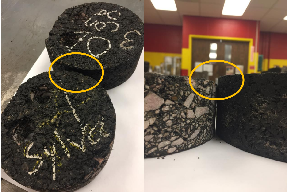
Figure 6-11 Difference in lab samples and field cores thicknesses
