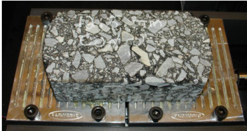
Figure 8: Specimen Setup in Overlay Test (OT) Device
