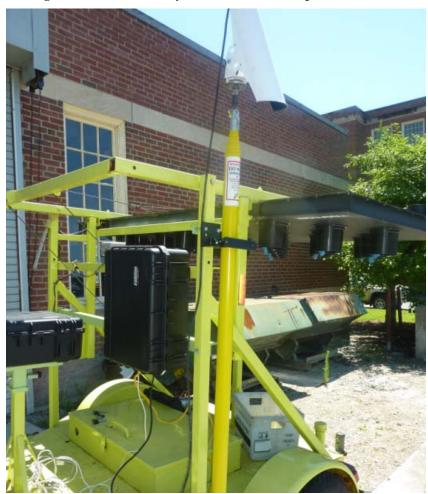
Figure 10: Solo Terra system mounted on a portable trailer
