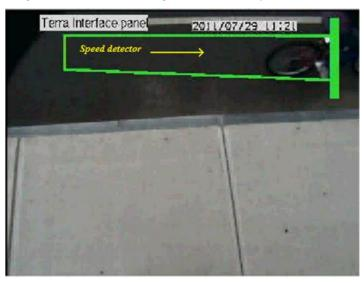
Figure 9: Detector configuration for bicyclist detection
