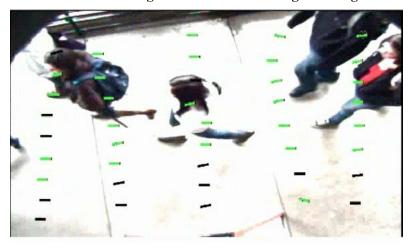
Figure 11: Detectors remaining "ON" due to blooming resulting in undercounts
