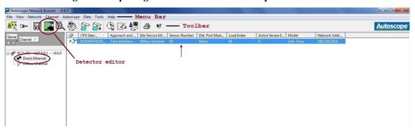
Figure 31: Opening detector editor in Autoscope network browser
