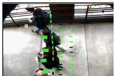
Figure 13: Detector configuration with non-uniform spacing
