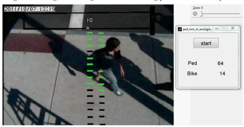
Figure 15: Integrated configuration for detecting pedestrians and bicyclists
