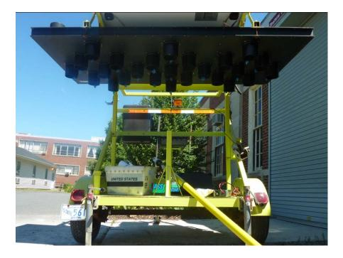
2. Open the black interface panel case (the one standing vertically) and pull out the two cables – the black camera cable, and the yellow interface panel power cord, through the hole at the bottom of the case.
