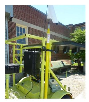
9. Once the mast is secured, draw out the second layer of the mast upwards to the point where it is locked with the red button. The first layer is not chosen to ensure that the pole does not sway with wind once the mast is drawn out at a higher level. Using the second layer improves the thickness of the mast, and thus its stability.
