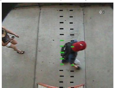
Figure 4: Two columns of uniformly distributed presence detectors
