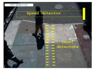
Figure 25: Autoscope video output
