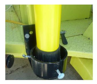
8. Secure the higher end of the mast by fixing the bracket around it. While affixing the bracket tightly, make sure that the camera is facing the road, perpendicular to the edge of the trailer.
