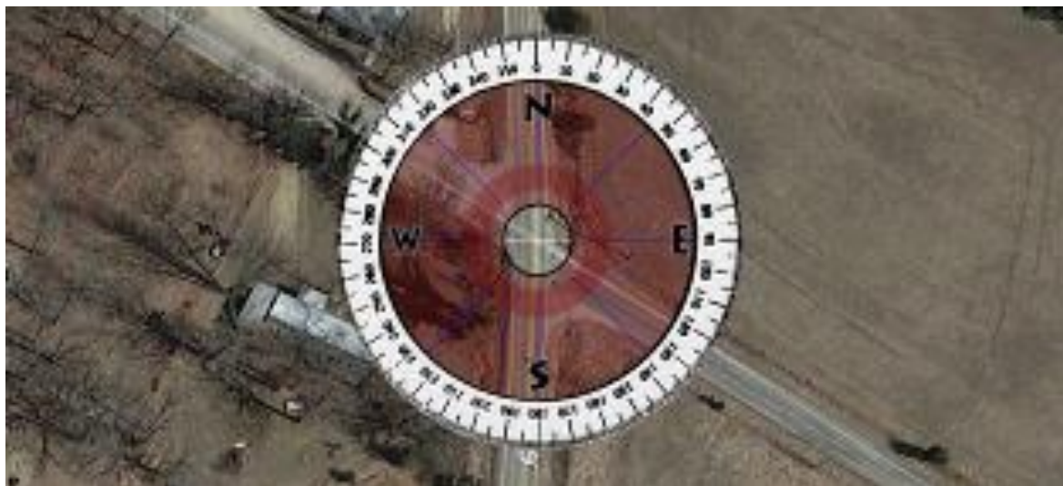
Figure 9.8 Skew angle measurement for a 4-leg stop-controlled intersection (Google 2016)
