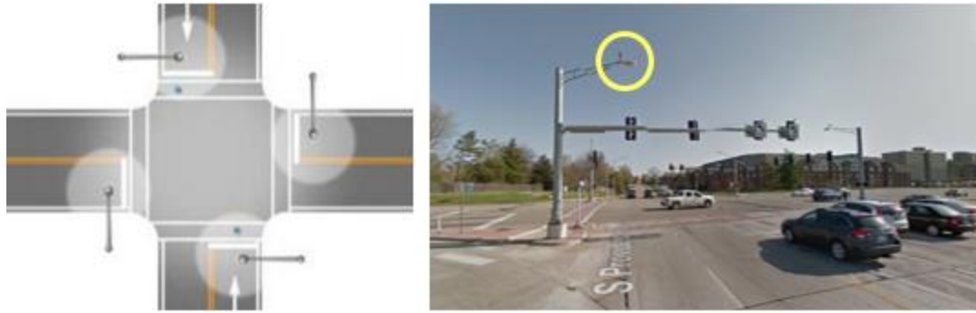
(a) Common intersection lighting layout (b) Street view of intersection with lighting
