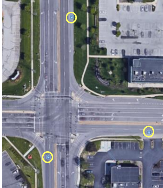
Figure 8.11 Intersection bus stops (Google 2016)
