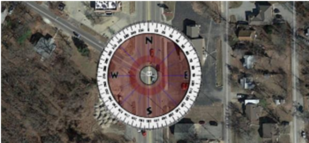
Figure 9.7 Skew angle measurement for a 3-leg stop-controlled intersection (Google 2016)
