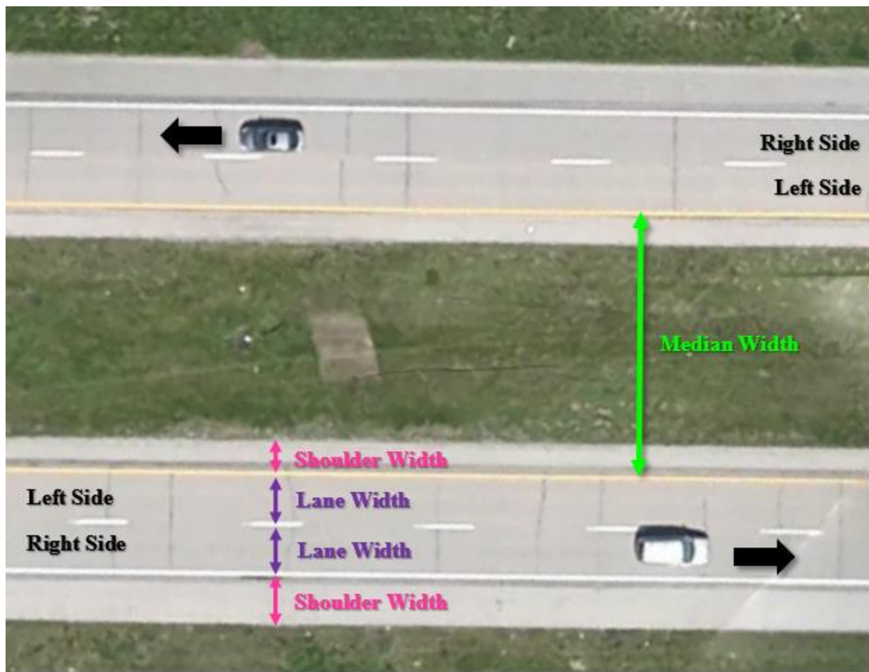
Figure 5.1 Lane, shoulder, and median width illustration
