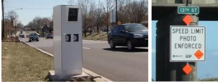
Figure 6.12. Automated speed enforcement camera (Google 2016)
