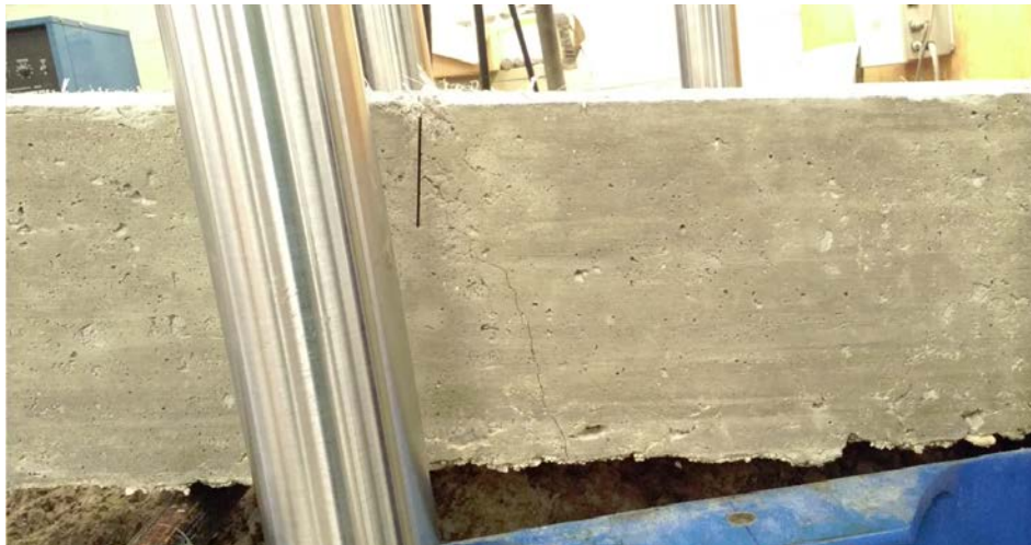
Figure M-42. Crack patterns with respect to dowel location (Specimen 5)
