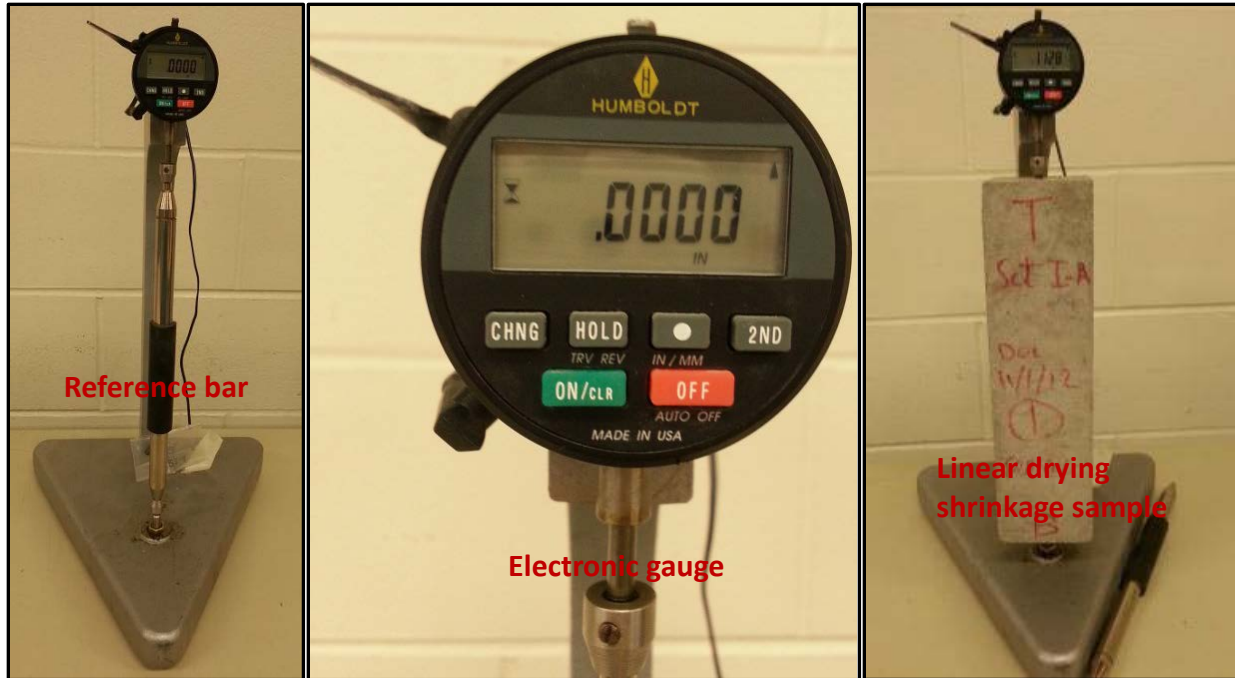
Figure 5-9. Linear drying shrinkage-test configuration.
