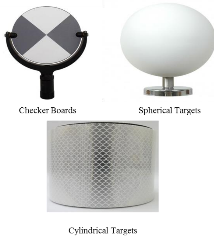
Figure 6. Commonly used targets for terrestrial laser scanning
