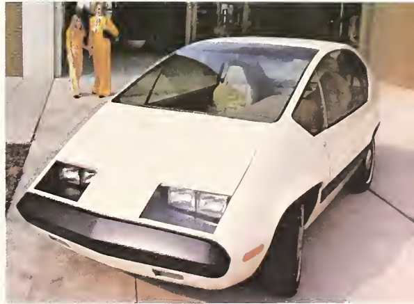
A full view of the Copper Association's prototype car. The front wheel drive car accelerates from 0-30 mph in 11.8 seconds.
