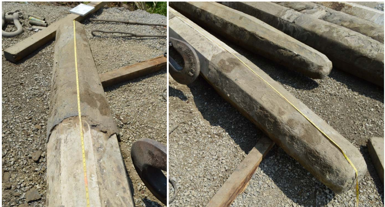
Figure 37: Photographs of tips of exhumed precast piles.
