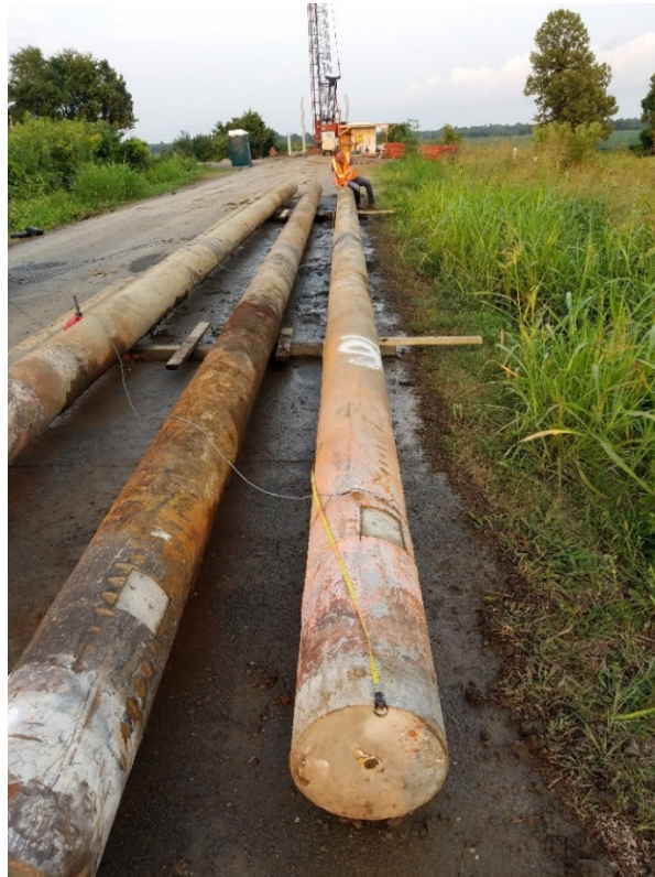
Figure 22: Experimental setup for measuring wave velocities in exhumed CIP piles at Route WW.
