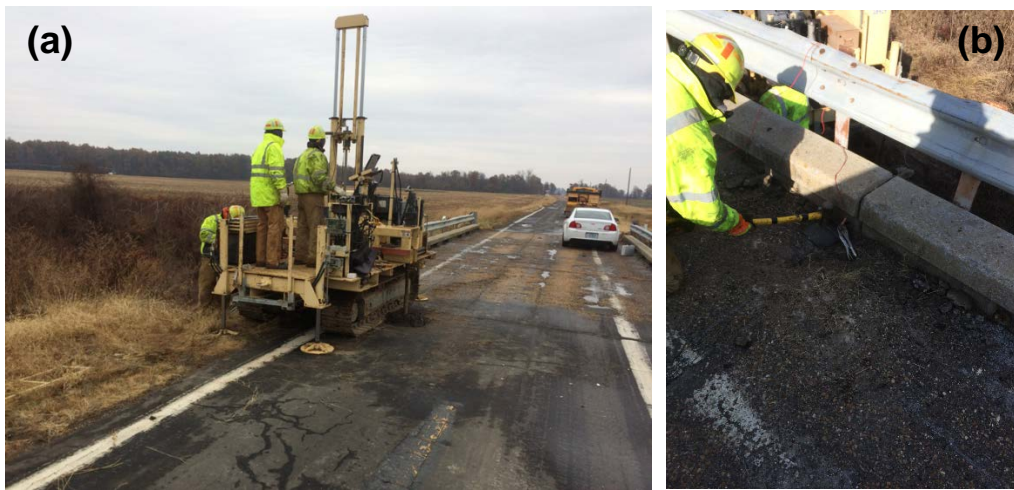
Figure 16: PS testing at the Route U bridge site: (a) SCPT rig and (b) impact hammer.
