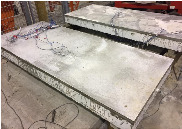
Figure 6-10 Composite slabs with sensors at three different locations
