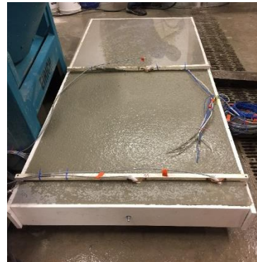
Figure 6-8 Preparation and casting of UHPC overlay
