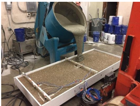
Figure 6-8 Preparation and casting of UHPC overlay
