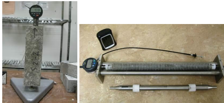
Figure 3.5: Drying shrinkage (left) and autogenous shrinkage (right)
