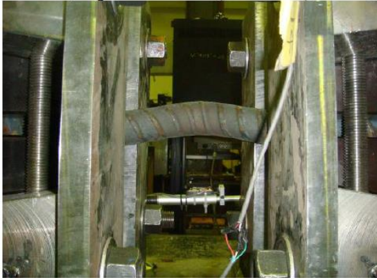
(b) Test apparatus with a buckled bar
