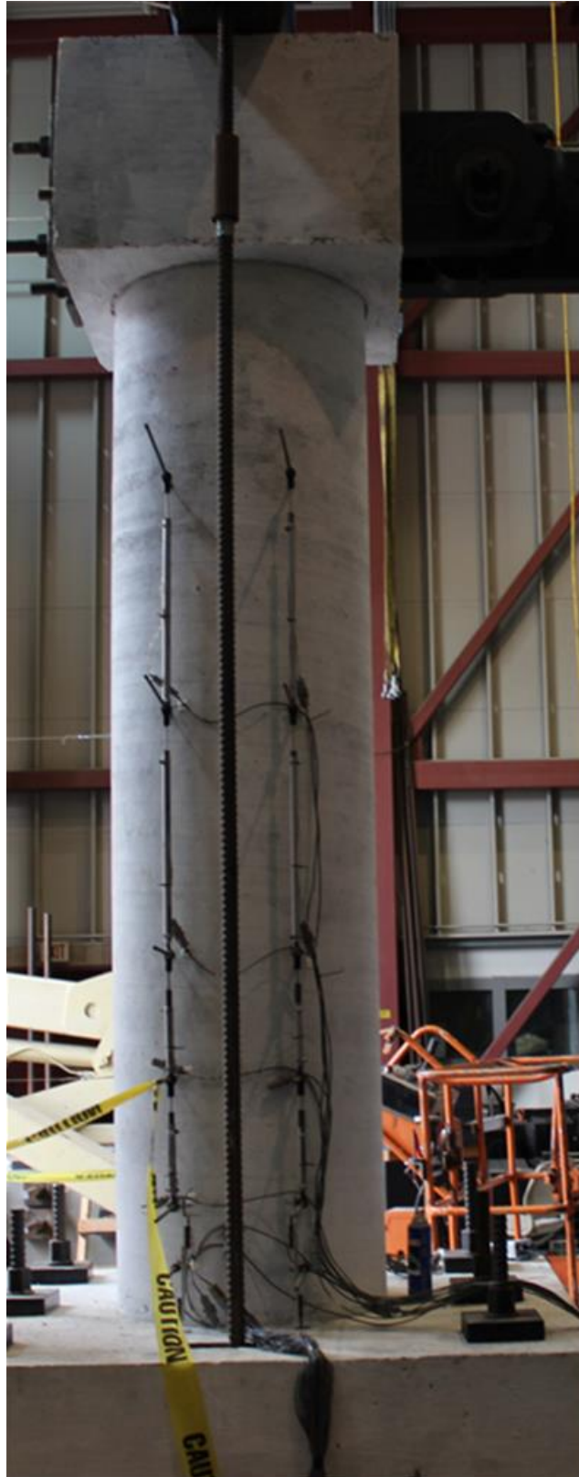
Figure 2.13 - Picture of displacement transducers mounted on west face of Specimen #1
