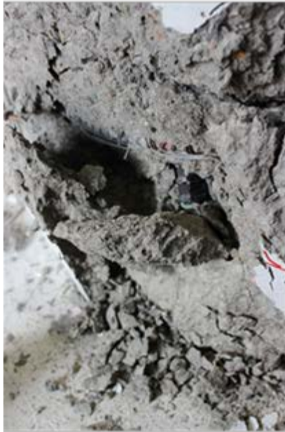
Figure 3.7 – Specimen #1 at 6% drift
