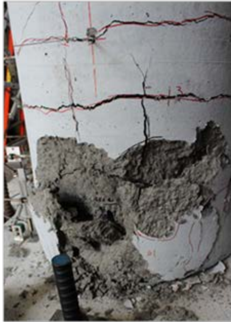
Figure 3.7 – Specimen #1 at 6% drift
