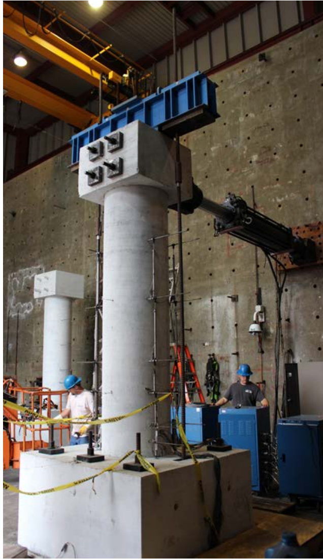
Figure 2.9 Picture of Specimen #1 test setup
