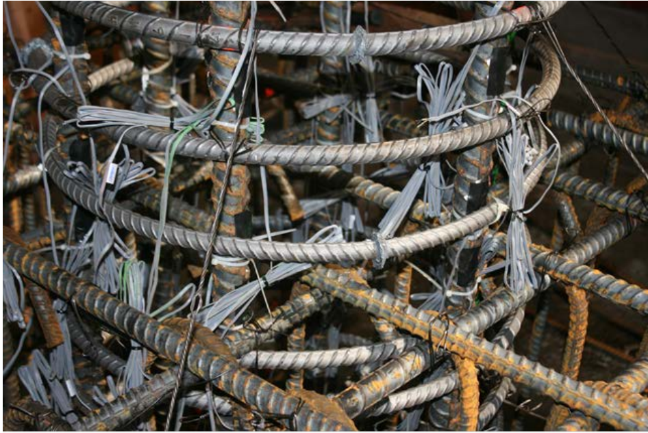
Figure 2.17 – Picture of strain gages on reinforcing bars of Specimen #1
