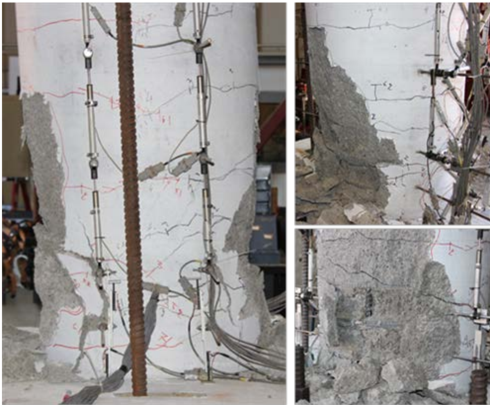
Figure 3.20 - Specimen #2 at 6% drift
