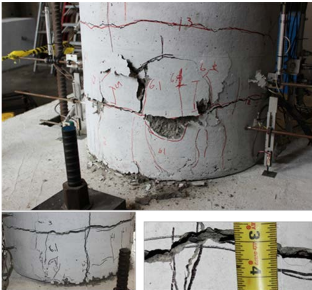
Figure 3.6 - Specimen #1 at 3% drift
