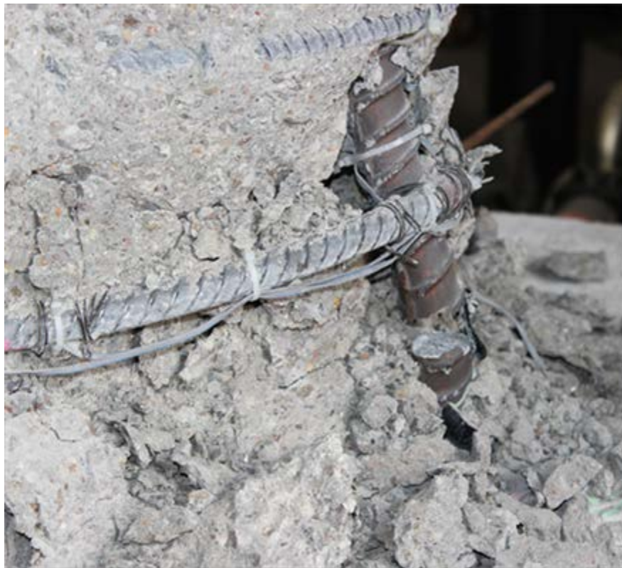
Figure 3.11 – Fractured bar #4 at north face of Specimen #1 during 2 nd cycle of -10% drift
