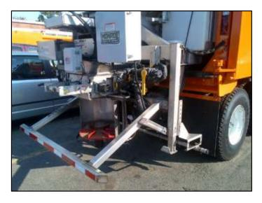
Figure 17: Salt-Slurry Generator
