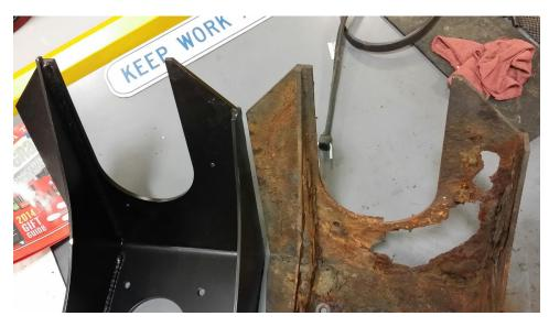
Figure 6.11. New and Corroded Muffler Support Brackets (Photo from [126])
