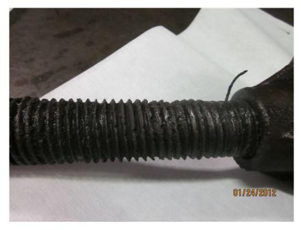
FIGURE 6.13. CORRODED LANDING LEG SCREW (PHOTO FROM [126])
