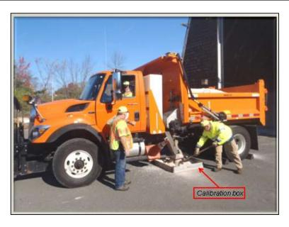
Figure 13: Spreader calibration
