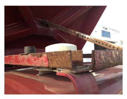
Figure 6.12. Corroded Air Shield Support Frame (Photo from [126])
