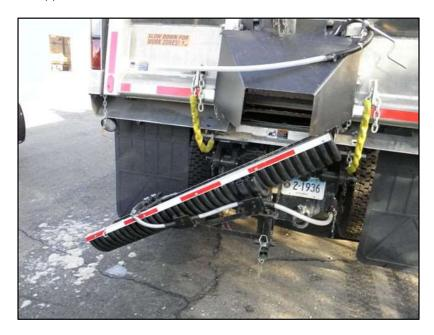
Figure 16: The Connecticut Rear Truck-Mounted Discharge Chute
