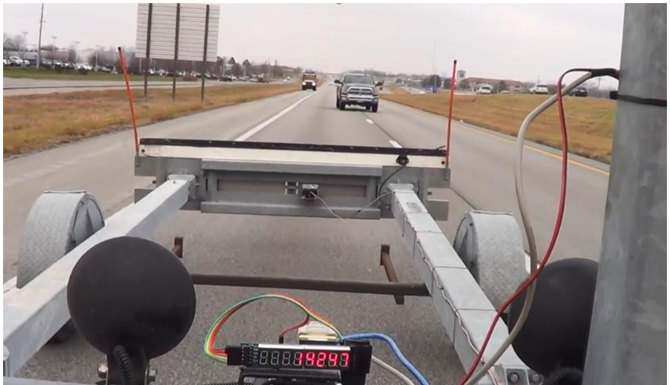
Figure 4.1.3 Example of LiDAR capturing distance from vehicle to rear advance TMA
