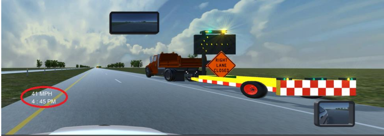
Figure 2.3.5 MOE 5 example: speed when passing shoulder TMA (mph)
