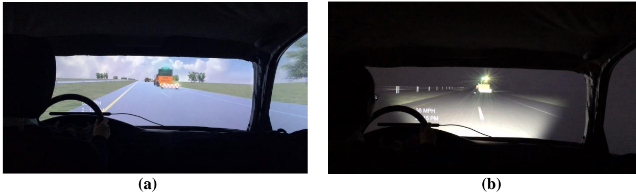
Figure 2.1.1 TMA experiment using ZouSim (a) Daytime example: green only TMA (b) Nighttime example: green/amber TMA
