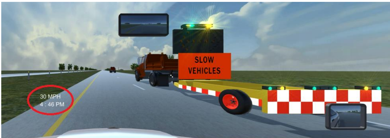
Figure 2.3.6 MOE 6 example: speed when passing rear advance TMA (mph)
