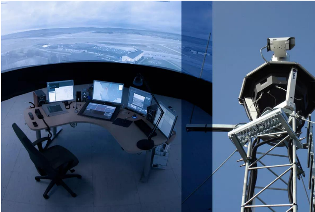
Figure 5. Example of Remote ATC Tower (SAAB). 37
