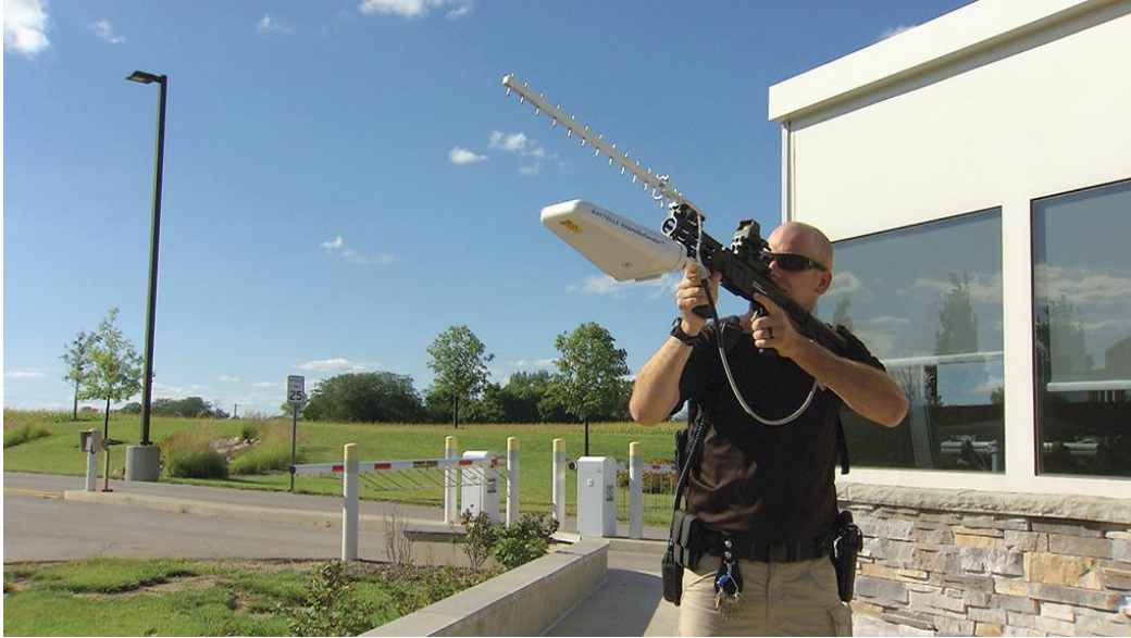
Figure 4. Example of a Hand-Held Counter Drone Technology (Battelle). 32
