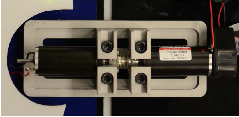
Figure 4.4: Actively coupled dynamometer
