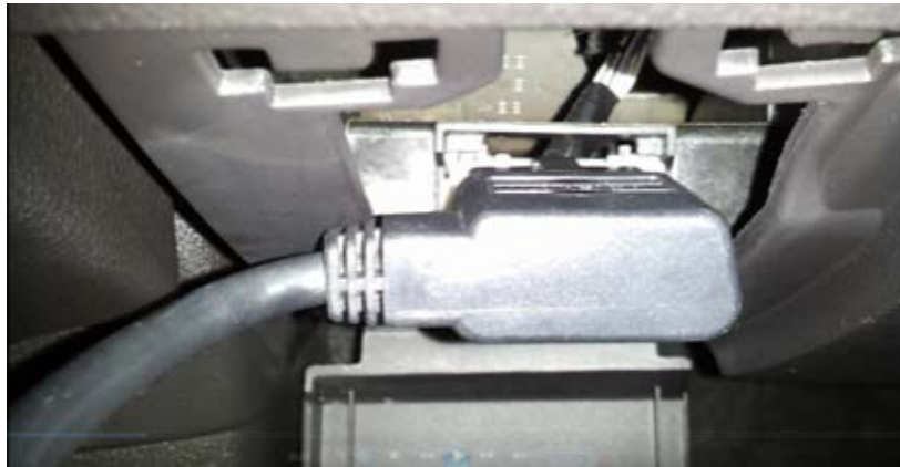
Figure 5.1: PCAN USB connected to the OBD port
