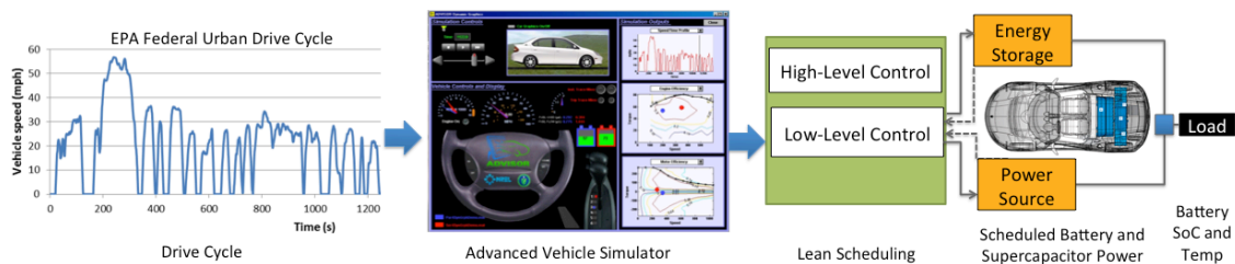
Figure 2.4: The Protodrive battery-super capacitor energy management system
