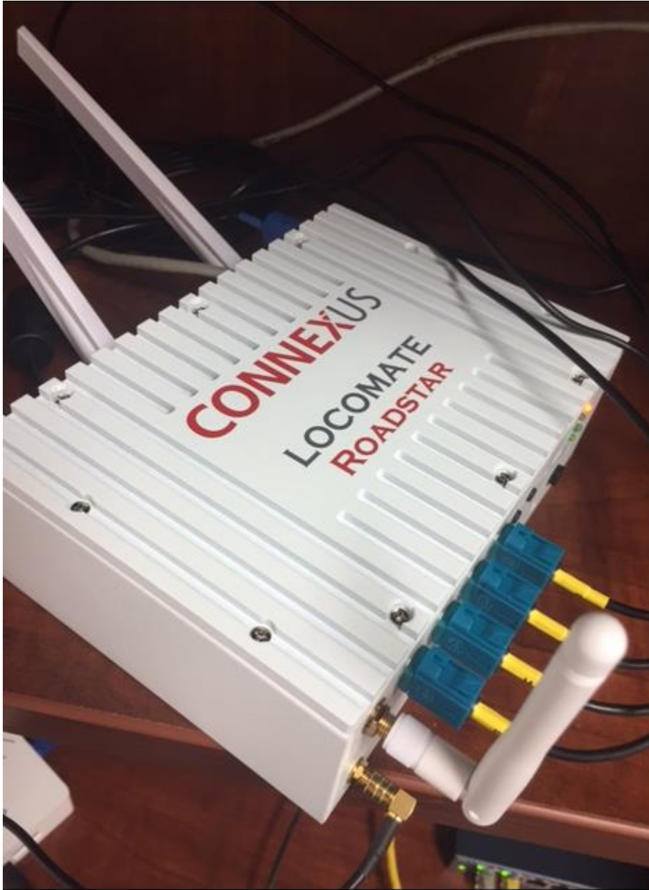
Figure 3-83. Lear Locomate Roadstar Premium OBU (Source WYDOT)
