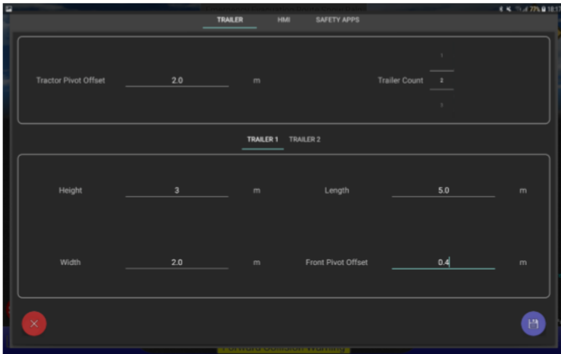
Figure 3-121. HMI Trailer Configuration Interface. (Source: Lear)
