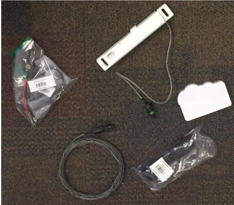
Figure 3-88. Weather Cloud Environmental Sensor hardware (Source WYDOT)
