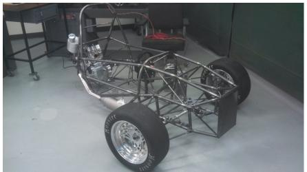
Completed chassis with completed front suspension, steering, and engine installed. Through the design and manufacturing process our team discovered which team members processed certain gifts and skills. Moving forward utilizing each team member's specialties will help propel our project forward.
