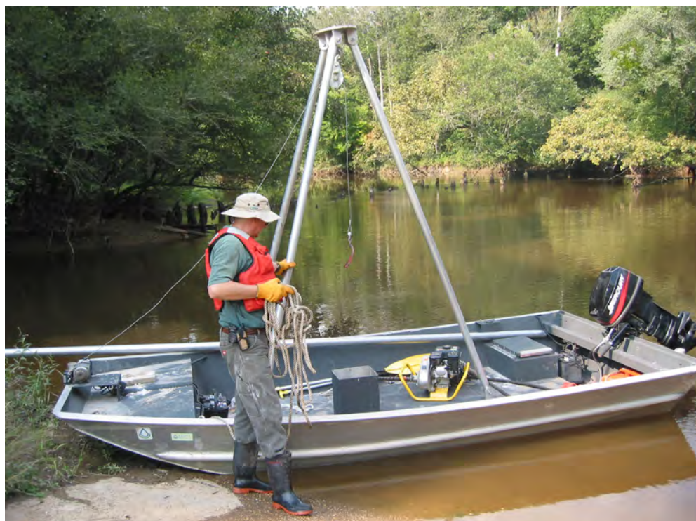
Figure 9. Vibracore system used to collect subsurface sediments. (Photograph by the U.S. Geological Survey, South Carolina Water Science Center, September 11, 2006.)
