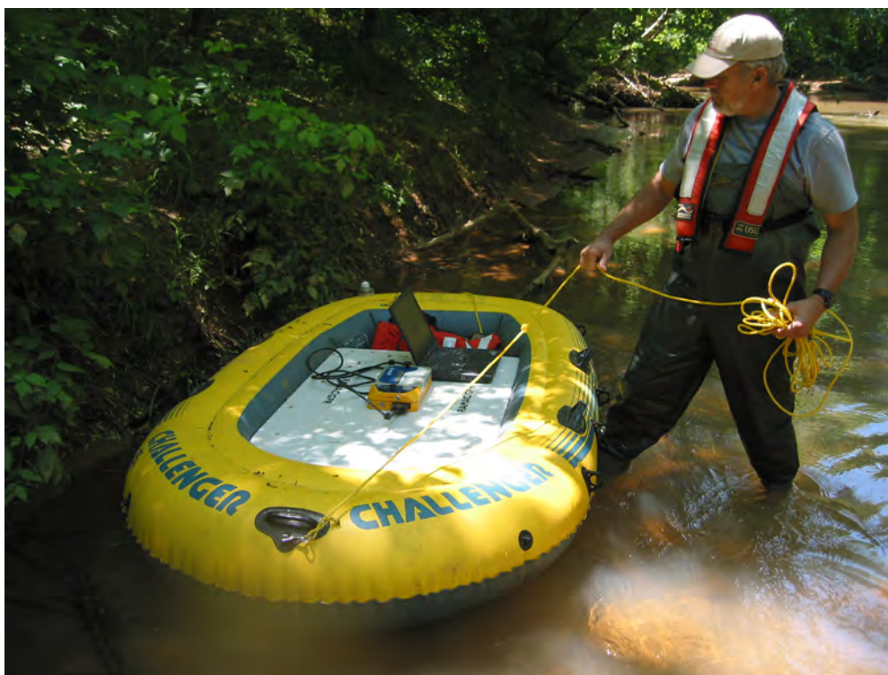
Figure 8. Collection of subsurface channel and scour data at structure 427006200500 on Road S-62, crossing the South Tyger River in Spartanburg County, South Carolina. (Photograph by the U.S. Geological Survey, South Carolina Water Science Center, May 26, 2005.)
