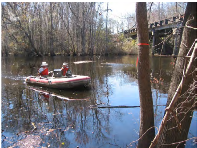
Figure 7. Collection of subsurface channel and scour data at structure 454004100500 on S.C. Route 41, crossing Black Mingo Creek in Williamsburg County, South Carolina. (Photograph by the U.S. Geological Survey, South Carolina Water Science Center, February 28, 2007.)
