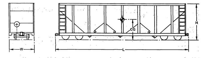
Length:Measured between pulling faces of couplers (in normal position)Width:Measured at eaves, tops of sides or platformHeight:Measured at eaves, tops of sides or platform
