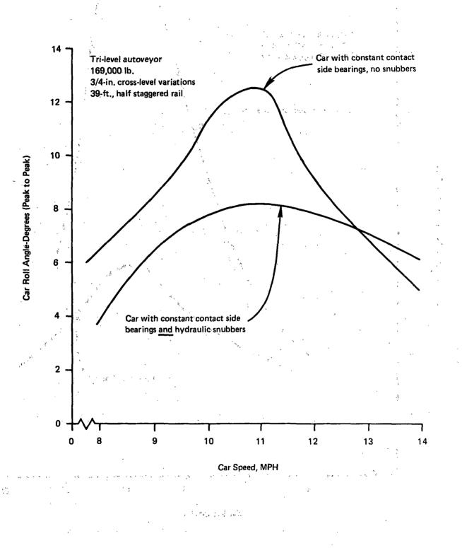
FIGURE F-2 EFFECT OF CONSTANT CONTACT SIDE BEARINGS AND HYDRAULIC SNUBBING ON MAXIMUM CAR ROLL ANGLE
