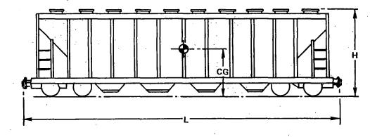
Length: Measured between pulling faces of couplers (in normal position)Width: Measured at eaves, tops of sides or platformHeight: Measured at eaves, tops of sides or platform
