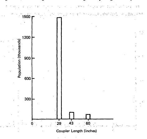
Source: DOT Transportation Systems Center Estimates Based on 1977 UMLER FIGURE 3-7 DISTRIBUTION BY COUPLER LENGTH, ALL CAR TYPES
