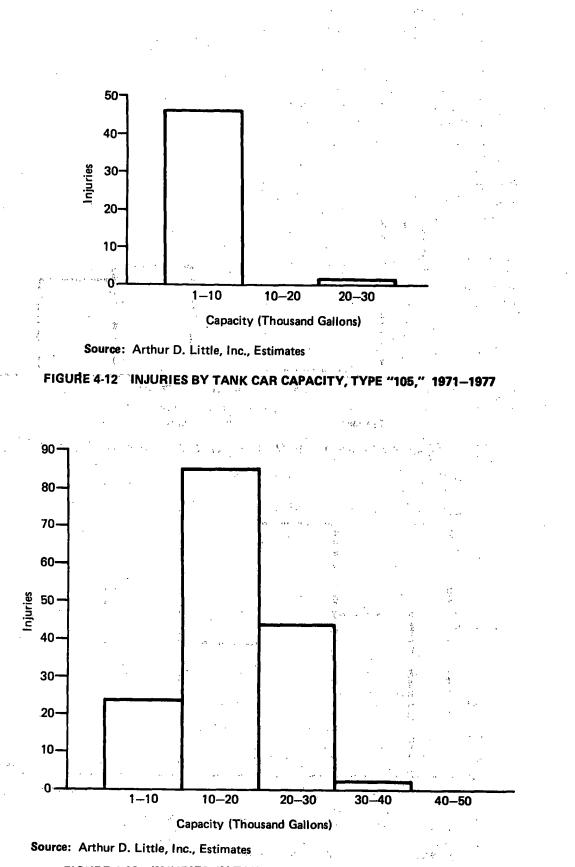
FIGURE 4-13 INJURIES BY TANK CAR CAPACITY, TYPE "111," 1971-1977
