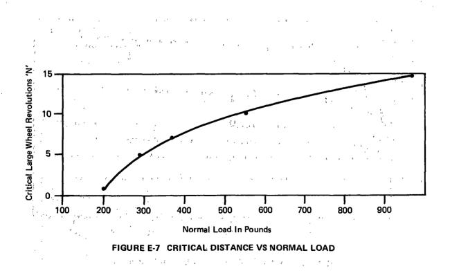
aspect needs further investigation and validation. The above data do not apply directly in a quantitative way to the plastic flow of rails in the field because the geometry and the side constraints of the total rail are not fully simulated; also non-linearity of material behavior is involved. However, it can still be used to gain a qualitative indication of the effects of higher tonnage cars.
