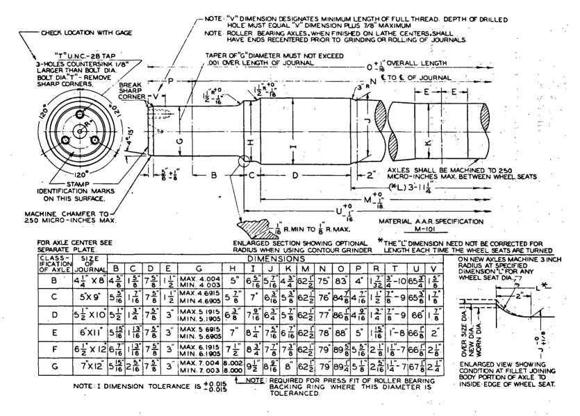
Source: Specifications for Design, Fabrication, and Construction of Freight Cars, AAR, October 1977
