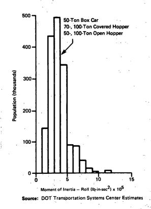
FIGURE 3-12 DISTRIBUTION BY ROLL MOMENT OF INERTIA, ALL CAR TYPES, UNLOADED
