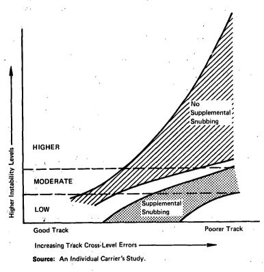
FIGURE 1-11 RANGE OF EXPERIMENTAL RESULTS FOR 100-TON OPEN HOPPER CAR
