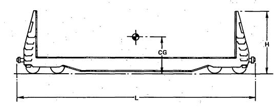
Length: Measured between pulling faces of couplers (in normal position)
