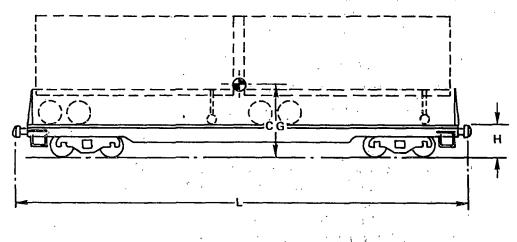
Length: Measured between pulling faces of couplers (in normal position)Width: Measured at eaves, tops of sides or platformHeight: Measured at eaves, tops of sides or platform
