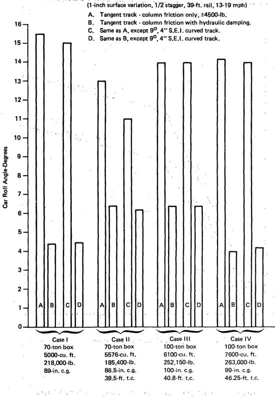
FIGURE F-5 EFFECT OF SNUBBING ON CAR BODY ROLL ANGLE ON TANGENT AND CURVED TRACK (1-inch surface variation, 1/2 stagger, 39-ft, rail, 13-19 mph)
