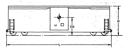
Length: Measured between pulling faces of couplers (in normal position)
