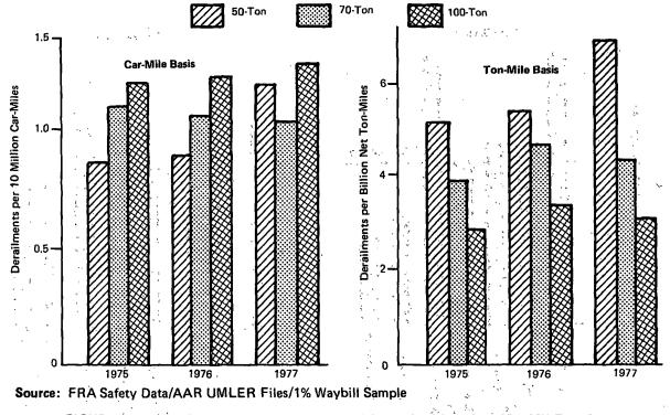
FIGURE 4-2 RELATIVE ACCIDENT HISTORY ON CAR-MILE AND TON-MILE BASIS (SPEED GREATER THAN 10 MPH)
