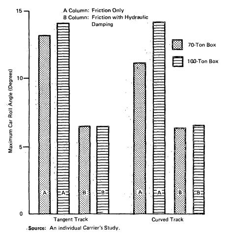
FIGURE 1-9 IMPROVEMENT FROM ADDITION OF HYDRAULIC DAMPING (1-Inch Surface Variations, ½ Stagger, 39-Ft. Rail, 13–19 MPH)
