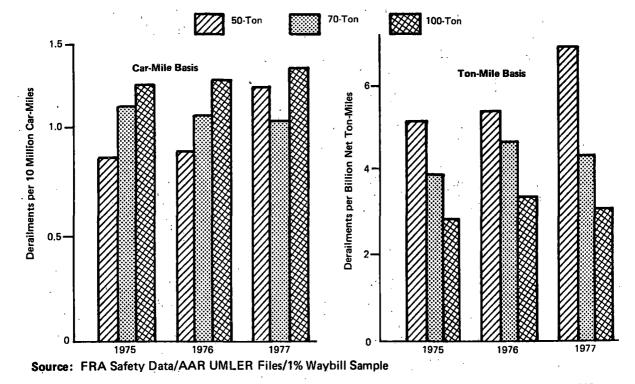
FIGURE 1-6 RELATIVE ACCIDENT HISTORY ON CAR-MILE AND TON-MILE BASIS (Speed Greater Than 10 MPH)
