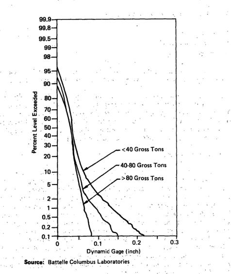
FIGURE 5-1 EFFECTS OF CAR GROSS WEIGHT (AXLE LOAD), ALL SPEEDS, RAIL TEMPERATURE <80°F
