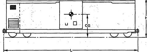
Length: Measured between pulling faces of couplers (in normal position)
