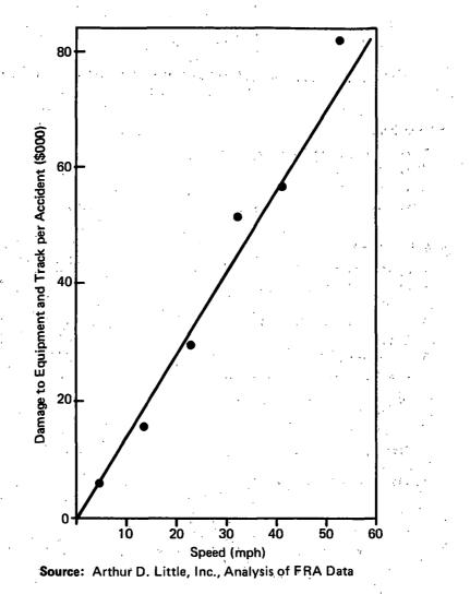
FIGURE 5-5 RELATIONSHIP BETWEEN ACCIDENT SPEED AND EQUIPMENT AND TRACK DAMAGE
