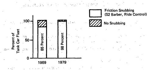
(b) Implementation Record: Improved Snubbing on Tank Cars (based on a survey of approximately 75% of the tank car fleet)
