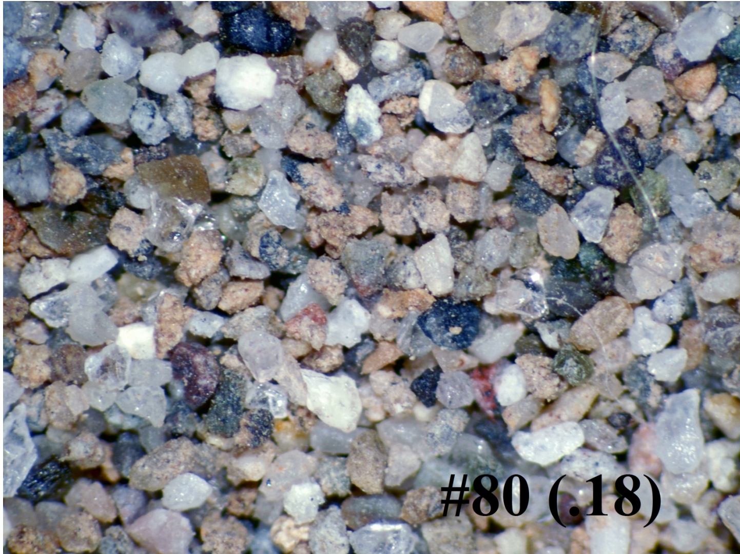
Figure B.5. Close-up of 0.0071 in. (0.18 mm) soil particles used in 2013 and 2014 K_{sat} testing.
