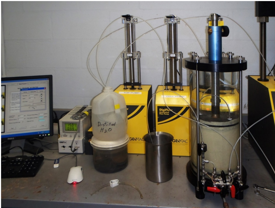
Figure 10. Flexible wall permeameter testing system.
