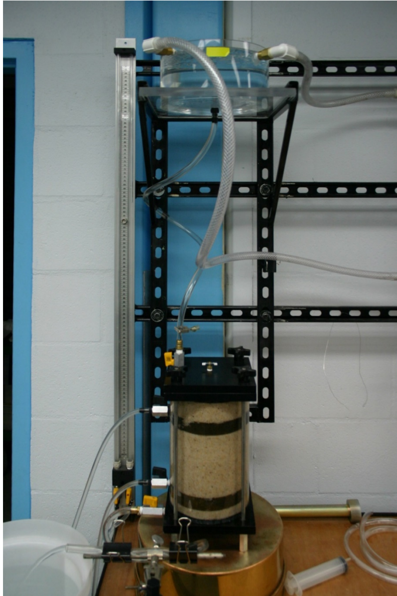
Figure 8. Test equipment setup for rigid wall permeameter testing.
