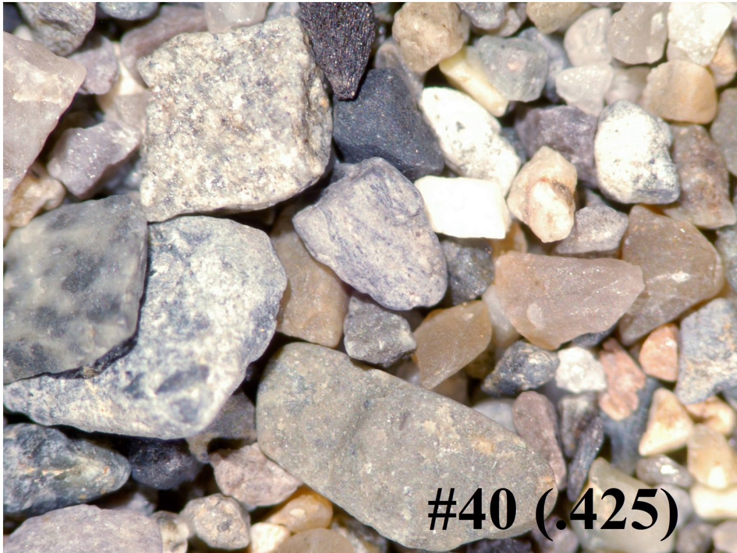
Figure B.3. Close-up of 0.0167 in. (0.425 mm) soil particles used in 2013 and 2014 K_{sat} testing.
