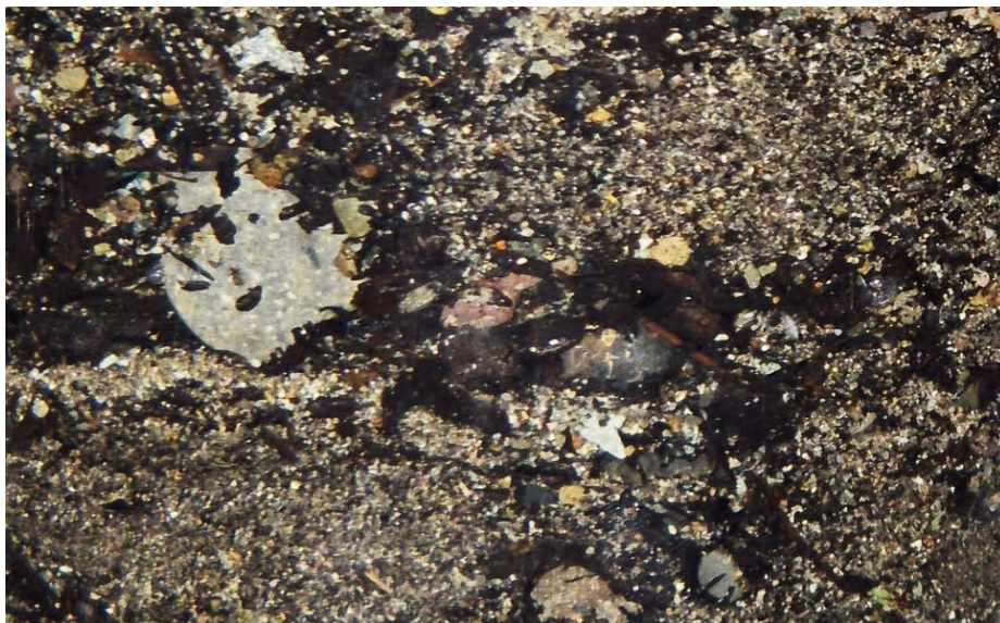
Figure 4. Close-up of soil as placed in the rigid wall test cell for soil used in the 2008 testing.
