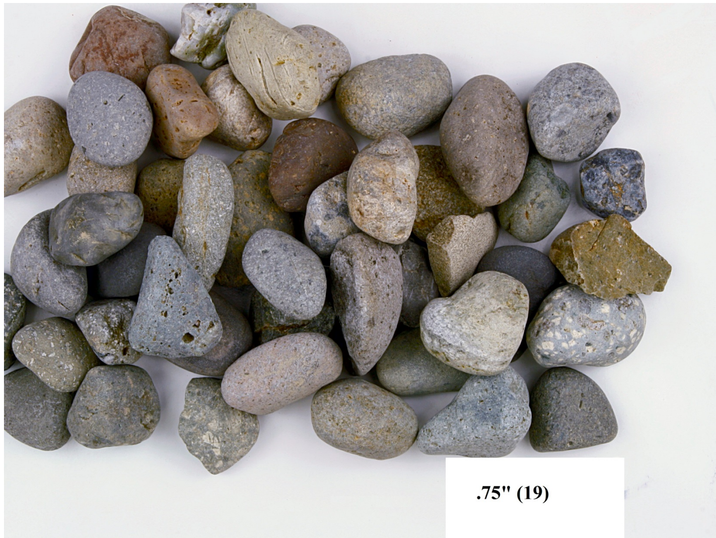
Figure B.2. Close-up of 0.75 in. (19 mm) soil particles used in 2013 and 2014 K_{sat} testing.
