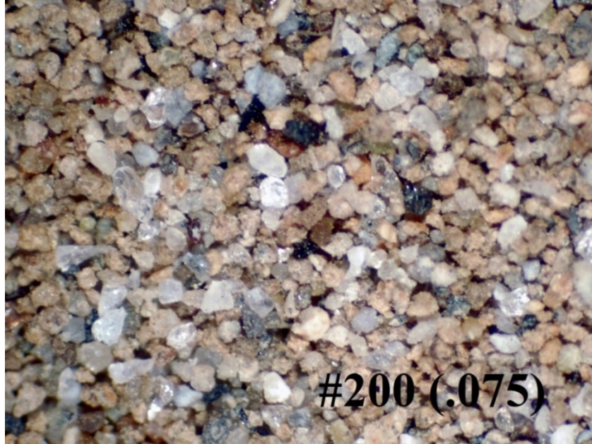
Figure 7. Close-up of test soil grains used for 2013-2014 testing – 0.003 inch (0.075 mm) size.
