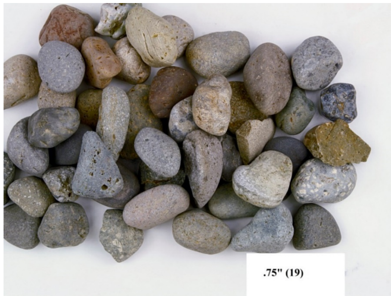
Figure 5. Close-up of test soil grains used for 2013-2014 testing – 0.75 inch (19 mm) size.
