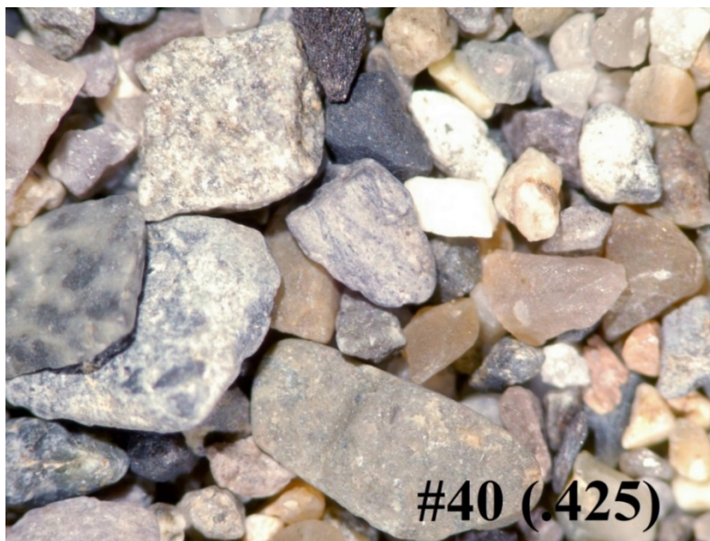
Figure 6. Close-up of test soil grains used for 2013-2014 testing – 0.017 inch (0.425 mm) size.
