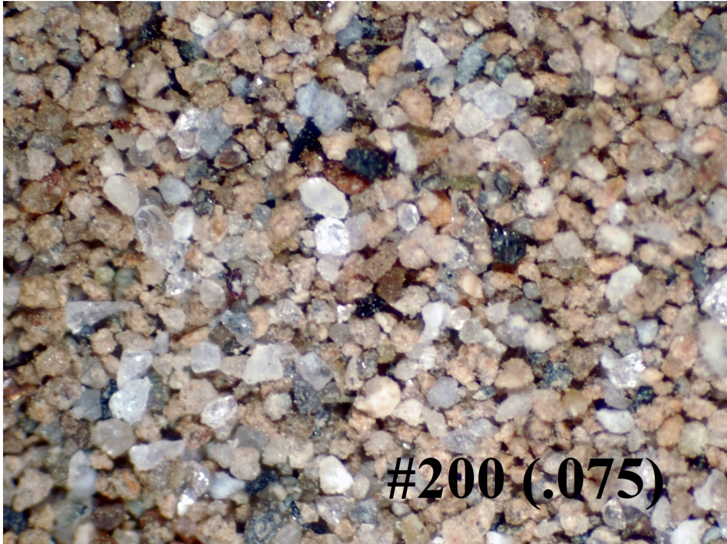
Figure B.7. Close-up of 0.003 in. (0.075 mm) soil particles used in 2013 and 2014 K_{sat} testing.
