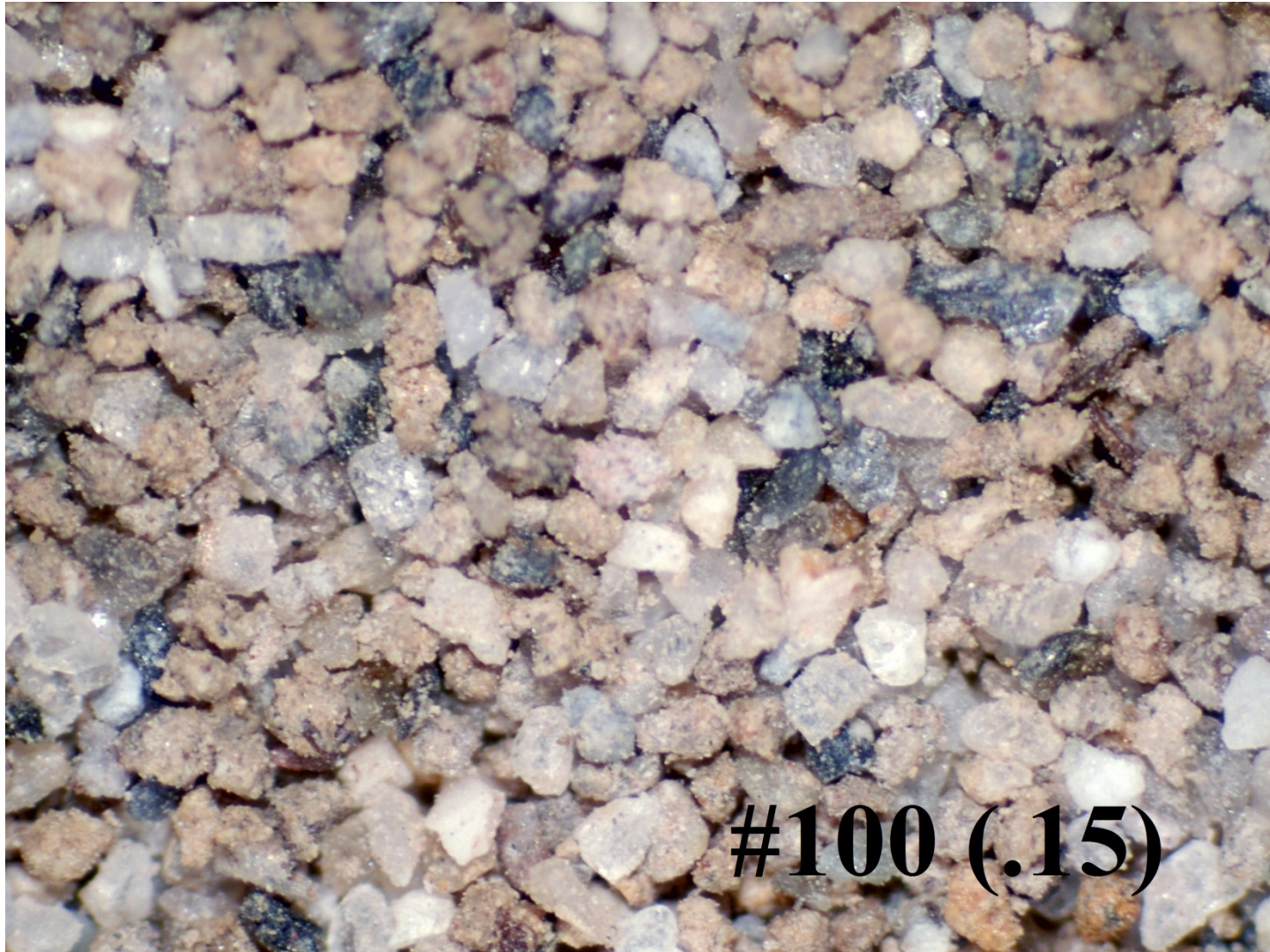
Figure B.6. Close-up of 0.0059 in. (0.15 mm) soil particles used in 2013 and 2014 K_{sat} testing.
