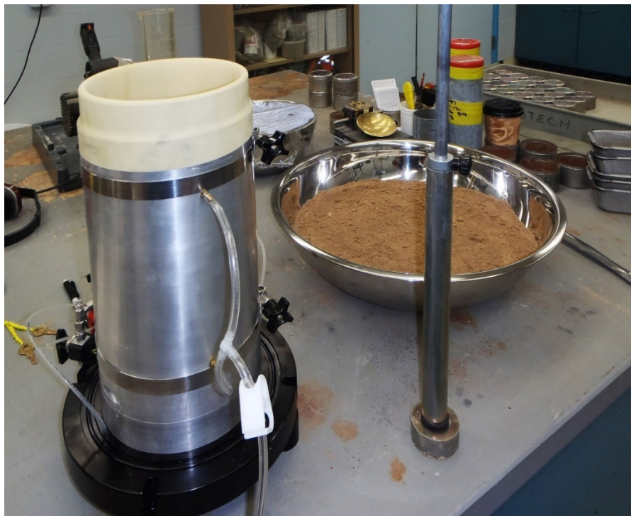
Figure 12. Specimen mold with rammer and test soil.
