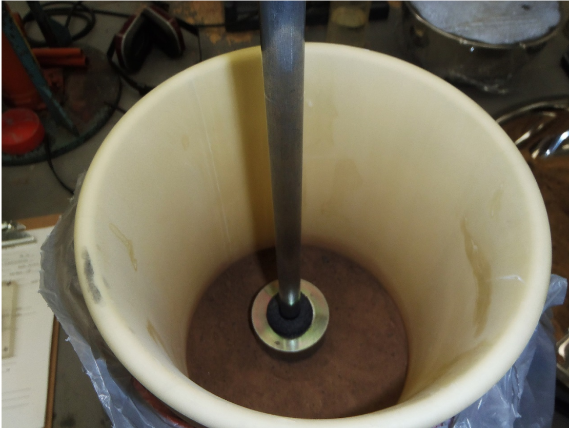
Figure 13. Test specimen being compacted with rammer.
